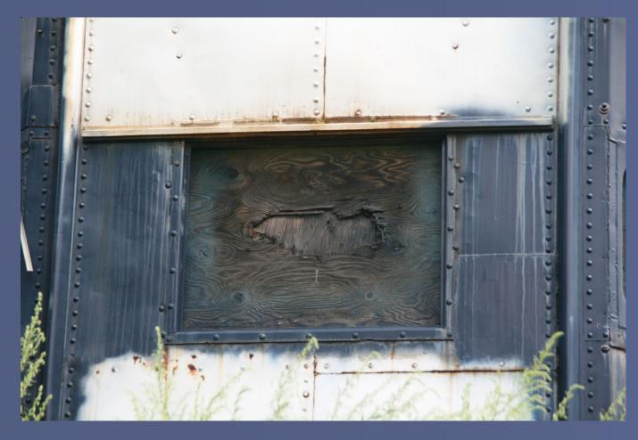
Figure 24: Plywood is often used to cover the windows of equipment that is in long-term storage. This removes a tempting target from vandals. The plywood covering the bay window of this caboose prevents weather from reaching the interior, causing further damage.
