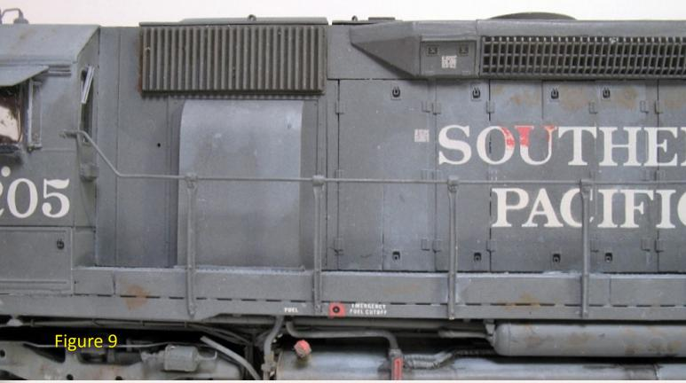
Figure 8 and 9: Elizabeth salvaged a portion of a damaged walkway from her parts stash to lengthen the duct for the traction motor blower, and to replace the top half of the blower cover. The grille was salvaged from an Athearn SD45T-2. The fairings on the dynamic brake bulge and radiator were built-up from strips of styrene.
