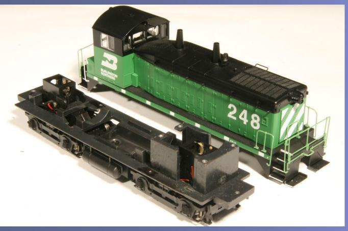
Figure 17: With the locomotive's drivetrain fully removed, we now have an unpowered chassis that the shell can be mounted onto.
