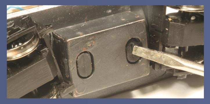
Figure 16: Removing the motor from a model locomotive requires removing any screws holding it in place, then pressing the motor mounts from the frame with a screwdriver.
