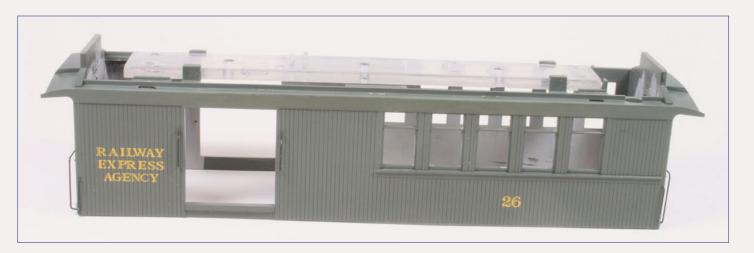
Figure 9: The light bar attaches across the top of the body shell and is held in place with plastic ears. Filing the tabs lower on the ears makes disassembly of the parts easier for repair. Grabirons and handrails have been applied to the body shell.
