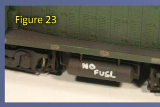
Figure 23: One marking that can be found on stored, sold, or donated locomotives is 'NO FUEL' indicating the tanks are empty and should remain that way.
