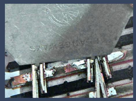
Figure 43: I test fit the guard rail and determine its position using the flangeways side of an NMRA gauge. Then I tack it in
