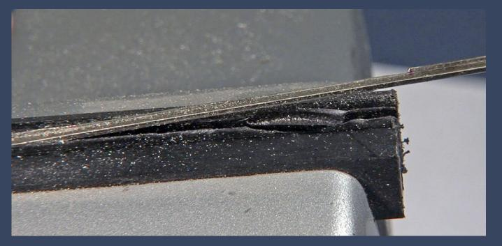
Figure 19: Here's the completed stock rail with a taper filed in the base. Notice I touched only the base of the rail – I did not touch the railhead with the file.
