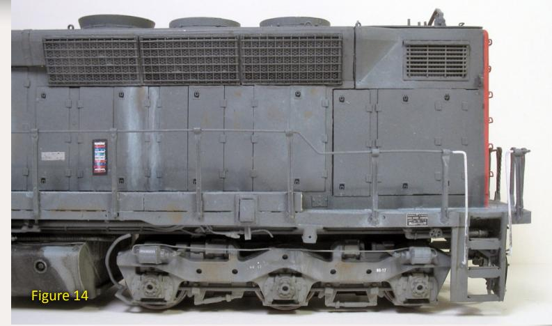
Figure 13 and 14: Elizabeth scratchbuilt the hood of her SDP45 using Evergreen styrene and Cannon doors. Other details include radiator grilles salvaged from a Proto 2000 SD45, and Precision Investment Associates (PIA) handrail stanchions (Figures 2, 8, 13, and 15).
