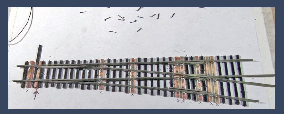
Figure 52: At this point turnout construction is basically finished, so I remove all the spikes from the PC ties. I leave the spikes holding the plastic ties since they need to remain in place until I'm ready to glue the turnout rails to them.
