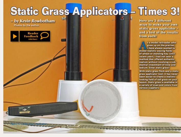
Figure 1: Kevin's original article in the Mar/Apr 2010 issue of MRH demonstrated step-by-step 3 different ways to build your own static grass applicator. One of the best ways was using the 12V negative ion generator from Oatley Electronics. Unfortunately, Oatley has discontinued the generator shown in the article, so here author Kevin Rowbotham gives updates on how to use the new improved 12V negative ion generator from Oatley.
