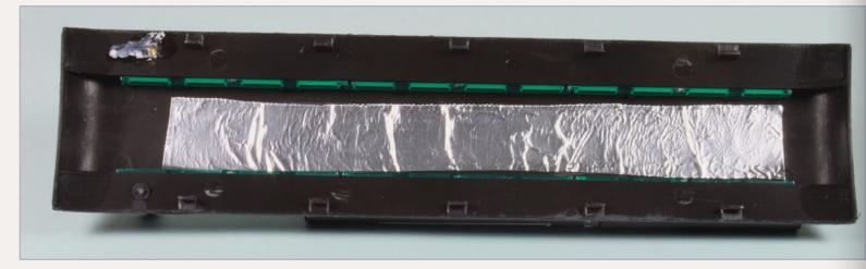
Figure 13: A roof reflector helps even-out the illumination. Apply a piece of double sticky tape to aluminum foil, trim with a scissors and attach the foil inside the roof.
