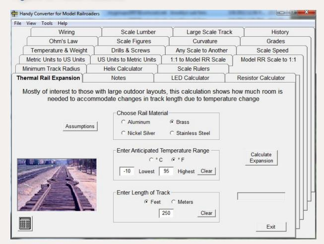
Figure 4: Thermal Rail Expansion.
