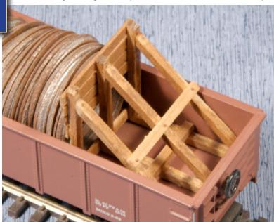
Assembled Bulkhead in gondola with load of ring castings.
