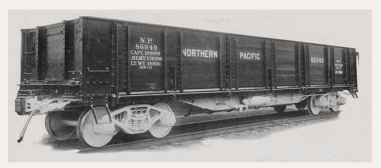
Figure 2: Builders photo of a Hart convertible car built for the Northern Pacific by the Roger Ballast Car Company in 1927. – Richard Bale collection.
