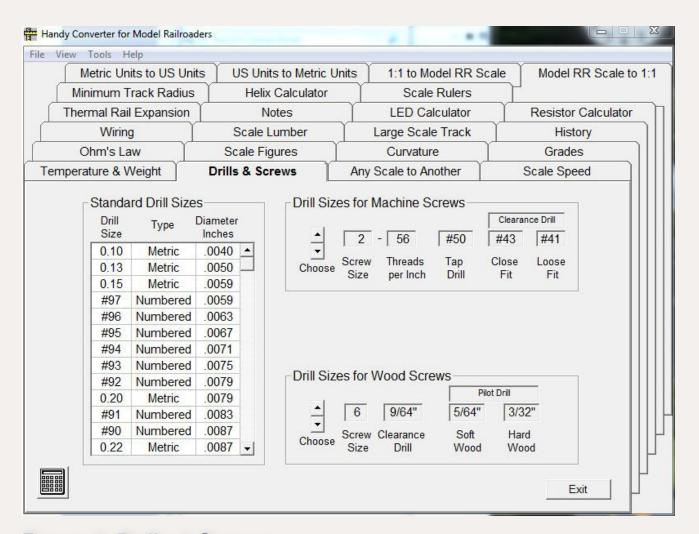
Figure 7: Drills & Screws.
