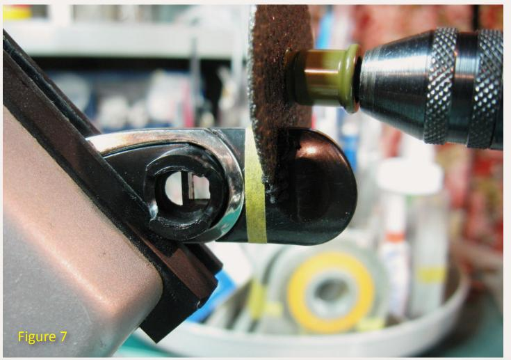
I made my cut a little bit away from the line and cleaned up the remainder with a disk sander (Figure 08). While I was there, I opted to give the bottom of the clip a pass on the sander as well to even things out.
