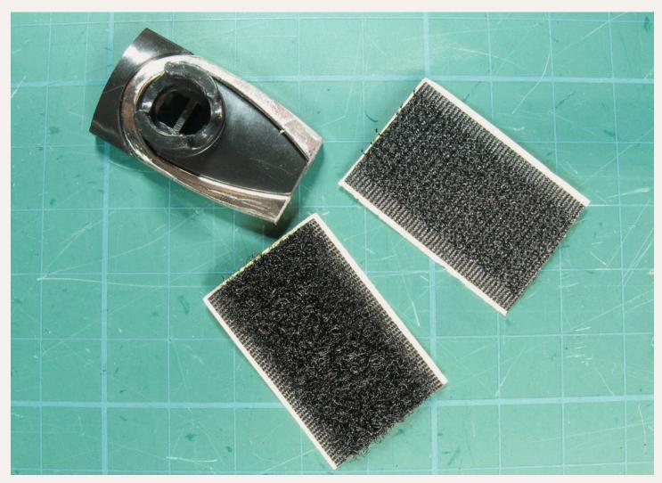
Figure 9: Cut two pieces of Velcro and add to the Optivisor and the other to the bottom of the modified clip.
