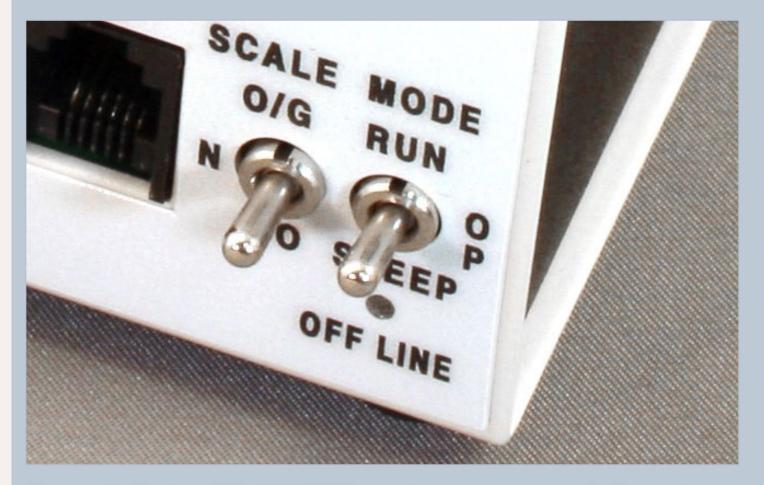
Figure 15: Digitrax DB150 MODE switch used to change OpSw settings – typical of all Digitrax system boxes.
