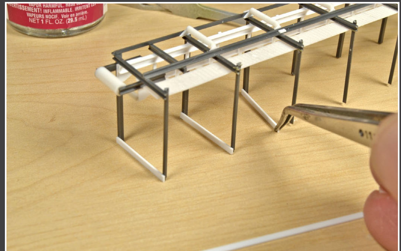
18: Connecting the Conveyor Roof Supports..
