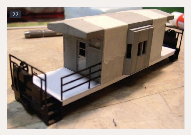
27: One handrail in position, and three to go. Don't glue the handrail. The masking tape holds the body in place temporarily.
