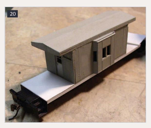
20: When the deck is secure, glue the .030" x .100" sill strip to the side.
