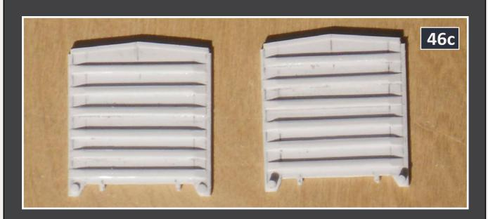
46c: Now for the tabs that the grab Irons mount to. I cut four pieces of 4" x 6" stock and cemented them to the bottom of the ends. The inside edges are 2'-6" from the edge of the car. Once these had completely dried, I filed a small taper on the inside edge of each one. That completed the major construction of the ends.
