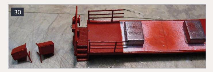
30: Place the former battery boxes next. They represent tool boxes now. Drill pilot holes to mount the boxes. I add support bars to the ends of the boxes when I glue them in.
