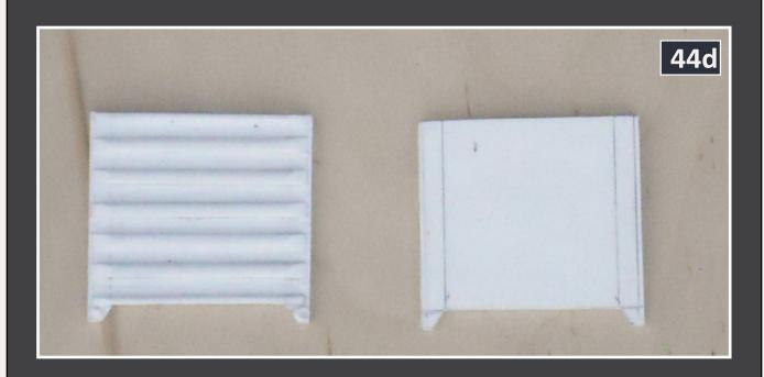
44d: I took a little extra time and care to make sure that the center rib was square with the body. All of the other ribs will be built off of this one. After studying the photos, I came up with a spacing of 9" between the ribs because it gave me the closest appearance to that in the photograph of 75893. Once all of the ribs had been placed on both sets of ends, I filed down the 4" x 4" to the height of the ribs on the car.
