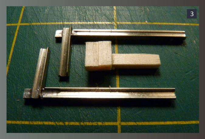
3: These are the three sub-assemblies required to make the bumper.
