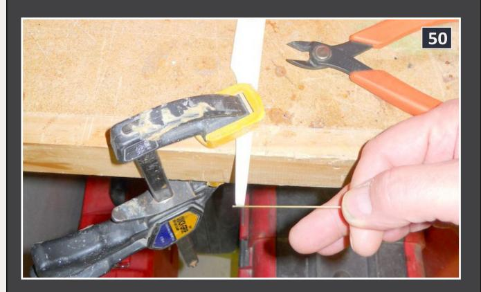
50: I have a homemade jig that I use for bending wire for grab irons. The jig is made of two pieces of .060" plain styrene were cut to 5-1/2" long by 3/4" wide. At one end I made a taper from 3/16" (HO scale 16") to 1/2" (HO scale 3'-10"), and this taper is 3" long. A hole was drilled so I could hang it on a peg at my workbench. A piece of .020" freight car siding was cemented to one side of the jig. I then filed the pieces to create a nice smooth surface along the sides.
