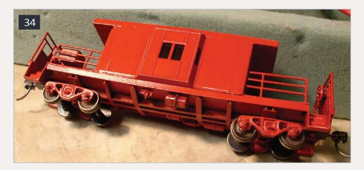
34: Details make the difference in any project. Here a brake valve and an extra air tank are attached. Kadee #5 couplers have also been installed and the finished trucks are mounted to the chassis. It is starting to look like a caboose!
