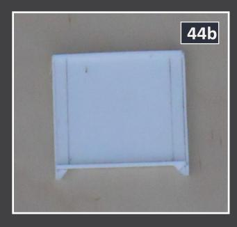
44b: I began by measuring up 10" from what would become the bottom, and drew a line. Next I measured in 8" from each side and made a mark at the bottom. This was followed with a measurement of 1'-2" in from each side and
