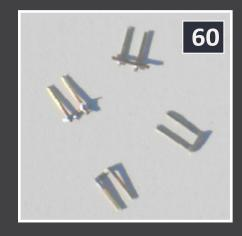
fly away into the vortex of the workshop floor. Little parts like these are hard to find unless they are spotted immediately. After the parts were trimmed I bent the top end approximately 45° angle.
