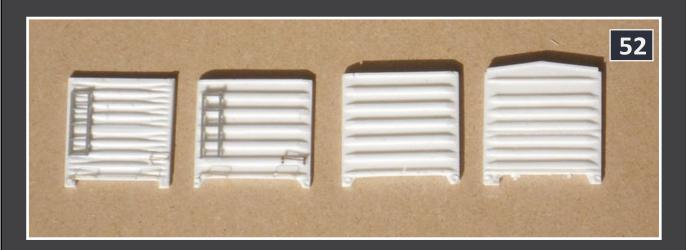
52: One of each of the ends in the process of being detailed.
