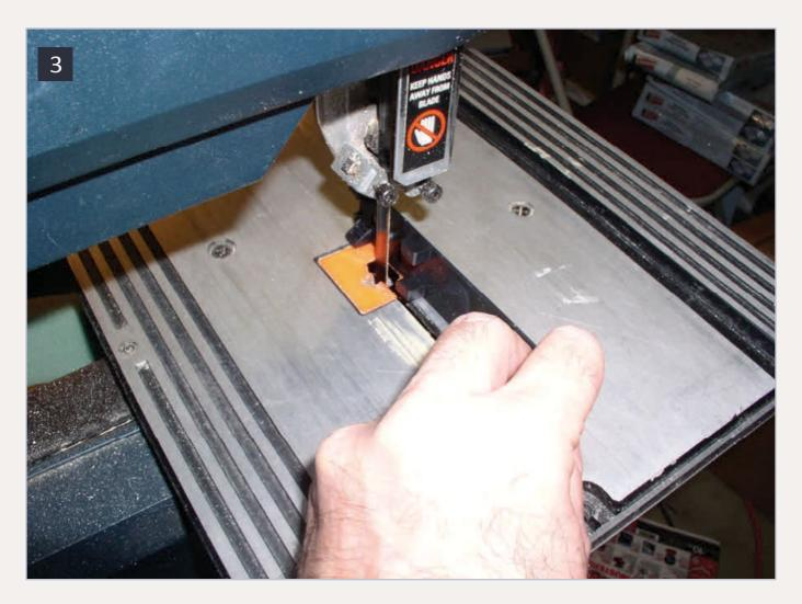
3: I use a 10-inch band saw to remove the battery boxes. Do not discard them, as they will be used in the superstructure build.
