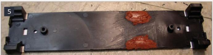
4-5: Add a thin piece of .010" or .020" styrene to the top of the underframe. Cut it to the width of the underbody, and short enough to expose the walkway grid on the ends. Fill the battery box holes on the underside with putty. After the putty cures, sand it flat and smooth. While I wait for the putty to cure, I can cut up the main bay window caboose body, exactly what the MP shops did in DeSoto, Missouri in the 1970s.
