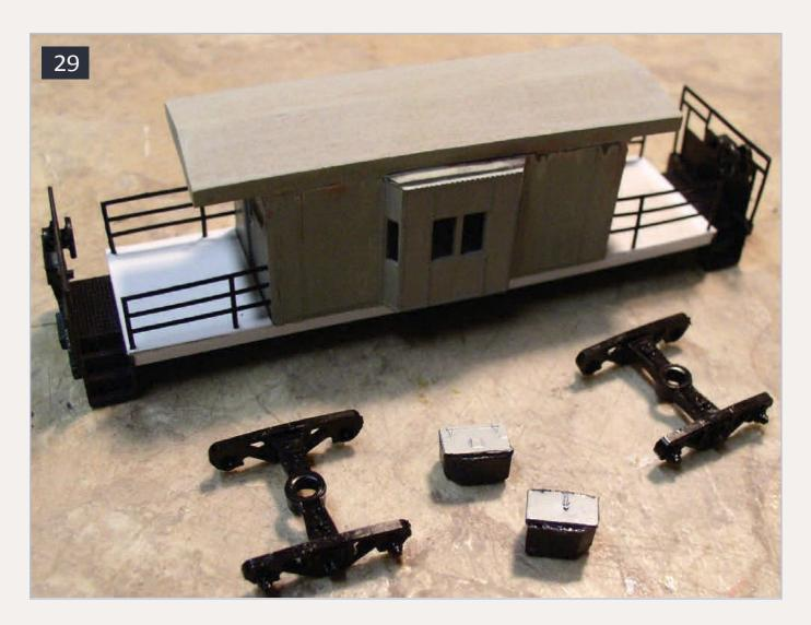
29: We are ready for paint. Everything in the picture will be painted Floquil Caboose Red. The battery boxes are made into tool boxes. Be sure to clean the truck bearings with the truck tool after painting to ensure free-rolling wheel sets. I use JayBee 33" wheels.
