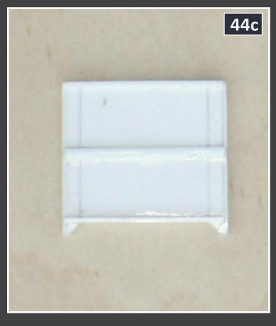
44c: Next the 75500-75999 and the 76000-76499 cars have a small rib at the top and bottom of the ends. I simulated these with 4" x 4" stock. I did not bother to round these over yet or reduce the thickness to 3". That will be done later. After the top and bottom rib were located, I identified
