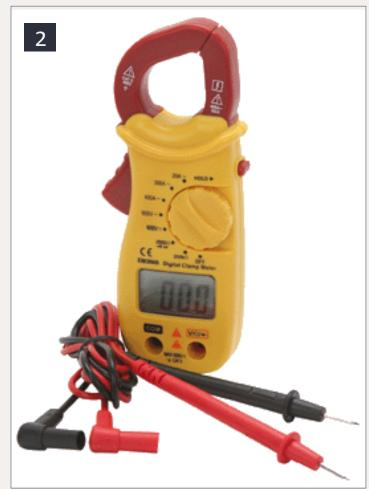
2: A typical inexpensive clamp-on ammeter. This one is available from Harbor Freight. We will use a meter similar to this to see if we can detect the DCC current flowing in our layout wiring.
