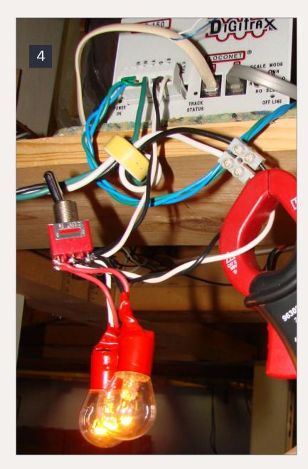
4: Current limited by lamps being measured at booster.
