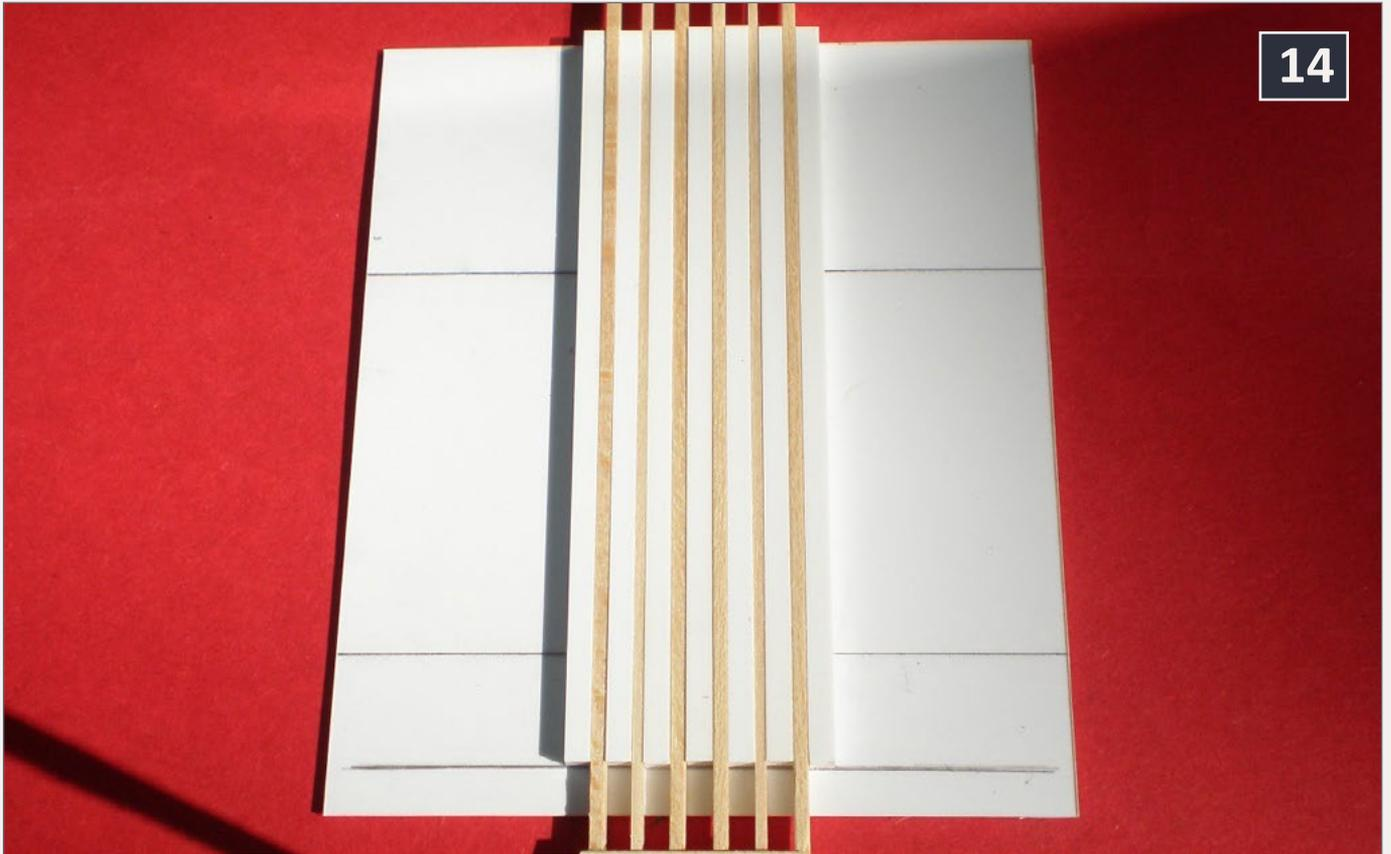
**14: Underframe and jig for the Tweetsie boxcars. This can be used for both the 32' and 36' cars. It can also be used for other railroads' cars.**
