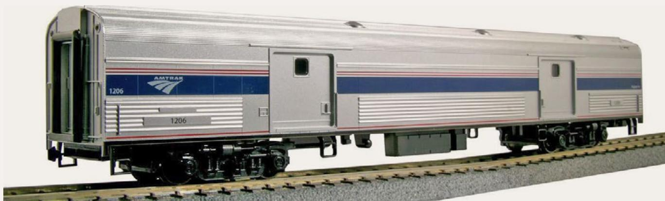
Kato USA ([katousa.com](http://katousa.com)) has added a baggage car to its lineup of Amtrak Superliner models. Features of the HO scale ready-to-run model include prototypical exterior fluting and appropriate trucks with working bearing caps and shock absorber. Optional Kinematic tight-lock couplers are included. The late additions to the Superliner group will be available in two road numbers in Amtrak's phase IVb scheme. The final MSRP is estimated at \$85.00 to \$90.00 each.
