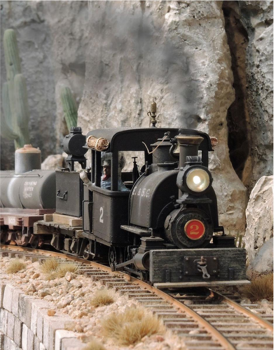
6. The drawbar on the pilot of #2 has a brass link-and-pin drawhead I designed with friend Bill Hay. link-and-pin drawheads were standard equipment on all E&SG locomotives.
