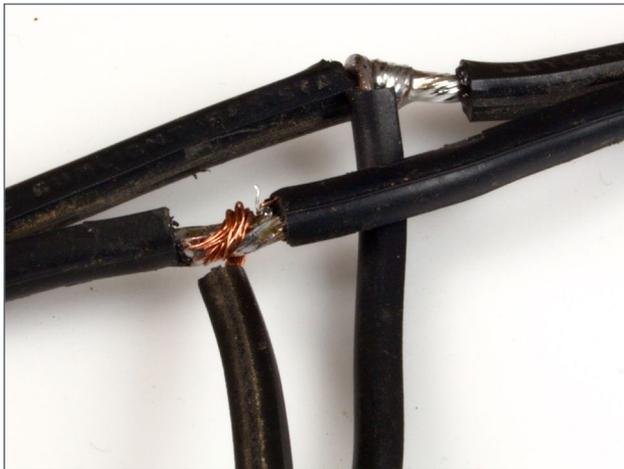
12. Connection between drop wires and bus wire. Two joints are shown in the photo. In the upper right is a completely soldered one – note the bright and smooth surface, indicating that enough heat has
