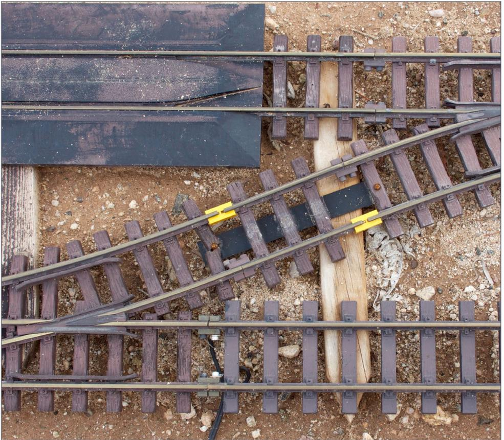
7. Rail gaps on the RMP before painting the yellow joiners. Note: black plastic strip screwed to ties to hold gaps together. Note, also: black feed wires connected to Split Jaw clamp with stainless steel socket head screws.
