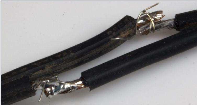
**14. Butt splice in bus wire. Lower left has been wrapped with smaller solid wire and soldered. The**
