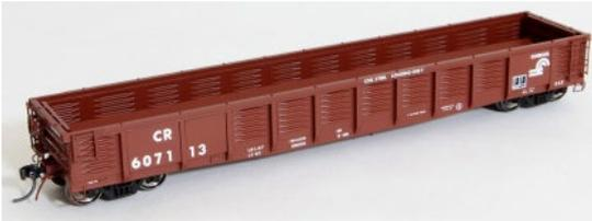
This Conrail version represents the G43 gondolas CR modified with special racks to transport uncovered steel coils. A set of eight steel coils painted in
