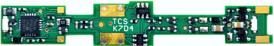
**Train Control Systems** is selling a drop-in decoder for Kato's ACS-64 electric locomotive and Electro-Motive Division SDP40F units. Identified as TCS item K7D4, the decoder includes built-in forward and reverse light-emitting diodes, two solder pads for additional lights, auto-adjusting back-electromotive-force control, and Quiet Drive. For additional information visit [tcsdcc.com](http://tcsdcc.com).
