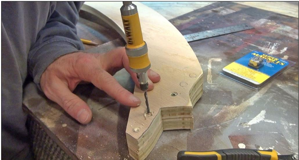
18. I drilled holes through the lift-out ends and the plywood that was cut to match the ends and would act as a base in the foam. These holes ensured that the magnets would match up.
