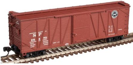
quarter of 2016. Depending on the prototype being followed, the N scale models will have either Murphy 7-8 or 5-5-5 (above) corrugated steel ends and simulated steel or wood
