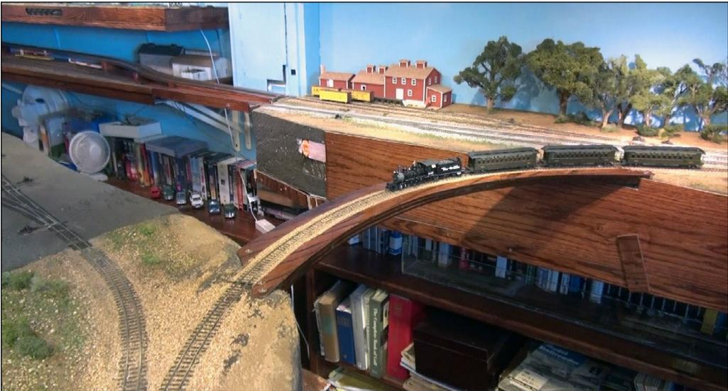
29. After testing the contacts for power conductivity I ballasted the track and finished the scenery for the approach areas to the lift-out section. I then test ran the first train across it.
