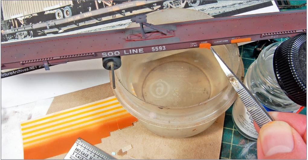
32. Now apply freshly painted patches on the 5593 and on the 5593. On the 5593, I decided that Reefer Orange will best capture this look. Use an airbrush to paint a scrap of Champ decal material. Use a #11 X-Acto blade to cut out the right size patches and apply these as a decal.
