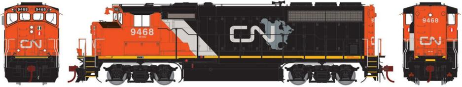
Athearn has scheduled a February release for a Genesis Series Canadian National GP40-2L diesel repainted in CN's modern liveries including the short-lived North American map scheme shown here. Spotting features include a late CN body with a comfort cab, snow shields, CN-style pilot plow, ribbed anti-climber, and Blomberg-M trucks.
