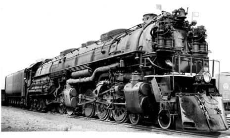
Notable features include cast pilot with a fold-down coupler, an enclosed cab with side entry doors, a simulated cab diaphragm, twin air pumps mounted on the front of the smokebox, unique four-wheel trailing truck with
