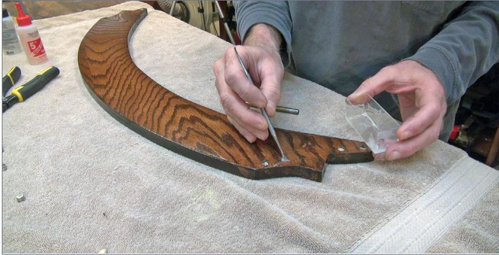
21. After staining the wood and applying polyurethane, I mixed 5-minute epoxy and placed this in the holes where the magnets would be glued flush in the wood.
