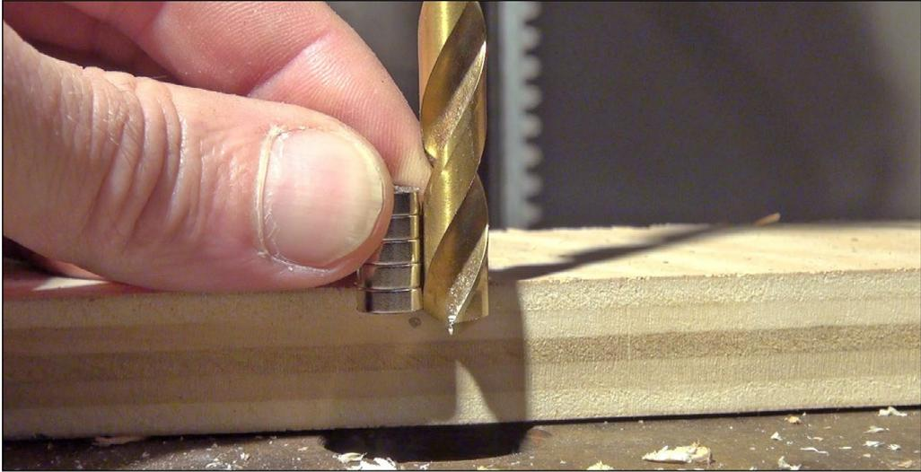
19. I set the depth of the feed on the drill press to match the magnets and drilled 16 identical holes in the plywood to accept the magnets.
