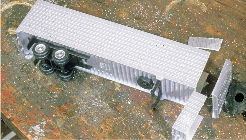
4. After removing this section, sand the edges for a square joint before using liquid cement to re-attach the body pieces.
