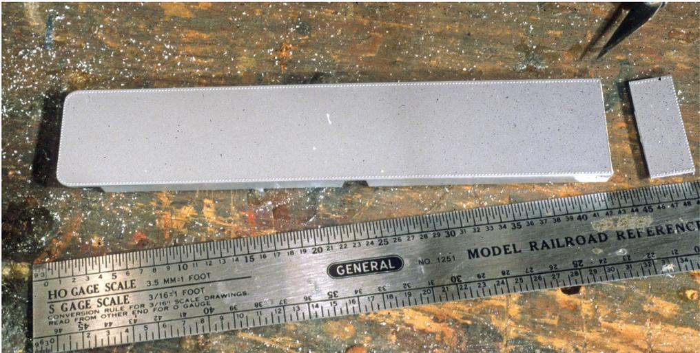
5. Next, remove the same amount of material from the rear of the roof piece.
