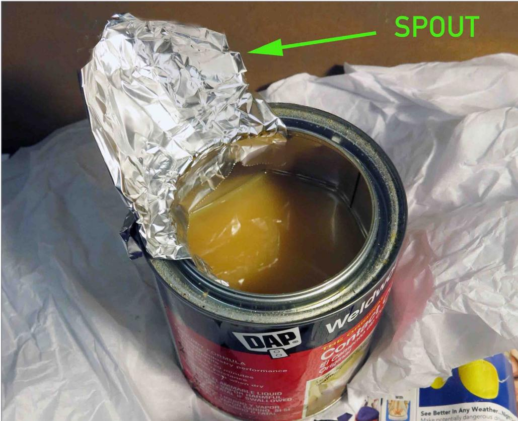
5. A home-made spout makes it easy to decant contact or rubber cement into a small container from a large can.
