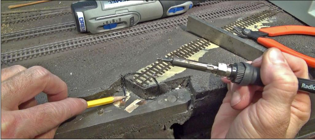
28. I also placed contacts in the base plywood in the end that adjoins my around-the-room home layout. These contacts were soldered to wires that pick up current from the rails.
