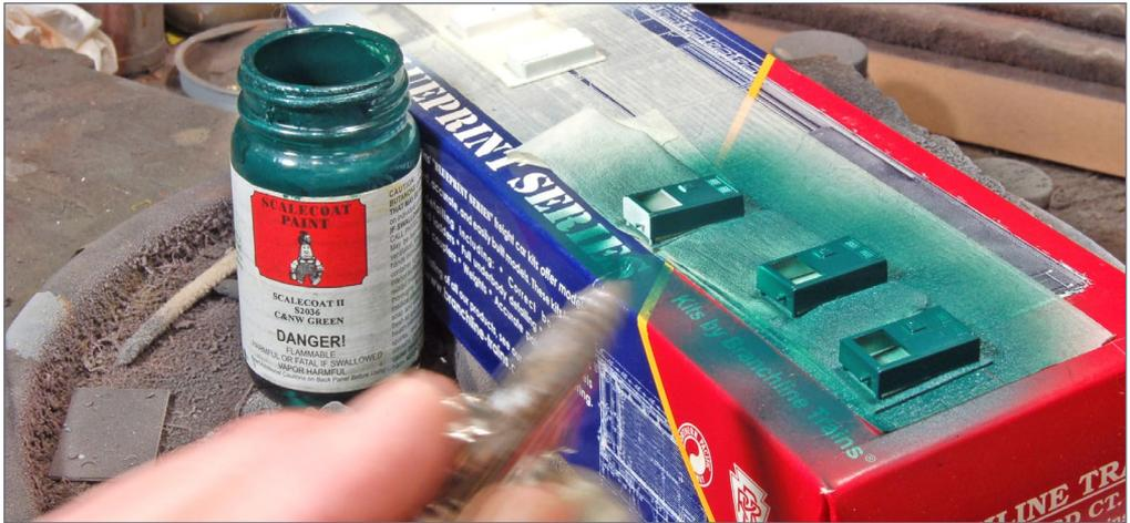
8. I use my airbrush to apply the paint to the refrigeration units.
