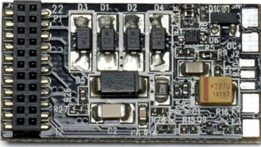
back-electromotive-force (BEMF) control with silent motor running, 28-step adjustable speed table that supports long addresses, advanced consist address setting, and an adjustable braking function. The
