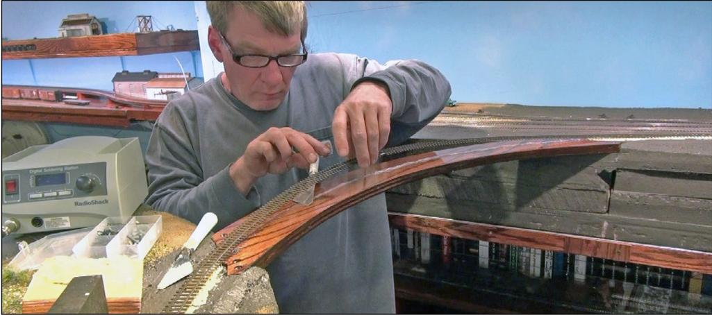
25. I glued Code 70 Micro Engineering track to the foam with Liquid Nails. I attached the track to the plywood lift-out with clear silicone caulk, using a painter's knife to spread the glues. The fact that Micro Engineering flex holds its shape after being curved made it easy to match the ends to where it would join my main lines on both layout approaches.
