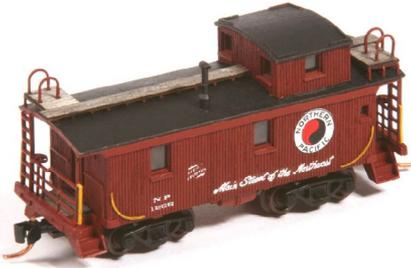
**American Model Builders** has introduced a laser-cut body kit for an N scale Northern Pacific 1200 series wood caboose. The kit features laser-cut underframe and end platform and laser-cut body components using custom
