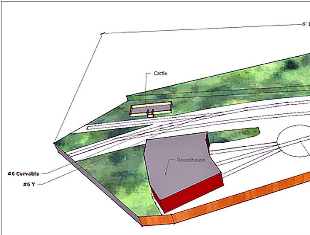
6. Pembroke TOMA - Phase 1 is a seven-foot corner module incorporating a turntable, passing siding and two spurs.
