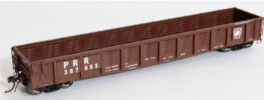
The newest HO scale freight car from **Tangent Scale Models** is an all-new Pennsylvania/Penn Central class G43 100-ton 52-foot 6-inch corrugated side gondola.
