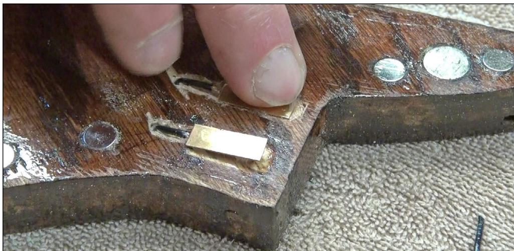
27. A piece of 1/32 x 1/4-inch brass stock cut one inch long forms the power contacts to feed current to the rails in the lift-out section. These contacts were placed in a carved-out space to fit almost flush. I soldered wires to the contacts, then fed the wires through the plywood to the rails.
