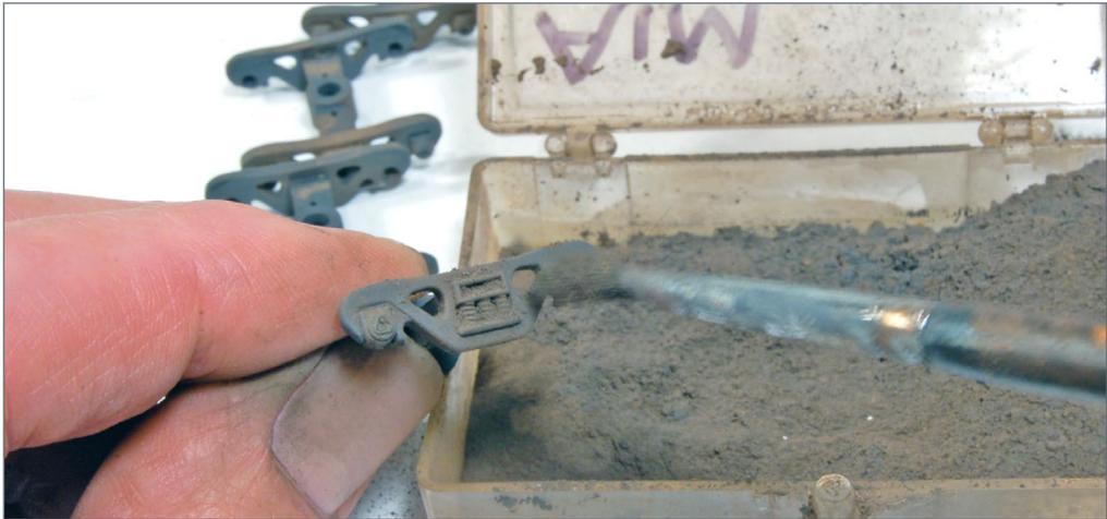
35. Next, apply weathering powders to the side frames and brush powders onto the wheels. The flat Grimy Black paint provides a great surface for the AIM weathering powders to bite into.
