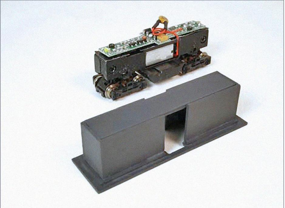
2. A simple shell of .040" and .060" styrene slips snugly over the top of a Bachmann 44-tonner mechanism, providing a sturdy structure for the couplers and the fragile stained stripwood wrap. The gap in the middle allows for airflow to prevent overheating. The styrene shell is spray-painted dark gray so it disappears behind the doors and windows of the outer structure.
