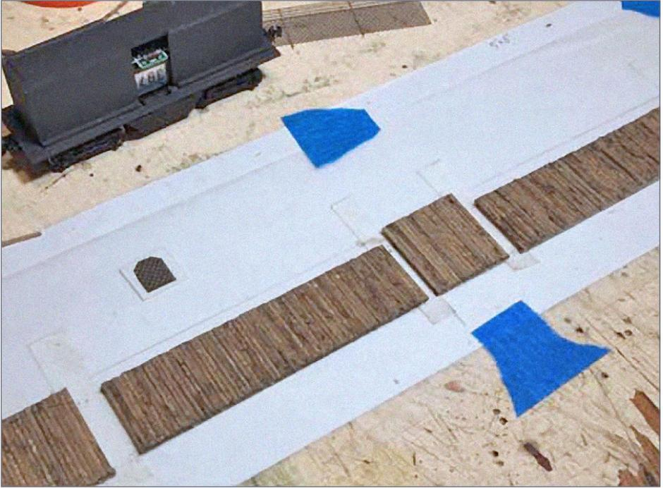
3. Once the styrene frame is finished and MTL Z-scale couplers are installed, draw a template for the sides and ends. Use prototype photos for reference and, while you don't need exact scale measurements, try to keep realistic ratios between doors, windows, and wall heights and widths.
