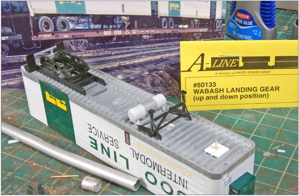
9. Next come the underframe details. I use A-Line #50133 for the landing gear. The A-Line Thermo King units are supplied with fuel tanks that are too small for this project. I extend the tanks to more appropriately reflect the prototype tanks. To do this, I use a piece of 2'-6" inch long aluminum tube cut to length using a razor saw. Glue this between the two A-line parts.
