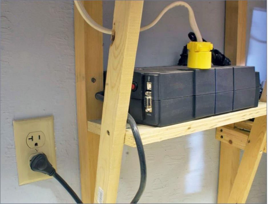
**3. UPS on the PCMR layout. Plugged into the wall and feeding the layout switch [2] through the Romex and (yellow) plug.**
