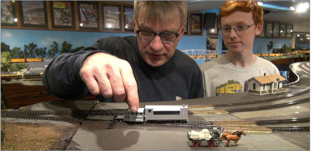
4. I was trying to run my HO<sub>N3</sub> Galloping Goose rail bus on my newly laid track near the log mill and it kept stalling on switch points – which I just cleaned last week. Due to the light weight of the model it stalls easily on dirty track. Daniel Coombs pointed out that Digitrax makes a Power Xtender that allows the model to run many feet without track power. That sounded like just the project I wanted to jump into.
