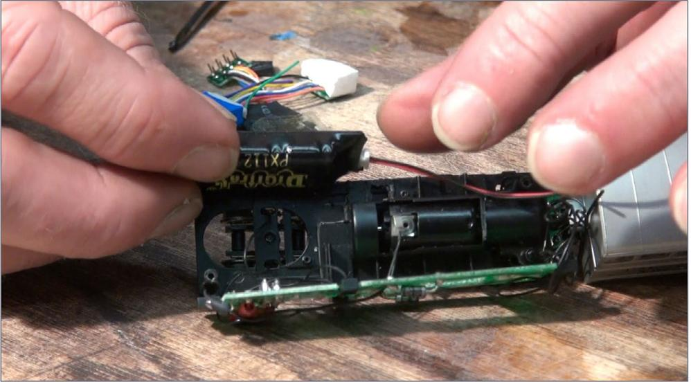
5. We pulled the model apart to see the space we had to work with. After cutting out five seats in the model, there was enough space to fit the Power Xtender under the circuit board.
