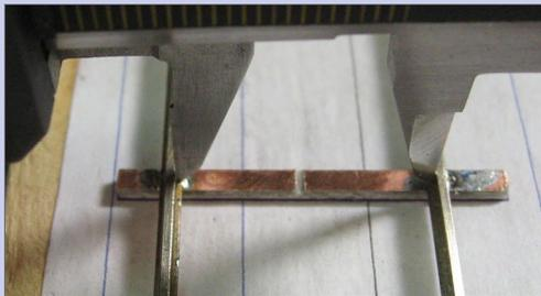
gauge to double check track spacing before and after soldering. Note that the track gauges are only useful until the stock rails begin to diverge. After that, you will need to rely on your printed plan for placing the curved stock rail. This is okay, because we will use the track gauge later to make sure everything is correct when soldering the point rails [16].
