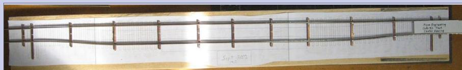
**14. Stock rails in place:** When the stock rails are complete, the scale track is half done and will look like this. Note that the stock rails are not soldered to the two long throwbars, they're just sitting in place unfastened to determine placement for now. The throwbars must be able to move to allow switching the points between the scale and bypass tracks.
