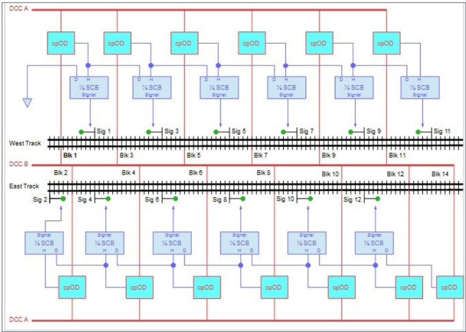
3. Here is the setup for ABS signals on double track. Note it is typical for double track to be signaled for movement in one direction on each track. Going the opposite direction means crossing over to the other track. In this case here, the signals all display green because there is no train on either track.
