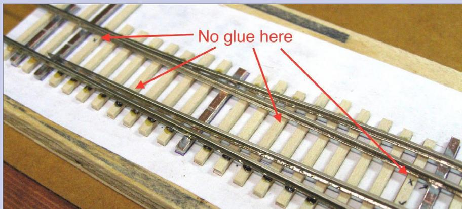
**21. Avoid gluing the movable points area:** *Do not glue the point rails beyond their last solder joint.* The point rails must be able to move! After the Pliobond glue had dried for a few minutes, I carefully set the scale track on a flat surface and weighted it down, then let the glue cure overnight.
