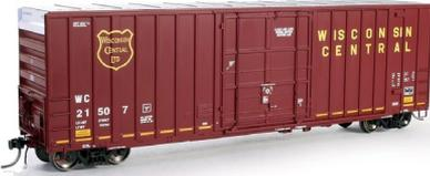
separate door tracks and door bars, etched stainless steel cross-over walks, Kadee #58 couplers, and 100-ton ASF Ride Control trucks with 36-inch machined metal wheelsets.
