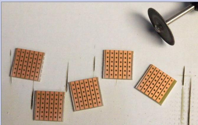
**2. Cut the perf board strips into squares of six holes long.**
