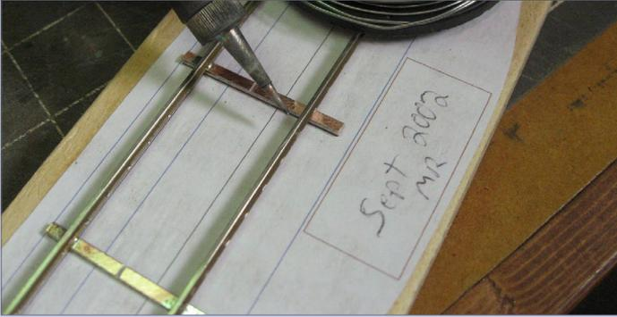
**9. Proper rail and tie prep:** A few light passes of the mill file on the tops of the ties and the bottoms of the rails will remove any tarnish. This way the solder joint will heat quickly and the solder will flow smoothly. Do this file prep now to make the soldering go easier later.
