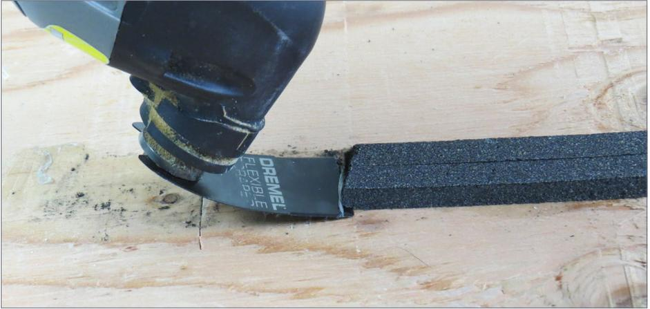
12. The flexible scraper works great for lifting cork roadbed.
