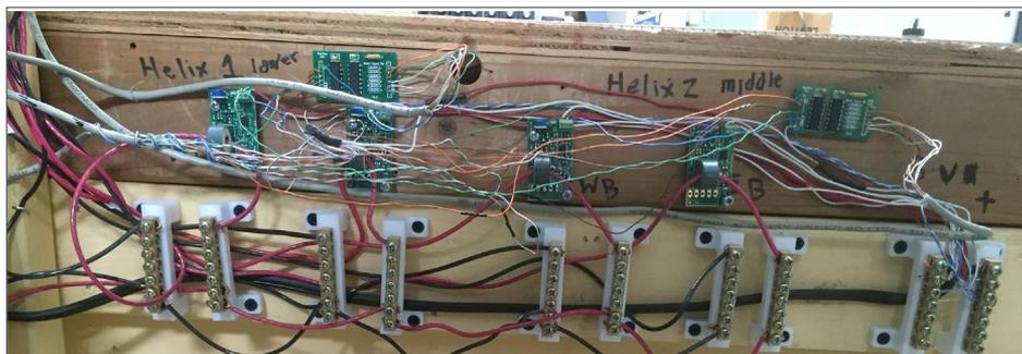
8. Here is one method showing how the SCBs, detector boards and bus connections can be made. At the top of the image you'll see two SCB boards (these are an earlier version without the screw connectors and are mounted to the benchwork with double-sided tape). Since the signals selected by this layout owner came pre-wired with resistors, there are wire jumpers instead of resistors on these SCBs.
