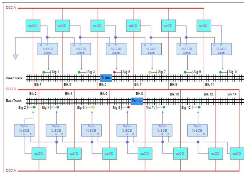
4. Here is how the signals look for double-track ABS with a train in both the east and westbound tracks. The westbound train is in block 7 while an eastbound train is in block 8. In both cases the signals behind each train provide protection for following moves, while the signals in advance of the trains show clear indications.
