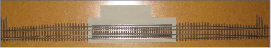
**24. Done and ready to install:** Completed scale track with concrete pad, ready for installation. Note how difficult it is to tell which ties are wood and which are copper clad fiberglass after they have been painted.
