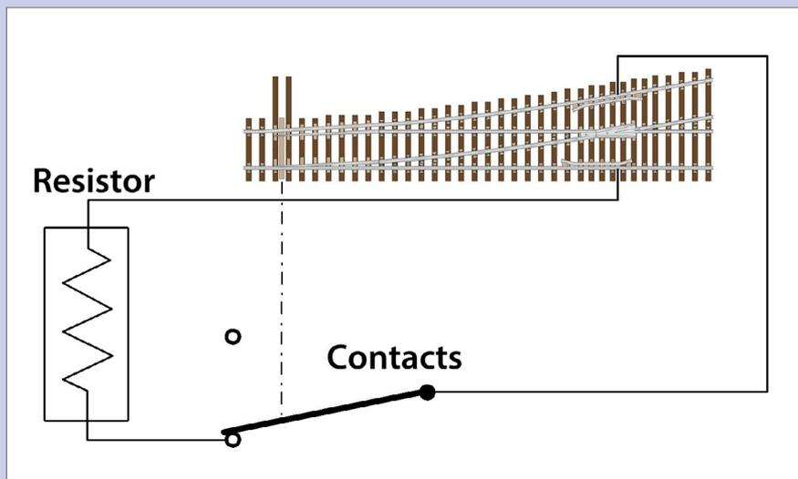
**5. To have a turnout thrown against the main line route trigger occupancy, use contacts to connect a resistor across the rails when the turnout is thrown.**
