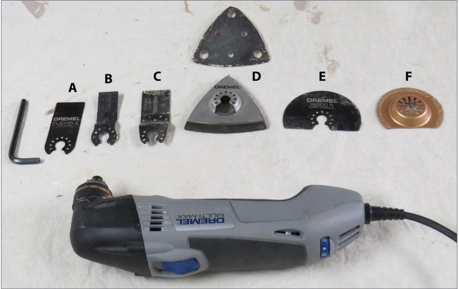
1. Here is the author's Dremel Multi-Max tool with attachments. From left to right: A) Flexible scraper; B) Wood & metal cutting blade; C) Wood cutting blade; D) Sanding attachment and sandpaper; E) Half-moon drywall and wood blade; F) Grinding attachment, purchased separately.
