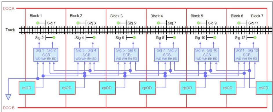
1. Block diagram for a single-track railroad. All signals are green because there is no train on the track. This is the default state for an automatic block system.
