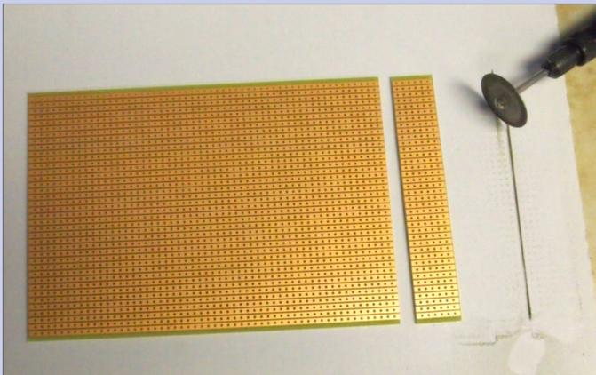
**1. Cut a strip of perf board six holes wide. Use of a Dremel cutting wheel is recommended.**
