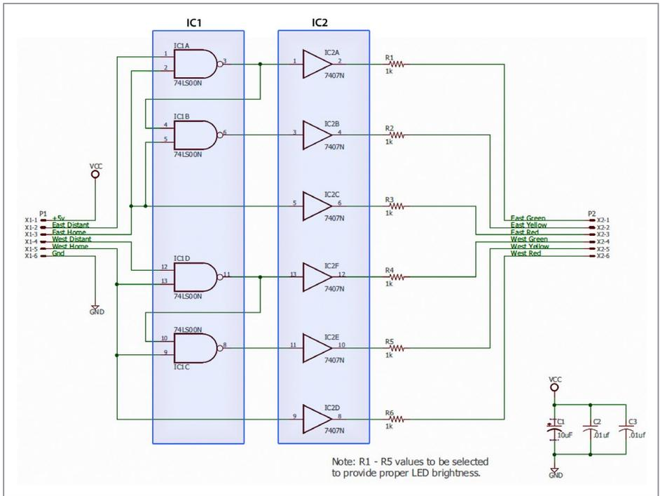
6. Here is a schematic of the Dual ABS (DABS) controller. It is described in detail in the text.
