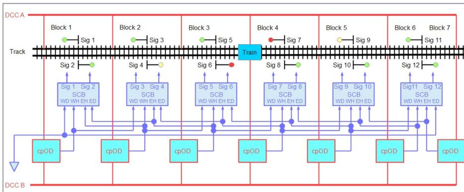
2. What the signals look like if there is a train in the block. In this example there is a train in Block 4. Signals 6 and 7 are red, signals 4 and 9 are yellow, and the rest are green. As the train moves across the layout, the signals will automatically change aspect based on the position of the train. The basic rule is this: signals leading immediately into a detected block will be red, signals one removed from a detected block will be yellow, and all other signals will be green.
