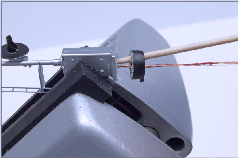
**12. Once I'm about halfway around the black base ring, I flip the signal over in the Panavise and finish cutting through until the black base ring comes completely off. Take care to not nick or cut off any wires!**
