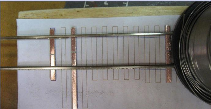
**10. Position the stock rails:** When the two stock rails are ready, carefully align them on the PC Board ties and weight them down so they don't move. I use spools of solder as weights since they are very heavy, flat on the bottom, and just about the right size.
