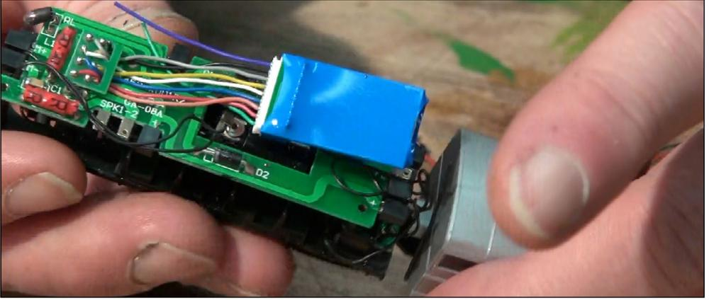
6. I plugged a new Digitrax DH126PS decoder into the model's main board, using the eight-pin harness plug.
