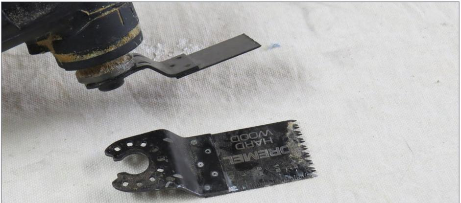
2. Both the wood blade on the tool and the wood & metal offset blade shown below the tool lets you cut flush to a surface.
