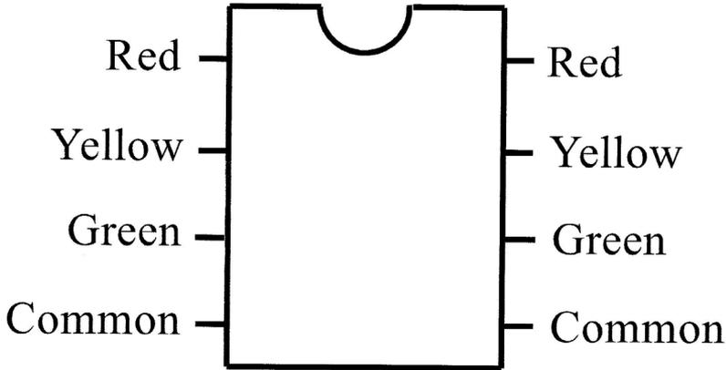
**5. Strip the red, yellow, green, and orange wires from the middle of the 10-conductor ribbon cable that comes with the signals. You will not need the other colors for this project – save them for use elsewhere. Refer to the drawing for the wire locations.**
