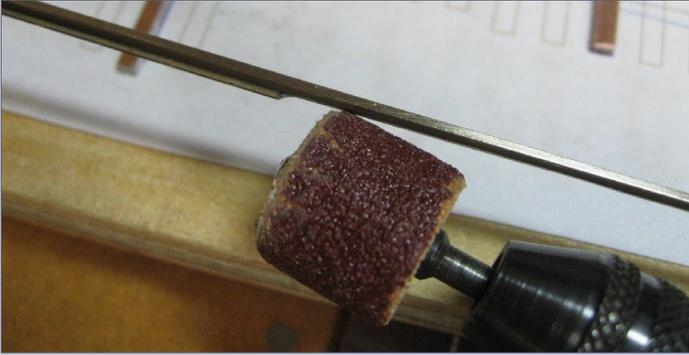
**8. Notch the stock rails:** The two outside rails are the stock rails and need notches filed in them to admit the point rails leading to the scale. Fast Tracks sells a tool called the Stock Aide for doing this ([handlaidtrack.com/sa-m](http://handlaidtrack.com/sa-m)) but I did not have one, so I used a sanding drum in a Dremel rotary tool to notch my stock rails. To do this:
