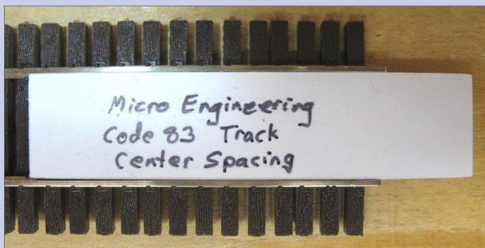
**5. Check the finished styrene track gauge:** When I was happy with my work, I labeled the gauge for future reference. You can see the edges of the gauge aren't perfect, but this method proved workable. I recommend purchasing a commercial gauge for the best results.
