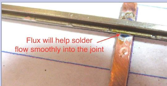
dering iron against the web of the rail. I placed the solder against the PC Board tie at the base of the rail, and kept the hot iron on the joint until the solder flowed. The solder should flow *under* the rail making a solid joint. Excess solder outside the joint is not necessary. The Fast Tracks site has some excellent videos on proper soldering techniques: [[handlaidtrack.com/FTV-Turnouts-5](http://handlaidtrack.com/FTV-Turnouts-5)].
