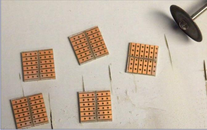
**3. Slice a groove in the center only through the metal to insulate the holes across the perf board squares.**
