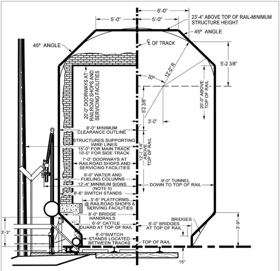
1. A 1977 Union Pacific clearance diagram calls out the proper spacing for various lineside construction and appliances.
