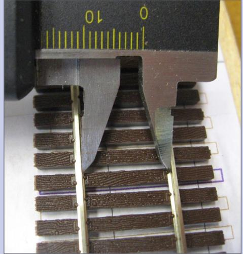
**4. Transfer calipers measurement to styrene:** To begin, I used calipers to measure the distance between the rails of a section of MicroEngineering bridge flex track [3]. Next, I transferred this measurement to a piece of sheet styrene and carefully cut it out. I sanded it as necessary for a good fit.
