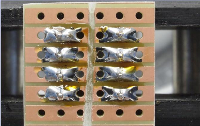
**4. Insert a DIP socket in the center of the perf board square from the fiberglass side, straddling the insulating groove, so the socket legs appear on the metal side of the perf board square. Solder all eight socket legs to the perf board square.**
