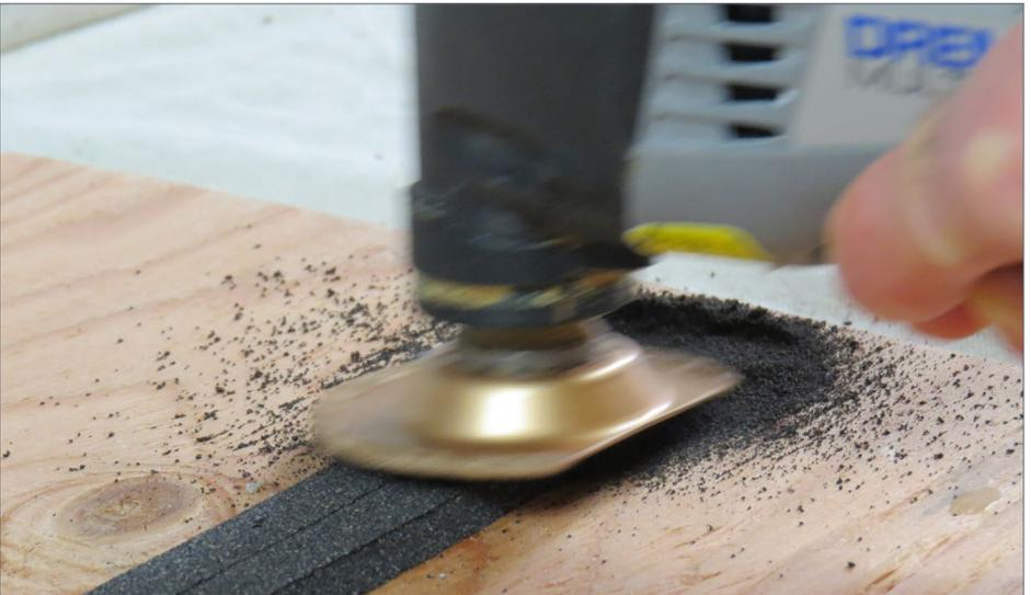
9. The grinding attachment makes short work of tapering cork road bed.
