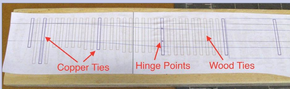
**2. Looking closer at the scale track layout:** Here is a close up view of my plan. I attached the plan to a piece of plywood using spray glue giving me a strong base to support my work. You can see I included a concrete pad on the far right where the actual scale would be. The fourth tie from the left shows the "solder location" for the point rails (that is, the hinge points).
