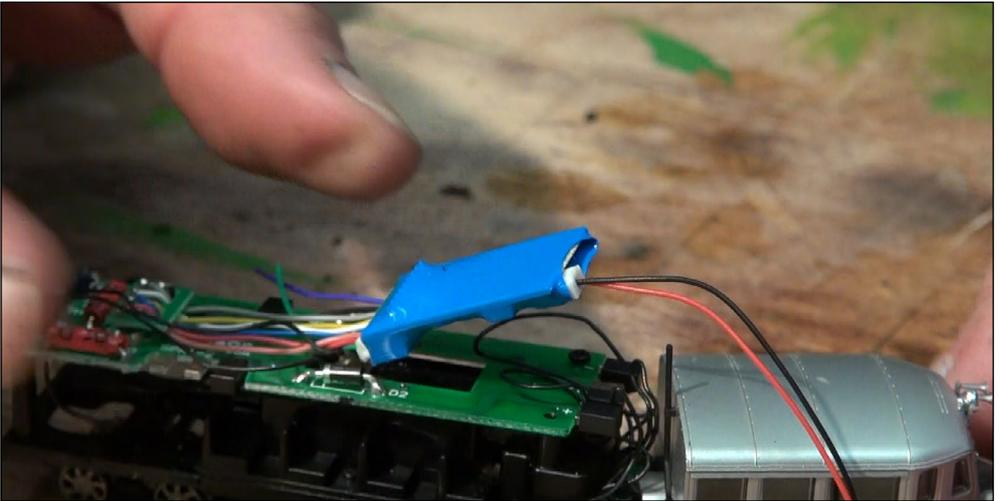
7. The Power Xtender plugged into the two-prong jack on the end of the decoder. That was it. I snapped the shell back onto the model and it was ready to test on the layout. It ran smoothly and did not stall on any of the newly laid turnouts and straight sections of the trackage. When taken off the track while under power, it ran about two feet on the plywood before the power stopped.
