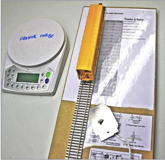
4. A test plank gathers all the tools and tests needed to check a car or locomotive before it is handed off to operating crews on the layout, and is useful in any scale and gauge. Tethering the NMRA gauge keeps it from walking away. *Franck Combe photo*
