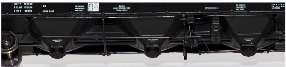
29. CABX 580772, Hopper and brake piping details.
