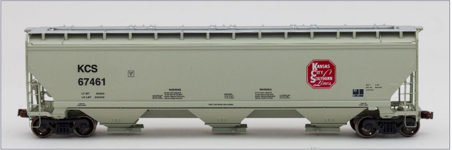
16. KCS 67461 side view, showing the single body style used for the Operator brand 5188 cu. ft. covered hoppers.
