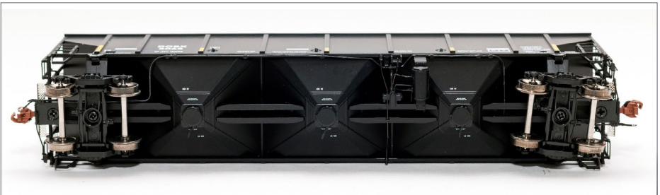
24. DCBX 2065, undercarriage with brake piping and hopper base detail.
