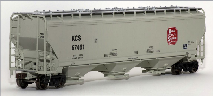
17. KCS 67461, view of B end with brake details and plastic end cage.
