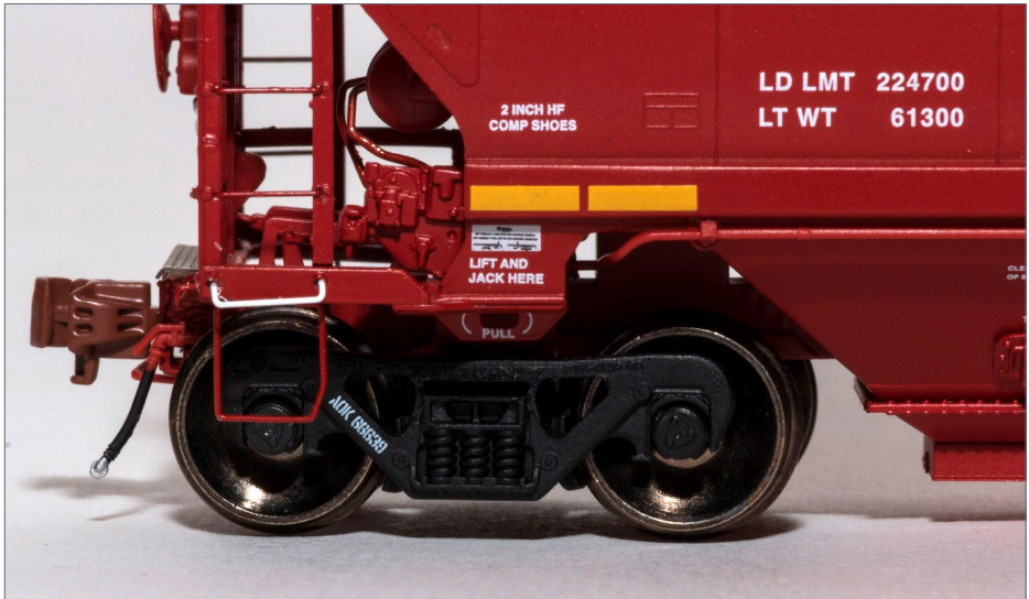
8. AOK 66639, detail view of B end with bolster mounted rope eye and road number printed on truck.
