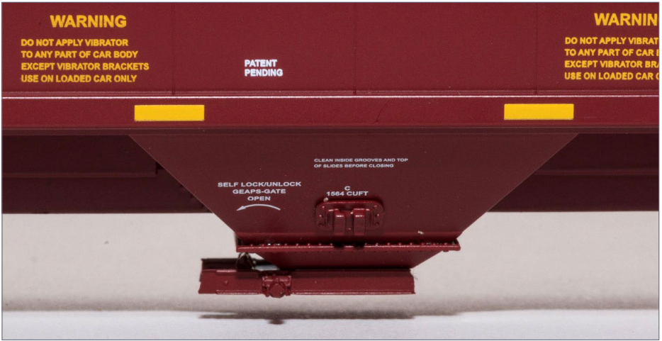
7. AOK 66639, detail view of Miner AutoLok II Gravity Outlets and very small legible printing.
