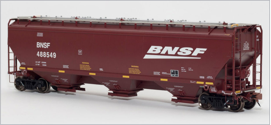
9. BNSF 488549, Version 3 body, equal-width intermediate panels, roping eyes mounted to the side sills of the car body.
