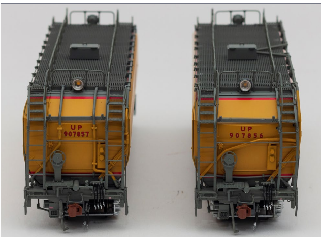
49. UP water cars. B end view. The light on each end is an LED.
