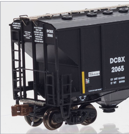
37. DCBX 2065 – N scale Thrall 4727 cu. ft. carbon black covered hopper, A end detail.
