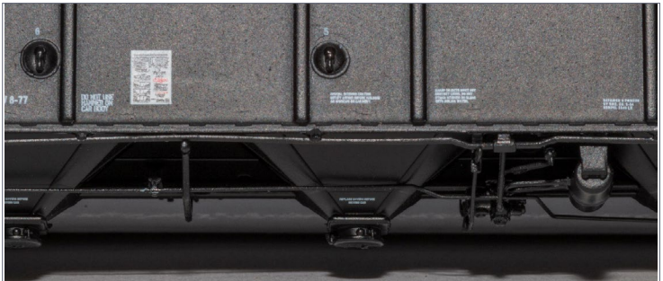
43. WITX 5875, N scale 5750 cu. ft. brake equipment, piping, lettering, and underbody detail.
