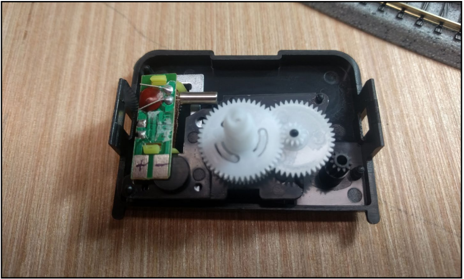
8. Quartz mechanism before disassembly.
