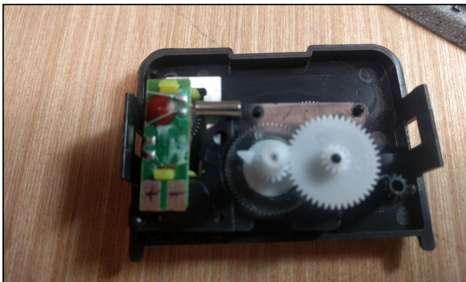
9. Removing the topmost gearing.
