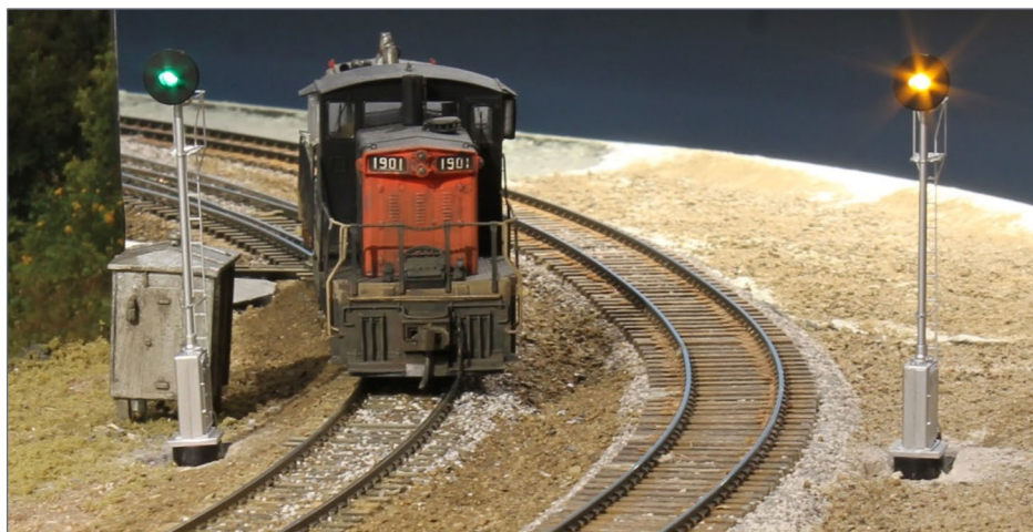
9. Two Signalman-S outputs drive two BLMA target signals. Each signal head has three individual LEDs.
