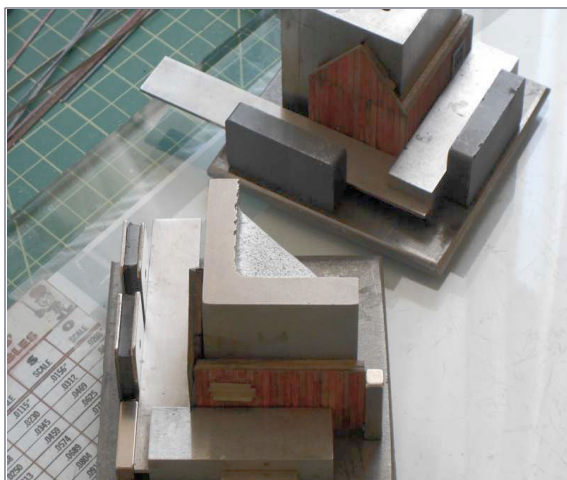
15. My metal block-and-magnets jig made nice, square corners while gluing.
