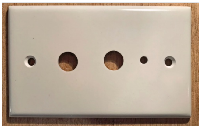
6. Holes for the two pushbuttons and the LED indicator are drilled.
