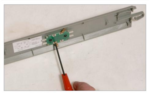
12. Loosen the screws, and the pair of pivoting copper contacts can be rotated 90 degrees to disconnect the two halves of the rails to allow the rerailer to serve as an electric block. There are power connections on both sides of the pivoting contacts, so power for the two blocks can be connected to both blocks at this one site.
