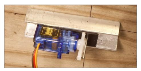
14. Next I thread the wire up through the hole in the aluminum channel, and thread the wire topside through the hole in the throw bar. Then I press the servo firmly into the channel, aligning the wire so it's nicely vertical underneath the throw bar. With this, we're ready to begin configuring the final servo throw!
