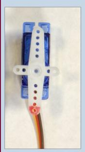
Next, I take some flush cutters and nip off the top part of the horn, leaving a t-shape. I use this t-top crossarm of the horn to hold a trigger wire for a micro-switch (more on
