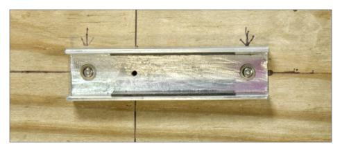
12. Once I had the starter holes for the mounting screws drilled, I mounted the aluminum channel on the underside of the roadbed with the mounting screws shown in [10]. Note how the half-inch hole crosshairs from [6] make aligning the aluminum channel easy – just make sure the thowbar wire hole is in the center of the crosshairs.
