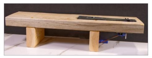
4. I built this servo test fixture using a 2x6 and a couple 2x4s. See text for details.
