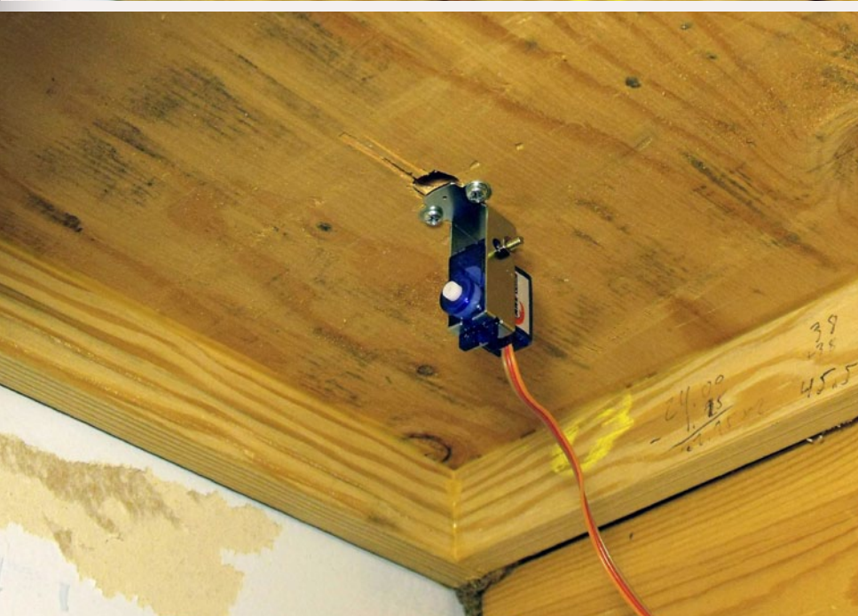
Figure 4: Servo installed in the bracket.
