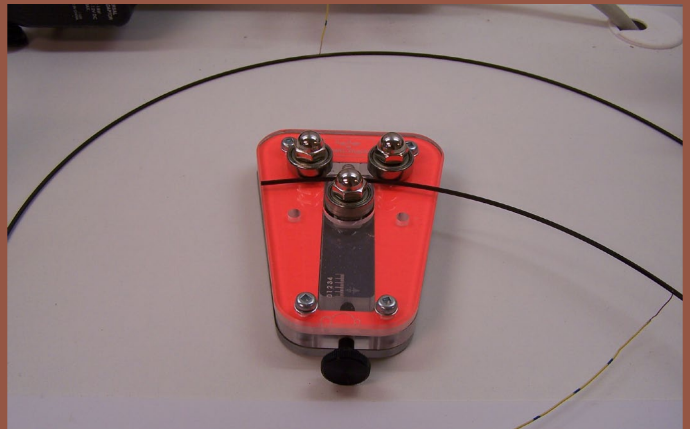
Figure 29: Bending the iron with the Fast Tracks rail bender.
