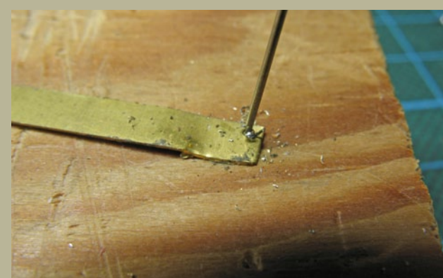
Figure 3: Drilling the #76 hole in the brass strip.
