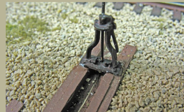
Figure 13: Switch stand glued with CA.
