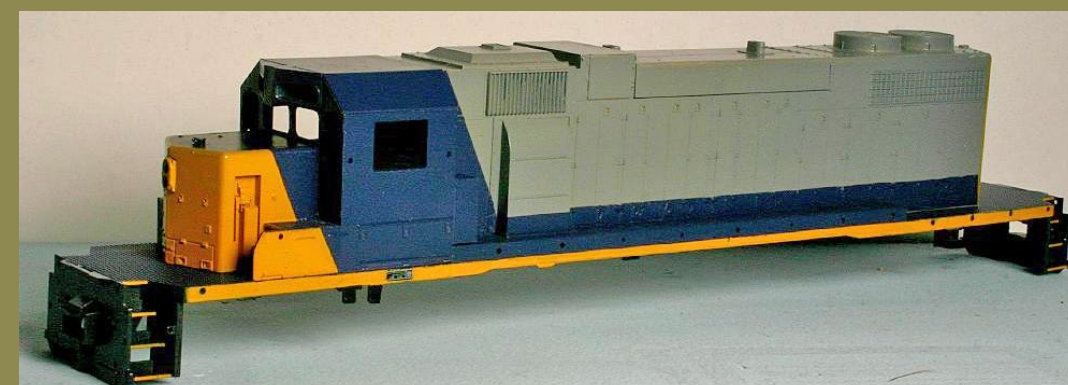
Figure 19: Painted body shell after gloss covering.
