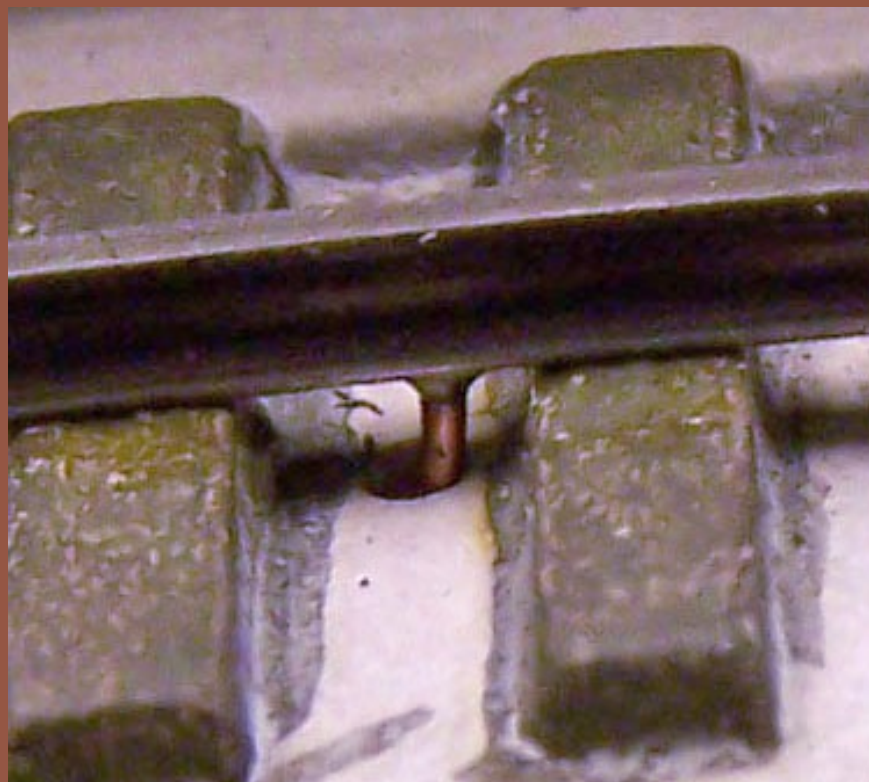
Figure 10: I then threaded the wires through their predrilled holes and secured them on the ties in the pit base.
