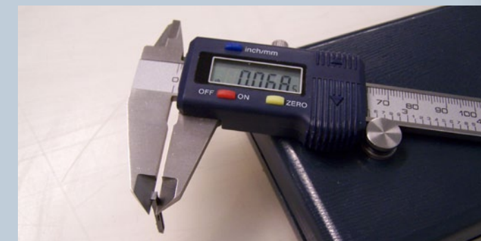
Figure C. CV siding tie is thinner.
