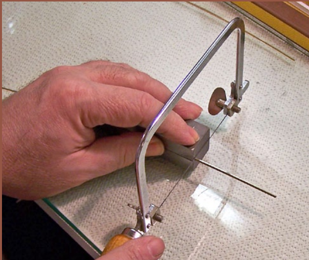
Figure 57: Cutting notch in rail head at 39' intervals.
