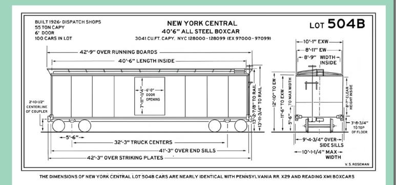
Figure 21: Diagram of New York Central Lot 504B boxcars. Diagram for a Reading XMt boxcar would be similar.
