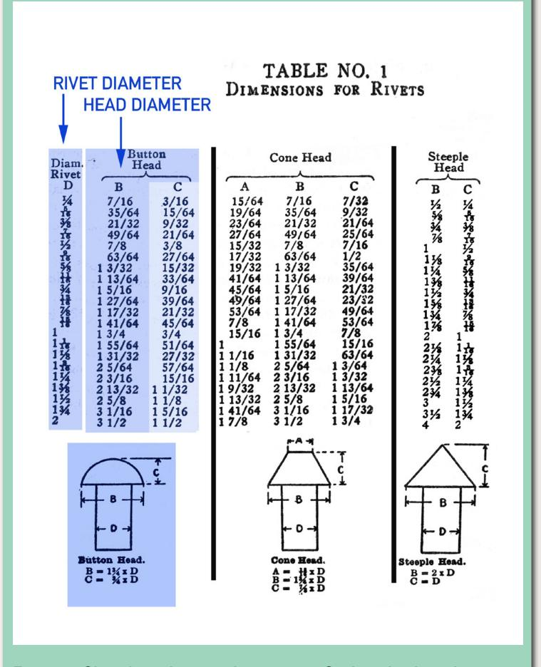
Figure 5: Chart from the 1930 Locomotive Cyclopedia describing rivet forms and head/shank size relationship.
