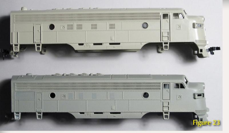
on models. EMD "F" units had louvers between their portholes and some railroads, such as Baltimore and Ohio, plated over the portholes on some of their passenger "E" unit diesels adding louvers instead.
