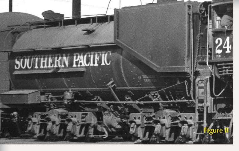
Figure 8: Prototype photo of an SP class 120-C-3 tender.
