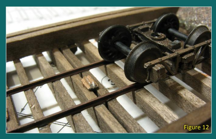
Figures 12 and 13: I also glued the cross beam truss rod saddles. You have to look carefully to pick them out.
