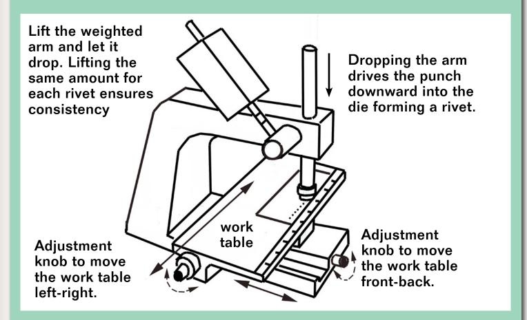
Figure 3: Rivet machine based on an arbor press. The specially tooled die and punch make very precise and consistent rivets in thin metal or styrene. The screw driven work table allows precise positioning for each rivet. But it requires great operator concentration.
