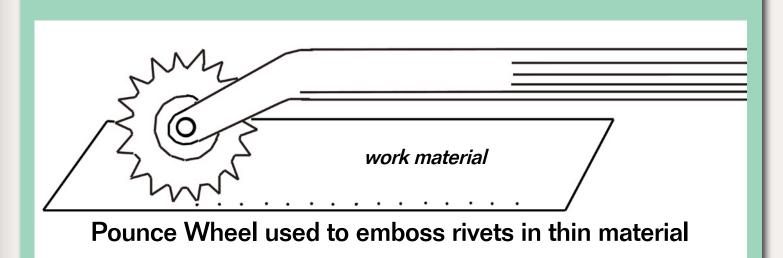
Figure 2: Pounce wheel (or riveting wheel), a simple device for embossing rivets in thin, soft material such as paper or plastic.
