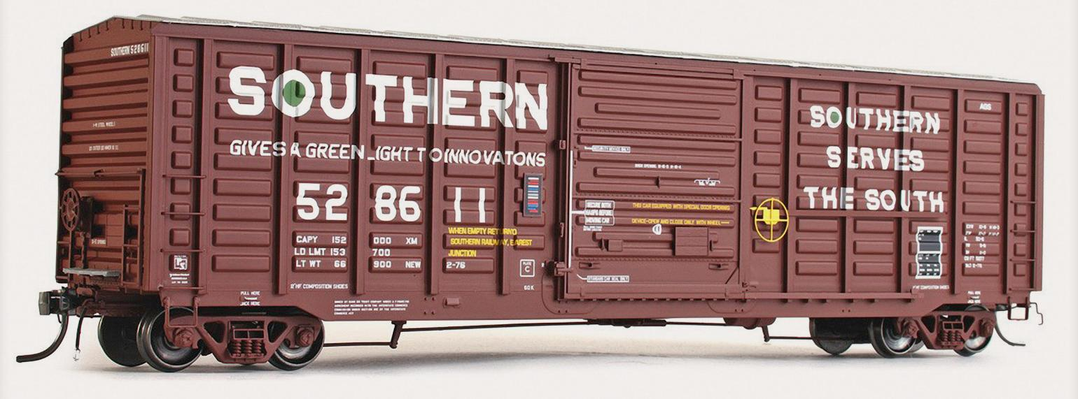
Southern Railway's car number 528611 epitomizes the rugged 60' waffle-side boxcar seen all across America. ExactRail has produced HO scale models of the Pullman-Standard 7315 cu. ft. car in several additional schemes including L&N, NW, BNSF, DT&I, CSXT, ATSF, Milw Rd, NS, UP, and GTW.
