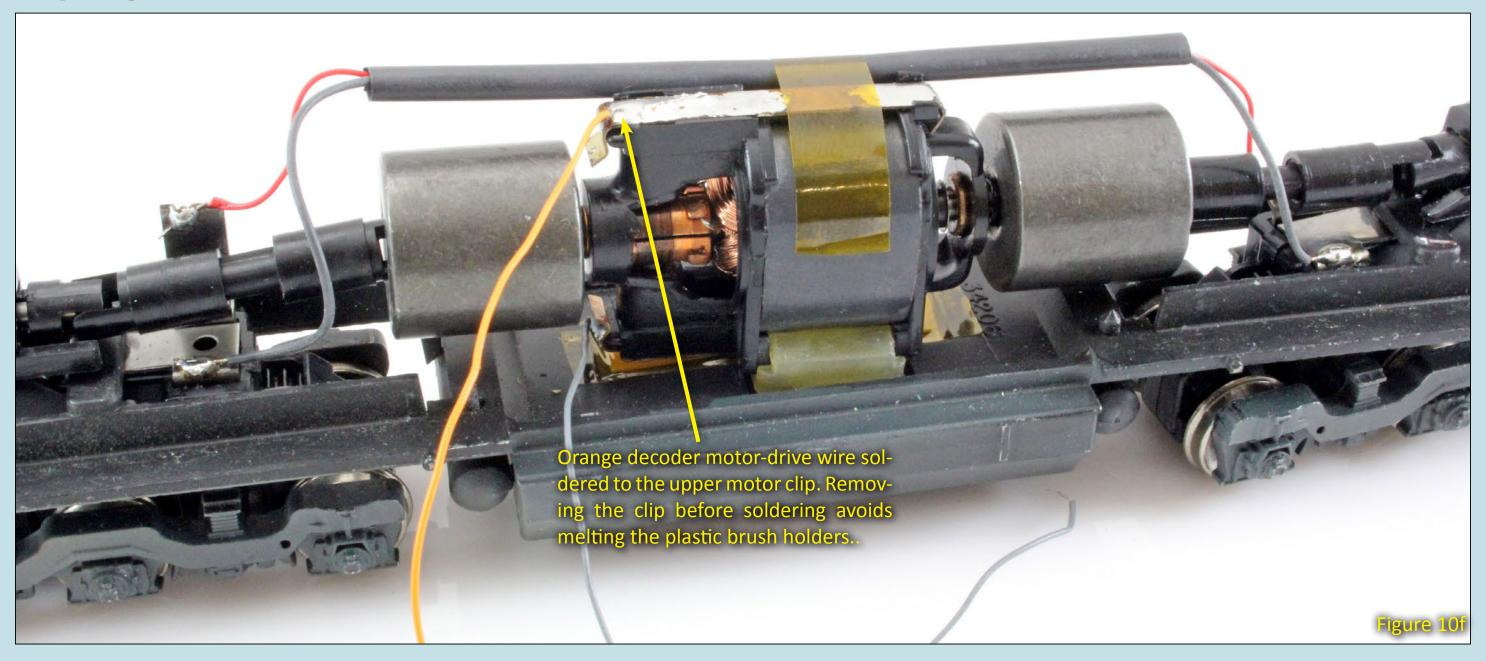
Figure 10f: The motor isolation is complete. This locomotive is ready for decoder installation.
