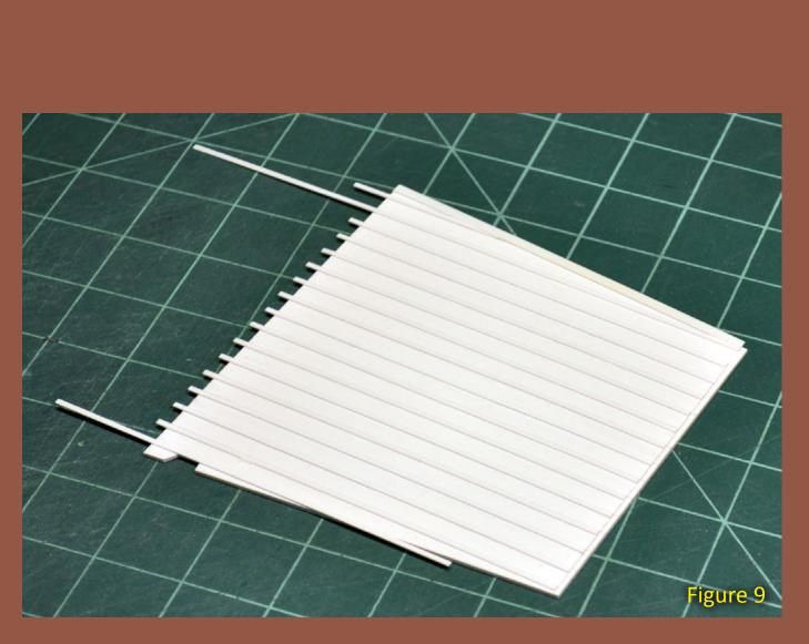
Figure 9: Once the strips dried I did some trimming. Cutting strips over-length and trimming them after assembly gives a neat and wellfinished appearance.
