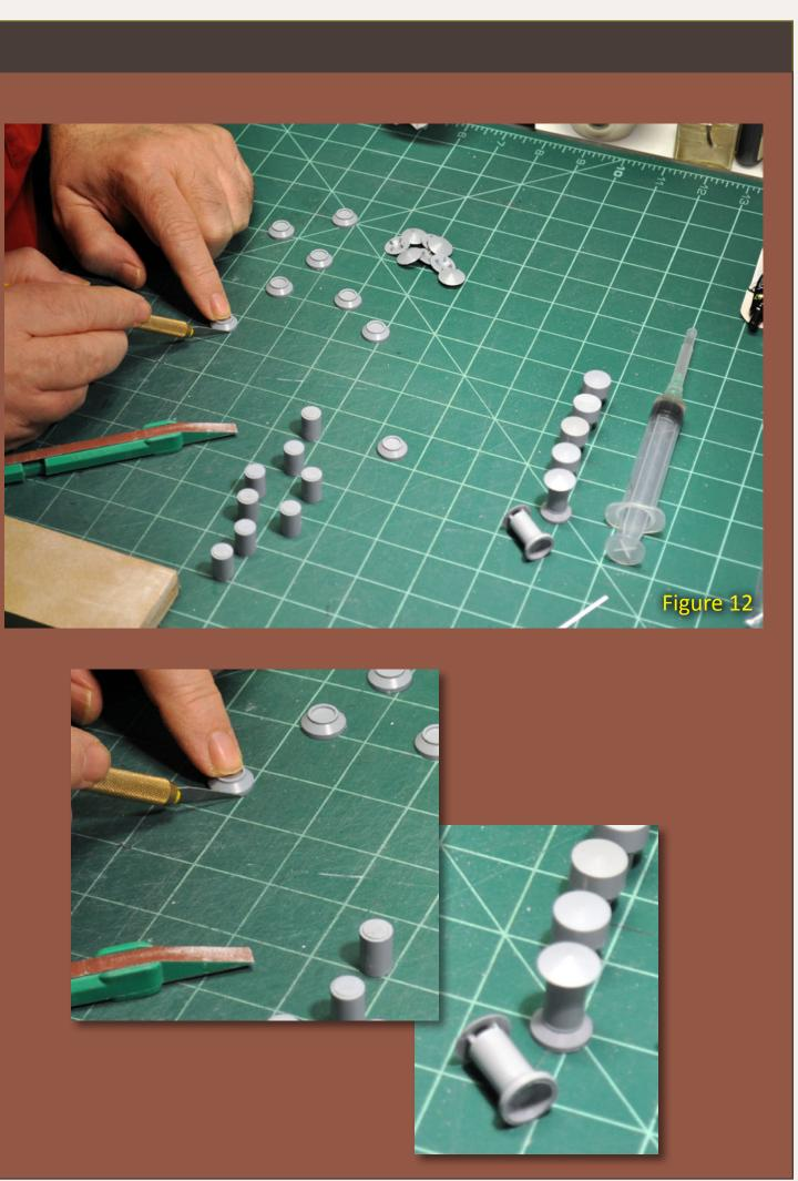
Figure 11: I considered scratch building stacks, but finally decided to use Modulars components from Walthers. I picked the Tall Monitor Vent with Flanged Stack for the machine shop, and the Capped Exhaust Stack for the stalls. In my opinion, these look just right.
