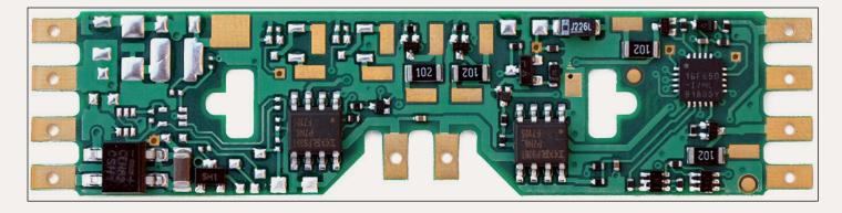
Figure 2: The TCS A4X decoder is an example of an open board decoder - photo courtesy of Train Control Systems.
