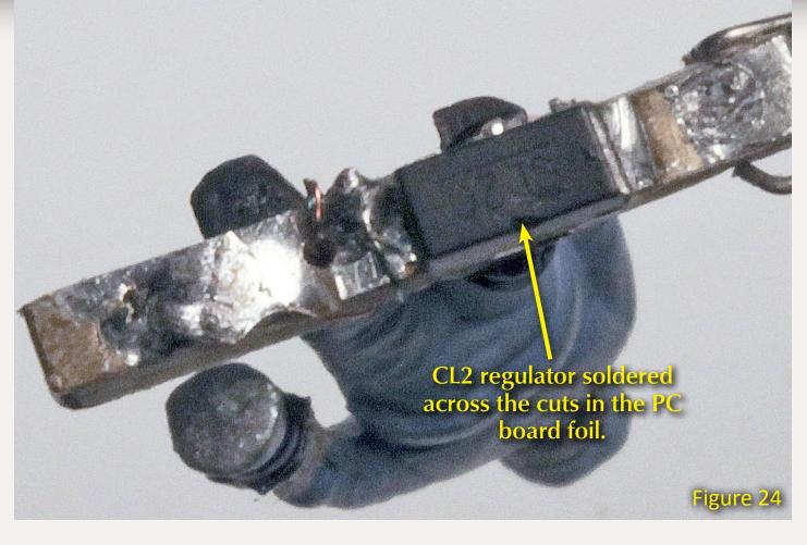
for the back contacts of the CL2 regulator so you can solder it to the strip. Clip off the third "no connection" pin from the CL2.
