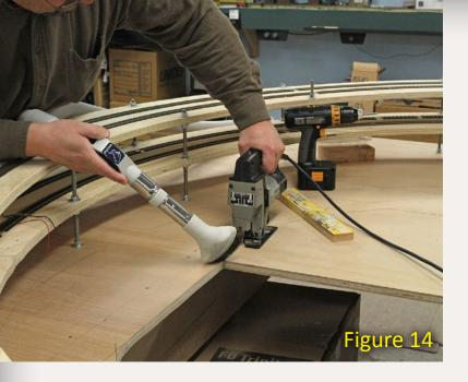
Figure 14: I've almost finished cutting out the second part of the central helix pit. Again I'm using cleats to prevent the heavy chunk of plywood from falling. The vacuum greatly reduces the dust released into the layout room.
