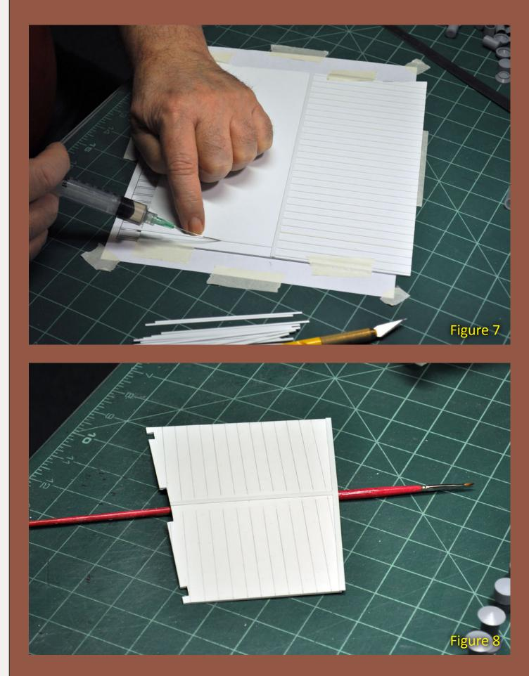
Figure 7: Using the drawing as a guide, I positioned the strips and glued them to their roof panel with MEK. I use a syringe to apply MEK because I can precisely control how much MEK I use – at least most of the time. More on this later ...
