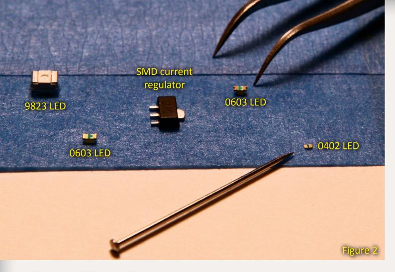
Figure 2: Different LED types. Note the wide range of sizes going down to roughly that of a pin point.
