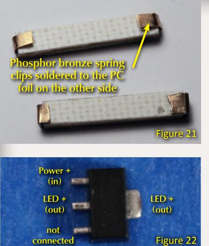
Figure 21: SINGLE-sided PC board for mounting the workman.
