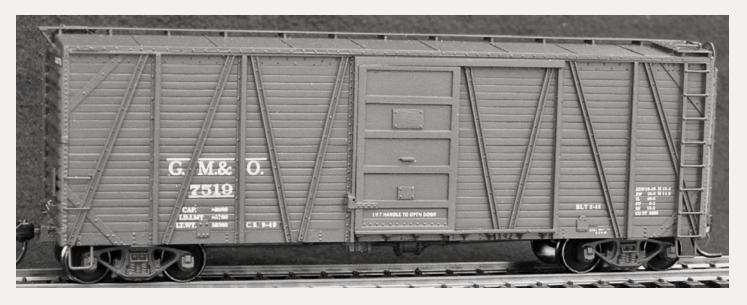
Sunshine also has the 10'3" ACY and GM&O cars with improved Dreadnaught ends and Pullman steel doors (above), as upgraded on the prototype beginning in the mid-1940s. Sunshine kits come with extensive instructions and a prototype data sheet, proprietary decals and all necessary detailing parts except trucks and couplers. They are priced at \$42.00 each.
