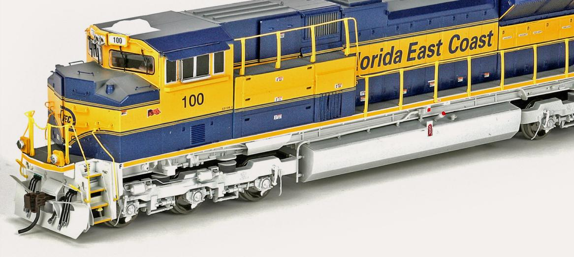
The modern SD70M-2 diesel locomotive was developed by EMD to meet strict emission standards imposed by the EPA. The diesel's 74' 3" frame mounts a 16-cylinder engine capable of generating 4,300 horsepower. External spotting features include a full-height nose door, rectangular windshields, large flared radiators with two fans, and the dynamic brake equipment located at the rear of the long hood.
