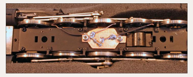
Figure 5: Added opposite rail pick-ups in an O-scale brass loco - similar pick-ups were added to the tender on the opposite side. The drivers equipped with wipers are insulated between the wheel tread and the inner parts. Note the wipers only touch the outermost portion of each wheel to avoid bridging the insulation and causing short circuits.
