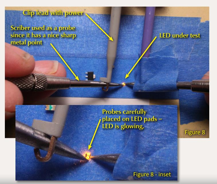
of a very thin piece of wire (I use 38 gauge magnet wire) against the SMD LED held by the right clip, so it can be tack soldered to the LED. Remember, minimize the independent movements required in performing every step with the LEDs. A similar tool can be purchased from ngineering.com/other cool tools.htm#LEDholder
