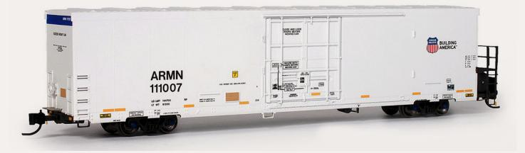
**ExactRail** (exactrail.com) has released an N scale version of the Trinity TRINCool 64' reefer car decorated for UP/ARMN in 24 different road numbers. Priced at \$29.95 each, the ready-to-run model features body mounted draft boxes with Micro-Trains<sup>®</sup> 1016 couplers, separately applied uncoupling levers, wire grab irons, etched-metal reefer platform, and ASF 100-ton trucks with machined 36" wheels.
