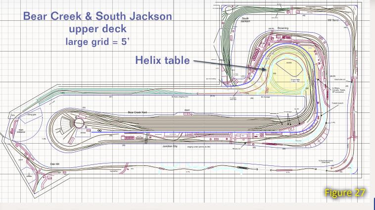
Figure 27: The current BC&SJ upper-deck plan. The peninsula is still under construction – there is no upper-deck yet. South Jackson, shown in green, has been substantially redesigned compared to the "scrap box" version (called that because it was hastily thrown together using plywood, screws, track, and wire salvaged from the previous BC&SJ). Zoom to expand the track plan for readability or <u>click here</u> to download a .pdf file of the plan.
