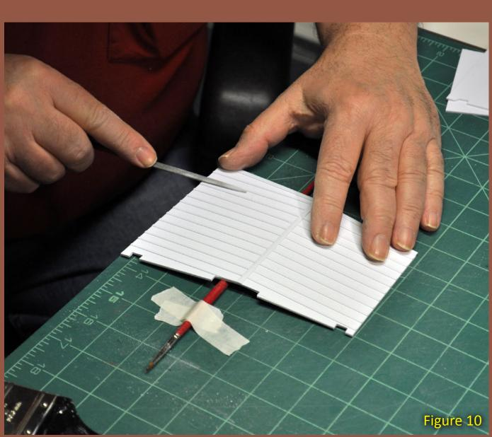
Figure 10: Despite using the syringe to dispense MEK, I'd managed to get some excess between the ribs in a place or two which messed up the plastic surface. Being as careful as possible, I filed and sanded this area smooth.
