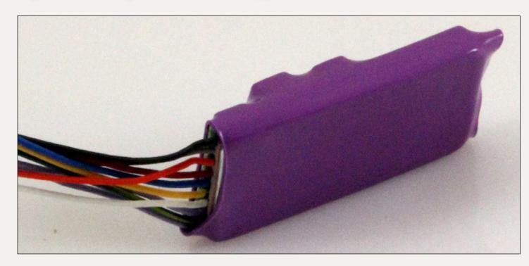
Figure 3: The SoundTraxx Micro Tsunami is an example of a wrapped decoder. In this photo, the heat sink side is toward camera.
