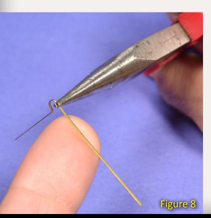
each piece and have them join at the center of the mast on each side, the loops would have been too small to manage, at least for me. Start by forming the brass into a loop by wrapping it around the mast (figure 7).
