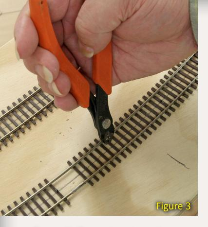
Figure 3: Removing three ties where each optical detector will be mounted.
