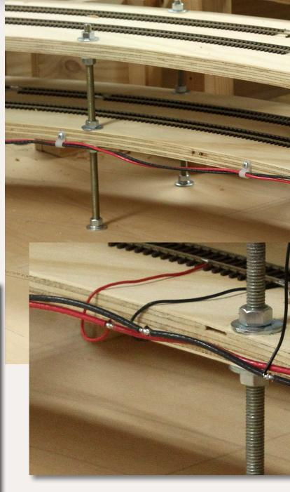
of the lower roadbed using plastic cable clamps to hold them in place (figure 16 and 16a). I soldered the 22-gauge feeders to the bus wires for reliability.
