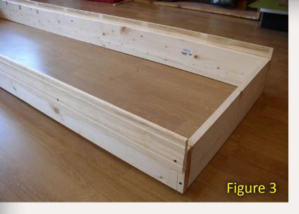
the sides (figure 3) to hold the pinkfoam-based scenes in place. The legs may be unbolted for transportation.
