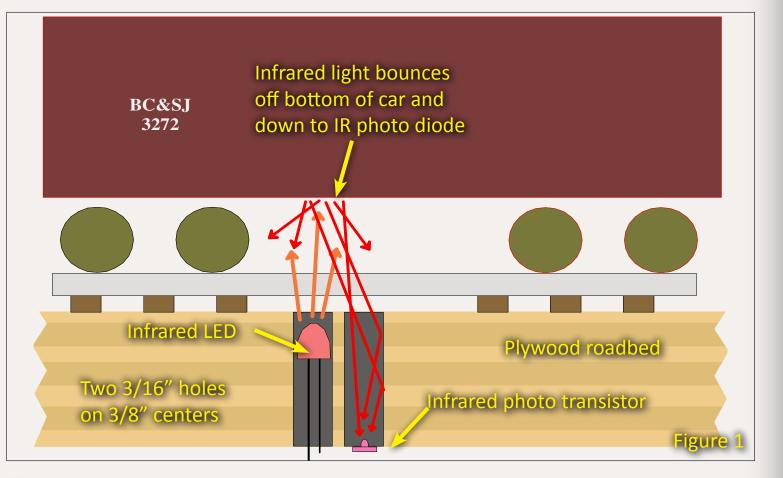
Figure 1: Holes in the roadbed contain an infrared LED and photo transistor. Light bouncing off the bottom of a passing train is detected by the photo transistor.
