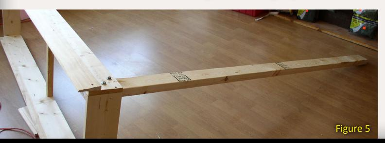
pine, the rim boards are 5" decorative pine baseboards (normally they'd be used where a wall meets the floor in a house). Legs are 2x4s. My cradle is 8' long by 2' deep by 54" high from the top of the four pieces of 2" thick foam (figure 6) to the floor. The legs have 5/16" lag screws screwed into their bottoms to provide height microadjustment.
