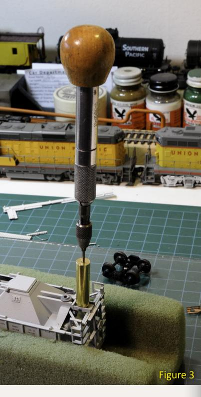
Coupler mounting post with #50 nole arilled precisely in its center.
