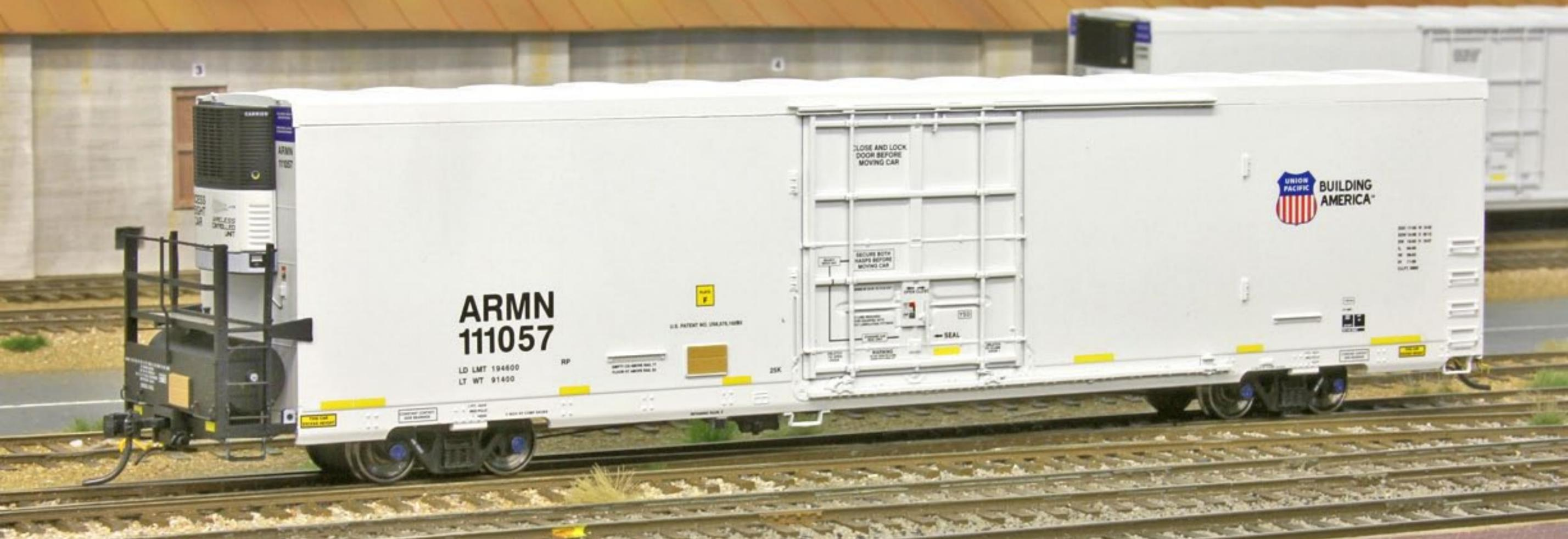
Introduced by Trinity Rail in late 2003, the 64' modern reefer/boxcar was designed for increased capacity, better protection during shipping, and greater loading and unloading efficiency. The Plate F, excess-height car provides a spacious interior that can handle the contents of four 53' truck trailers. The unique cars have successfully brought new life to the movement of refrigerated produce and other perishable goods.
