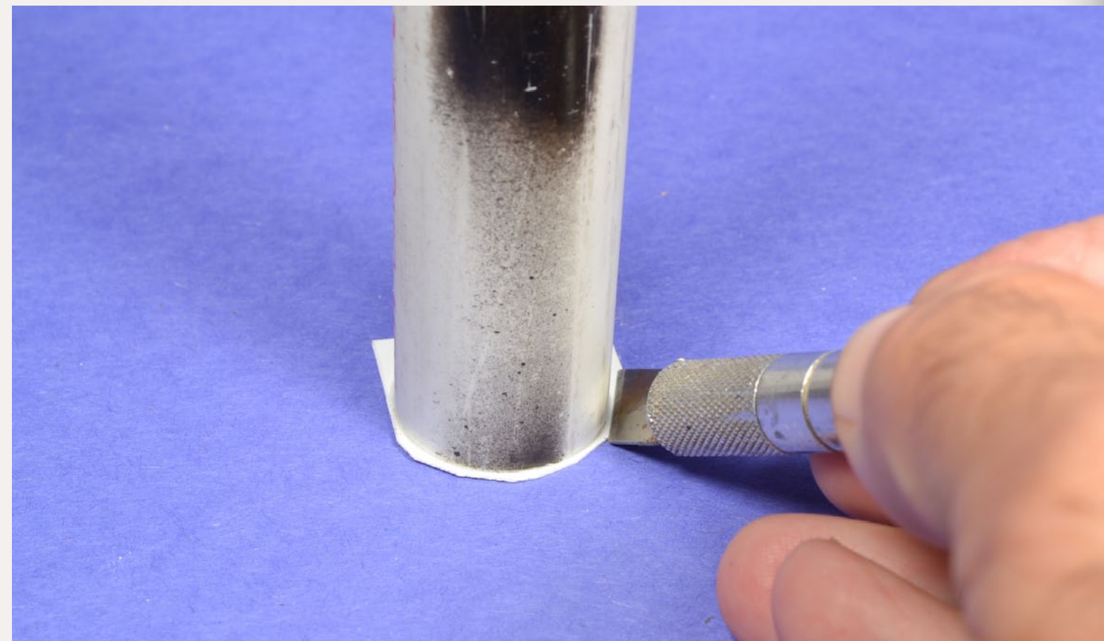
Figure 4: Trim the styrene close to the edge of the PVC pipe.
