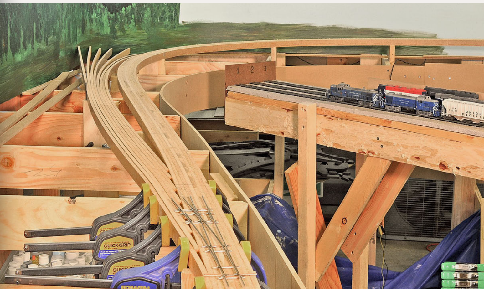
Figure 2: Smooth spline has to be laid out with care. This lay-up, with jagged edges abutting the main where the switch splits off to the left, was rejected in favor of attaching one long strip along the main and building the additional splines onto that.
