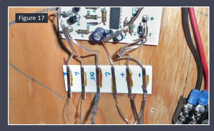
Figure 17: I carefully threaded the wires from the signal post down through the base tube, and then soldered one each to the L and R ties on my terminal strip. I also soldered two 1000K resistors in series to the end of the common (base tube) lead, encased them in heat shrink insulating tubing, and soldered the other resistor lead to the Out terminal.
