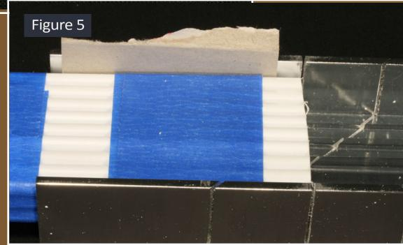
Figure 3: After cutting the tubing to length, it can be placed on a flat surface. Each tier can be constructed, combining the individual tubing sections into one solid layer that is easier to handle.
