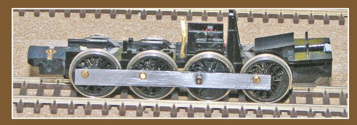
Figure 29: It's not exactly prototypical, but this side rod runs smoothly and that's all that really counts. There's no point spending time dressing it up unless it works well, so testing and fitting are important.
