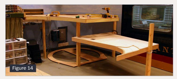
Figures 13-14: Placing the 2x4 legs, and the second level underneath.
