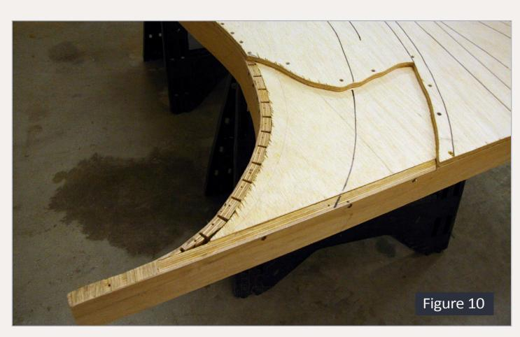
Figures 10-11: These photos show the notched curves created in the plywood.
