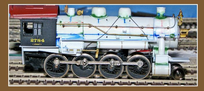
Figure 12: I've added the handrails, sand lines, and feedwater pipes. You can also see the generator and modified whistle.
