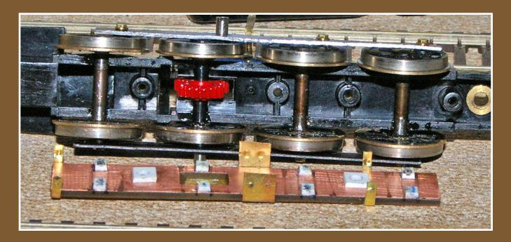
Figure 22: Before going to sprung plunger contacts, I made some simple wipers out of brass. They probably would have worked better if they were a little thinner, but these were too stiff and caused too much drag. You can see the styrene pieces I added to keep the axles in place, replicating cast on nubs on the original piece.
