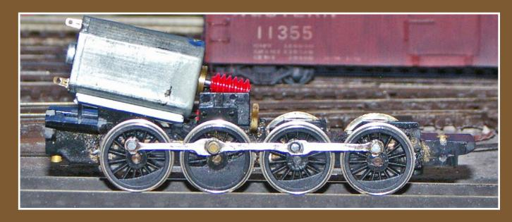
Figure 30: The new rods have a much finer profile than the originals did.
