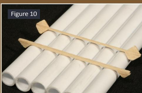
Figure 9: The first step in applying end chocks is to add them to the top of the runner strip along the edge of the two outermost pipes.
