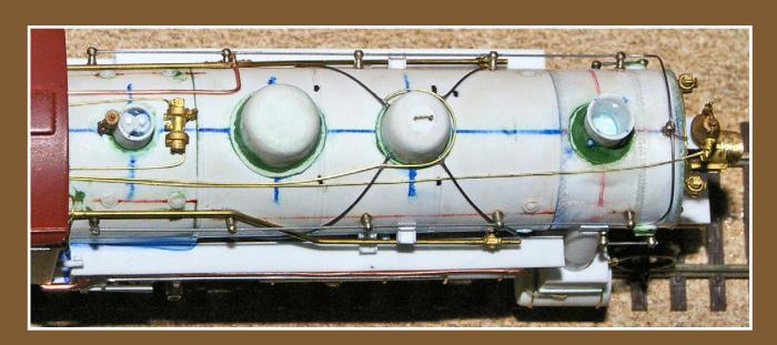
Figure 19: This is a good top view, showing the arrangement of the plumbing as well as the homemade pop valves. It also shows how thin the lip of the stack can be made, even in styrene.
