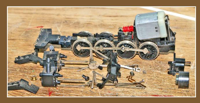
Figure 20: There is a lot on the chassis that is going to be replaced or is in the way. I left the pilot deck for the moment, until I knew exactly how much had to be removed and how I was going to design the cylinders and new deck.
