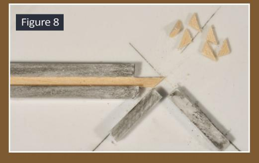
Figure 8: When cutting large quantities of identical pieces, a jig will help insure identical cuts, while saving much time.
