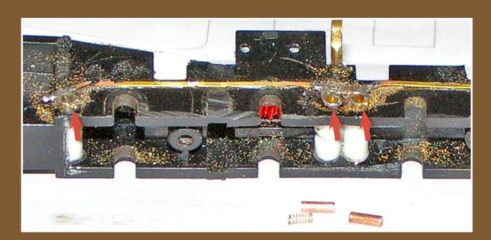
Figure 24: The plunger type wipers (at red arrow locations) are remarkably simple and effective, although the springs cause pieces to go flying when the drivers are removed! The white tubes inside the frame hold and insulate the brass contact tubes.
