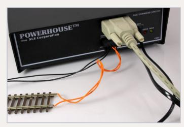
Figure 5: NCE command station with RS232 cable interface.
