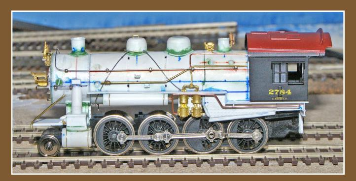
Figure 17: This is the finished fireman's side. You can see the steam and air lines for the compressors.
