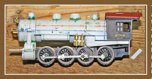
The pop-valves are made from the same tubing and rod used to make the cleanout plugs in the boiler. The tubing should be just over half the inside diameter of the turret. Cut
