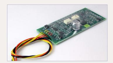
Figure 9: SoundTraxx' PTB100 Programming Track Booster.
