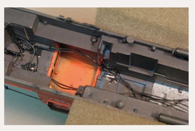
Figure 6: Wires are placed to clear the front truck gear tower. The shiny areas are the 'dry' (sticky) glue areas.
