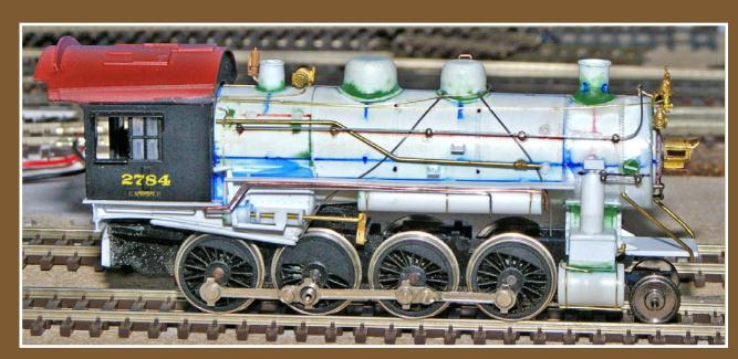
Figure 16: Here you can see the brake pipe, cooling line for the main reservoirs, air lines for the bell ringer and sanders, and the ash pan fitted to the bottom of the firebox. There are also lines running to the generator and power reverse. The engineer's side detailing is done at this point.
