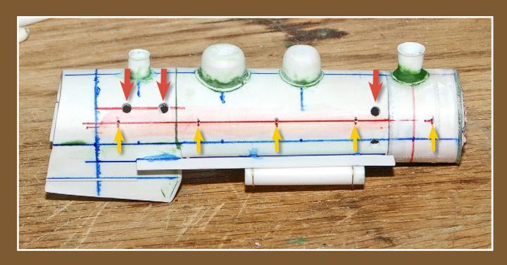
Figure 2: The holes are drilled for the cleanout plugs (marked by red arrows). They look large now, but they will look smaller when they're filled in. I have also drilled the holes for the handrail stanchions (yellow arrows).
