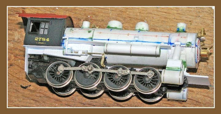
Figure 9: This is the scratchbuilt power reverse, in all its glory. By imagining it as a collection of basic shapes, it's simple enough to build.
