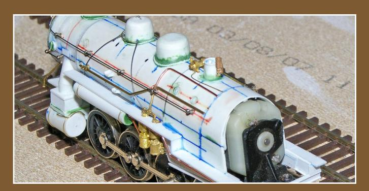
Figure 18: Rather than continue the plumbing inside the cab, with the associated challenge of fitting it through the cab wall or fitting the cab around it, I chose to simply end the plumbing at the cab wall. It's nearly invisible unless you look very closely, and it made construction a lot easier.
