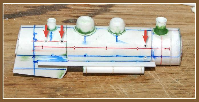
Figure 3: The first step in making cleanout plugs is to make the plug body by gluing in sections of styrene tubing, and then enlarging the opening slightly (red arrow locations).
