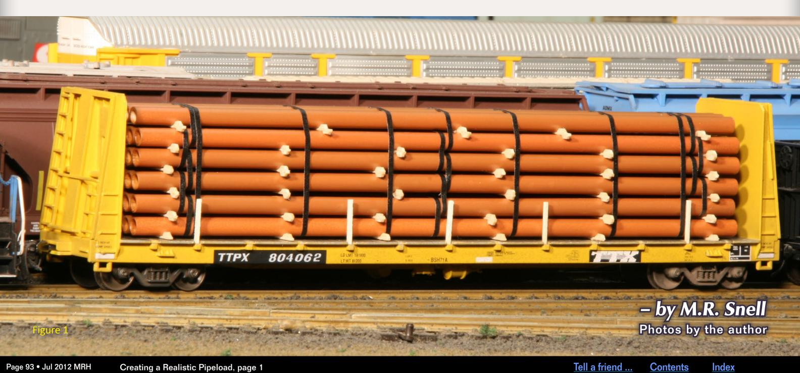
end-to-end the bulkheads would prevent either single or multiple pipes from traveling into the adjacent cars.
