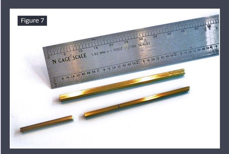
With both LEDs prepped, I began work on the sign post and mounting base. I cut two lengths of 3/32" tubing, one 2-1/2" long and the second about 1". I also cut a 3" length of 1/8" tube. The 1/8" tube will be the base of the sign post, and since this will form part of the conduction path for the common lead, it has to be long enough to extend below the layout. My benchwork is 2" extruded foam glued to 1/2" plywood, so I cut my base tube 3" long, but this will vary for other types of benchwork.
