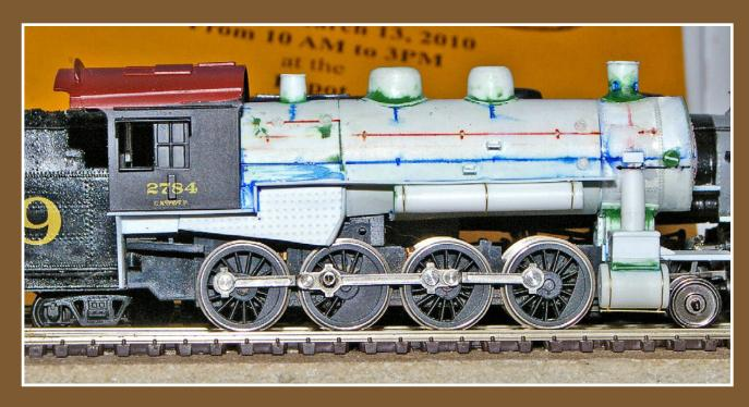
Figure 7: The firebox overlay is in place here, along with the smokebox cleanout and builder's plate. Also clear in this angle is how the #3 driver is recessed into the firebox, a compromise required because the drivers are too large and too widely-spaced, compared to the prototype. Many commercial models are lengthened to disguise this, but I chose to make the boiler the correct prototypical length.
