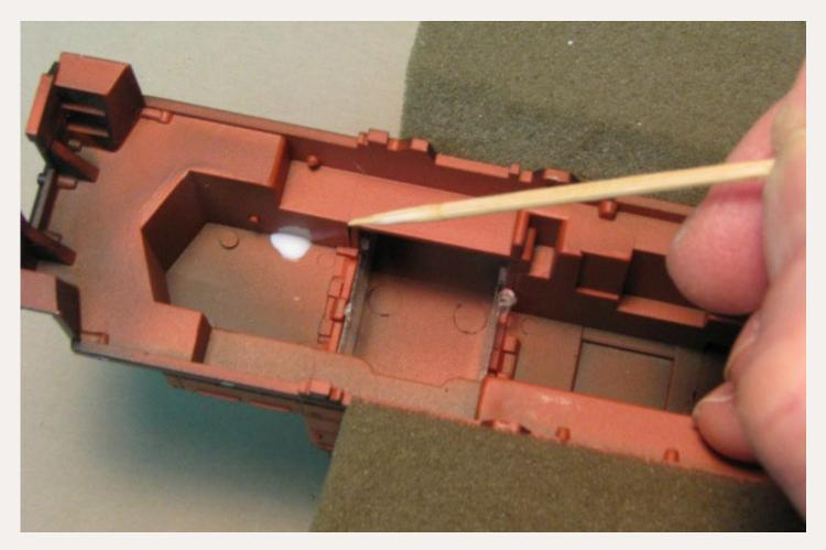
Figure 5: Apply the glue with a toothpick or Microbrush. Neatness isn't critical, but try to keep the blobs small.
