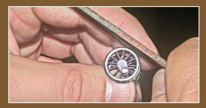
Figure 25b: Filing down too-deep flanges on a driver.
