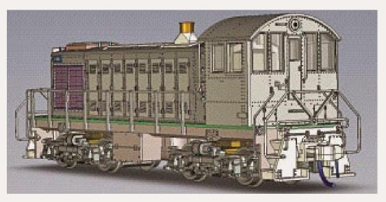
electrical pickup, all-wheel drive, directional lighting, flywheel drive, DCC-ready plug, and both horizontal and vertical grilles as appropriate to the prototype being modeled. Information about road names and pricing is expected to be announced soon.
