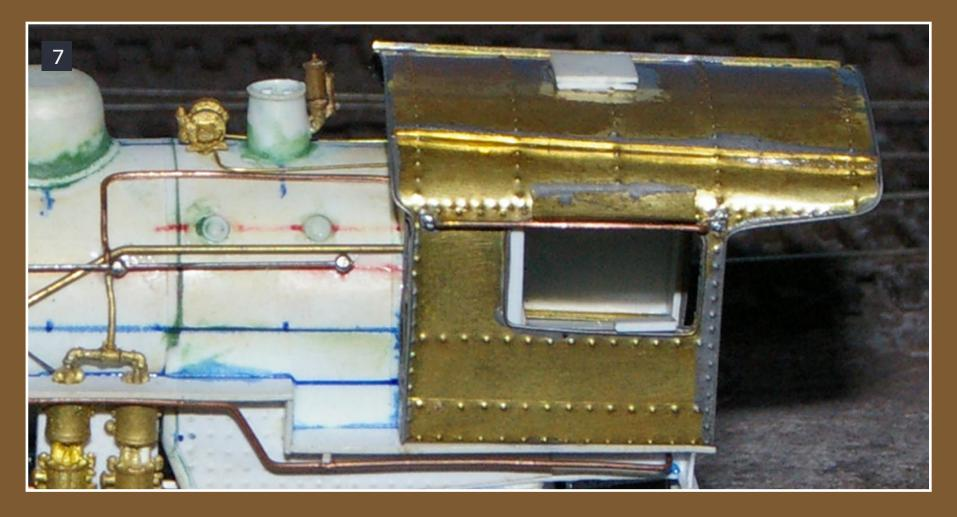
7: The drip rails are angled down toward the rear, to help channel rain away from the doors and windows. On the model, they're just soldered into place, positioned by eye.
