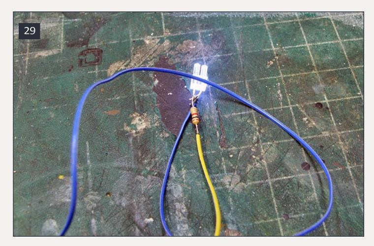
29: Wiring for front headlight LEDs.
