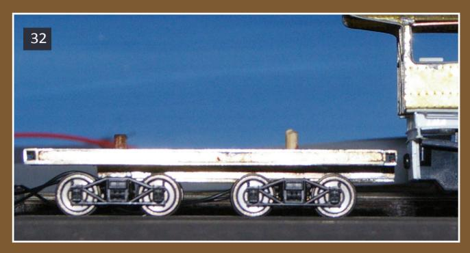
31. To test the height of the floor, I stuck some pieces of bamboo skewer in the trucks and slid them in the holes. 32: The bottom of the center sill just happened to come out almost exactly the same height as the rear of the loco frame. That makes mounting the drawbar very easy.
