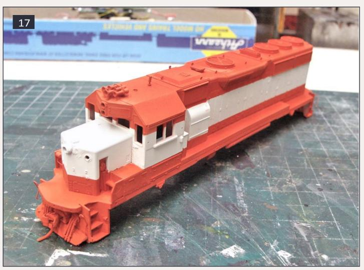
Figure 17: Loco shell after spray painting the Frisco Mandarin Orange (see text for exact color source) and removing the tape masking.
