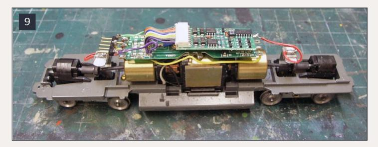
9: Gold-plated Digi-Key plug on the left end of the loco circuit board, to allow easy connecting and disconnecting of the lighting wires inside the loco. Also note the routing of the yellow and gray wires.
