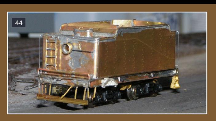
44. I chose a brass air hose on the rear, for added strength. All the details are in place at this point.
