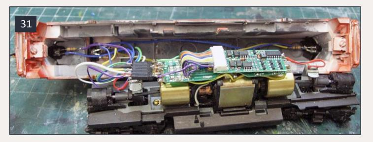
31: Completed shell with the headlight wired to the front socket. Using this socket makes it easy to disconnect the headlight wiring and completely remove the shell from the chassis.
