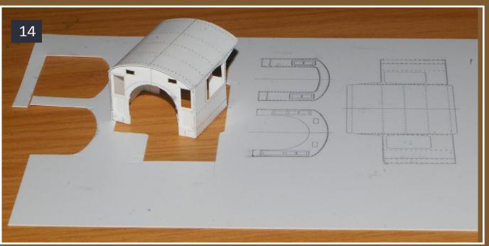
13: The internal bracing has been glued to the backs of the parts. It will be trimmed to length after the glue dries completely. 14: The cab is glued up and sitting on the sheet from which all the parts were cut.
