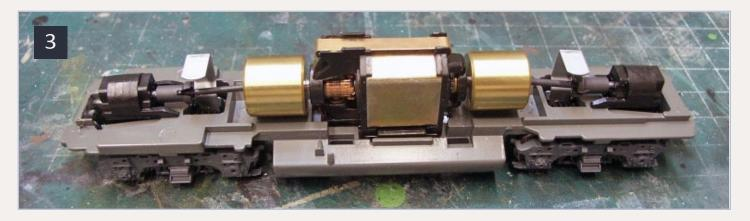
3: GP40-2 chassis, with the Athearn DCC-ready circuit board removed.
