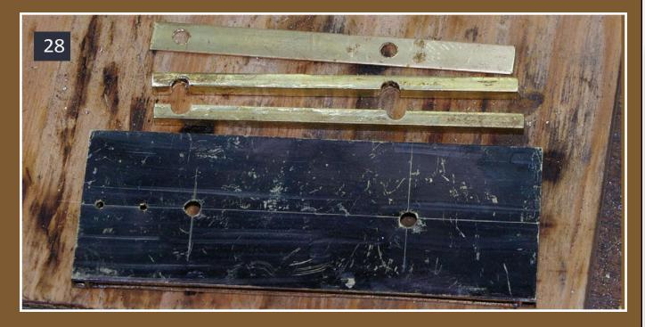
28. Since I don't have any layout dye (used by machinists to make marks visible on metal) I use a cheap marker. I've drilled the holes for the truck mounting pins and coupler box. Above the frame are the parts that will become the center sill.
