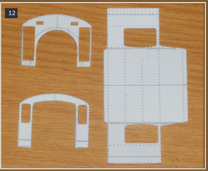
11: The .010" styrene after printing. I have marked the front of one cab for a smaller boiler opening.
