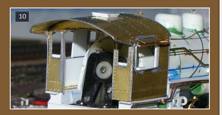
10: The rear windows on the prototype's cab slide down to open. As with the side windows, I modeled them open to make my life easier.
