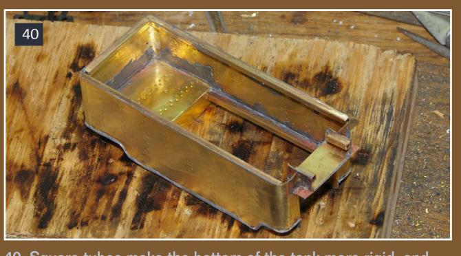
40. Square tubes make the bottom of the tank more rigid, and provide a mounting point to connect the tank and frame.
