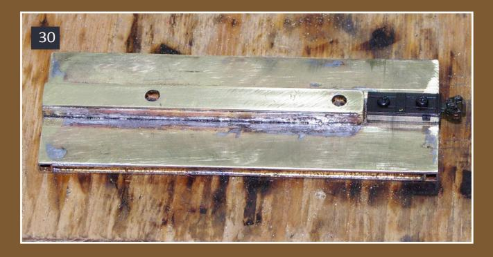
30. I made the center sill with the same dimensions as the scale Accurail Proto coupler box. With most trucks, that puts the coupler at just the right height.
