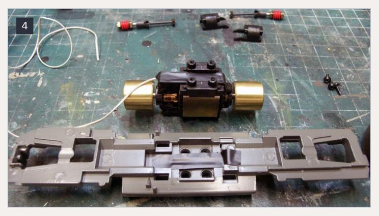
4: Motor and chassis insulated with black electrical tape.
