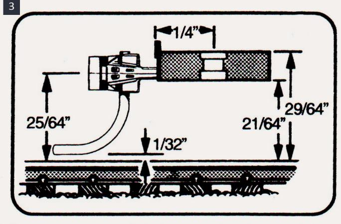
3: Dimensions marked on Kadee's diagram show the proper height of the coupler face and drawbar, and the amount of clearance for the trip pin above the railhead.
