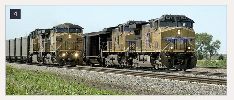
4: Two loaded Union Pacific coal trains, rolling east on the triple track mainline east of North Platte, Neb., clearly show the high-visibility triangular pattern formed by the locomotives' headlights and ditch lights. Photo by Graham Line.
