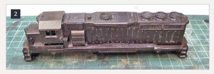
2: The SP GP40-2 shell with paint completely stripped using Castrol Degreaser.
