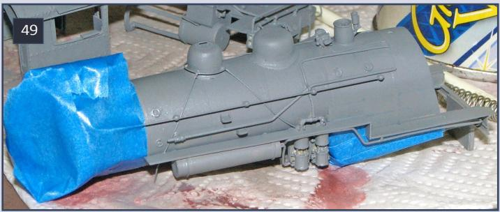
49: Blue painter's masking tape is great for a simple job like this. For the firebox, I trimmed it to fit after burnishing it into place. It is important to get the tape around the handrail as tightly as possible. I think I even slipped little pieces up tape under the handrail as well.
