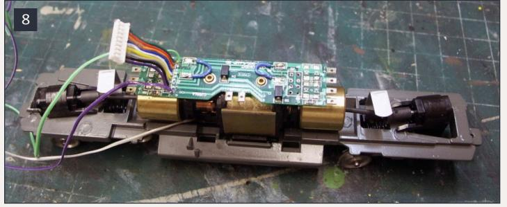
8: The alterations made to the Athearn loco circuit board, including adding a green and purple wire off the green and purple wire pads on the board.
