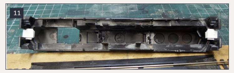
11: Loco shell, with the new styrene coupler pads to allow body-mounting the couplers.
