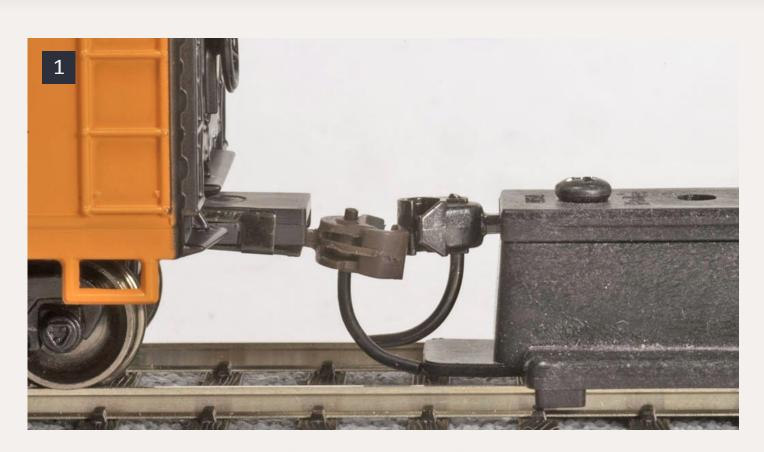
1: Drooping extended draft gear on this refrigerator car lets the trip pin foul the Kadee 206 coupler gauge, even though the coupler knuckle and the trip pin are the correct distance apart.
