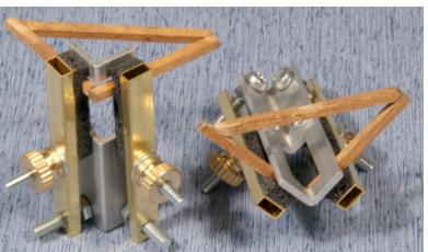
AC-2-2 "Mini Right Clamp"<sub>TM</sub> used for gluing Bulkhead Frames.
