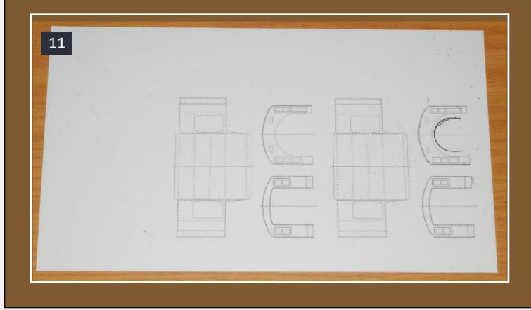
long enough, and smudged some of the lines. Fortunately, I was still able to see them well enough, but if I had to start over, a little alcohol will usually remove the ink for a clean slate. I chose not to seal the ink with a clear coat because I knew I would be gluing to the surface later, and I did not want to interfere with that in any way.
