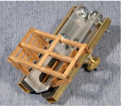
AC-1-1 "Original Right Clamp"<sub>TM</sub> used for Bulkhead Assembly.
