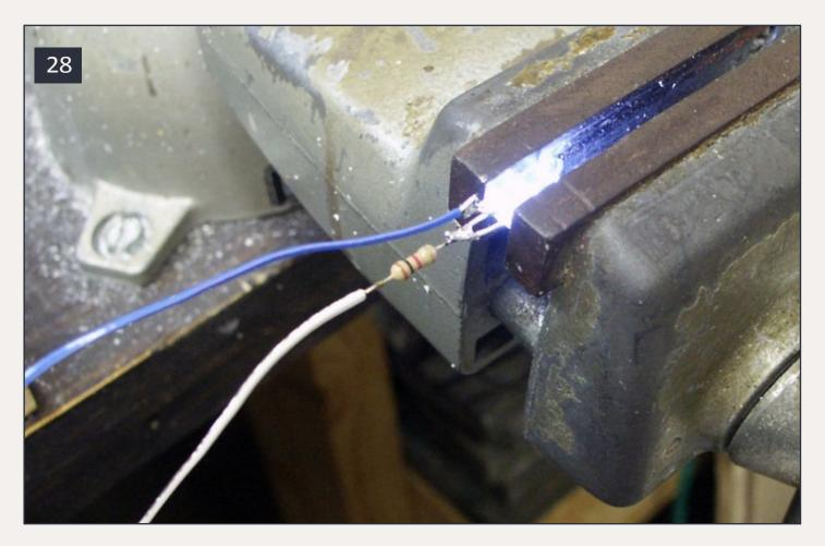
28: Wiring for front headlight LEDs.
