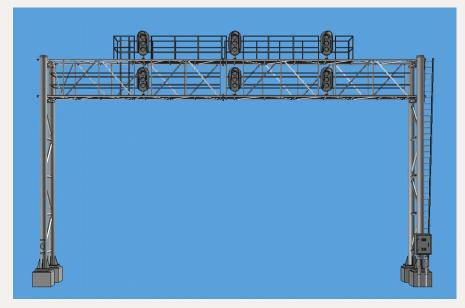
Here is an engineering drawing of a modern three-track signal bridge under development by **BLMA** (blma.com). The assembled HO bridge will be fully operational with six lighted signal heads – that's a total of 18 separate micro LEDs. The bridge legs are on 62' centers (8.55" in HO). The bridge is constructed of injection molded plastic with
