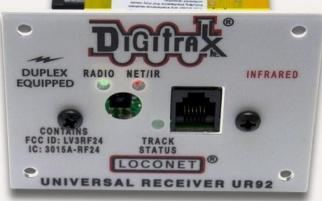
10: UR92 radio transceiver from Digitrax – photo courtesy of Digitrax.
