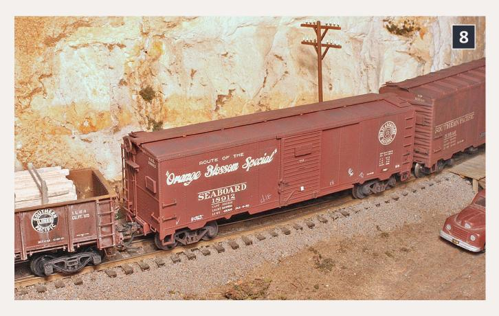
8: This model portrays the Seaboard's version of the 1932 ARA all-steel boxcar. The car carries the road's "Orange Blossom Special" lettering and the plain railroad medallion. It is a repainted Atlas styrene model with decal lettering, an Ajax brake wheel, and a replacement wood running board.
