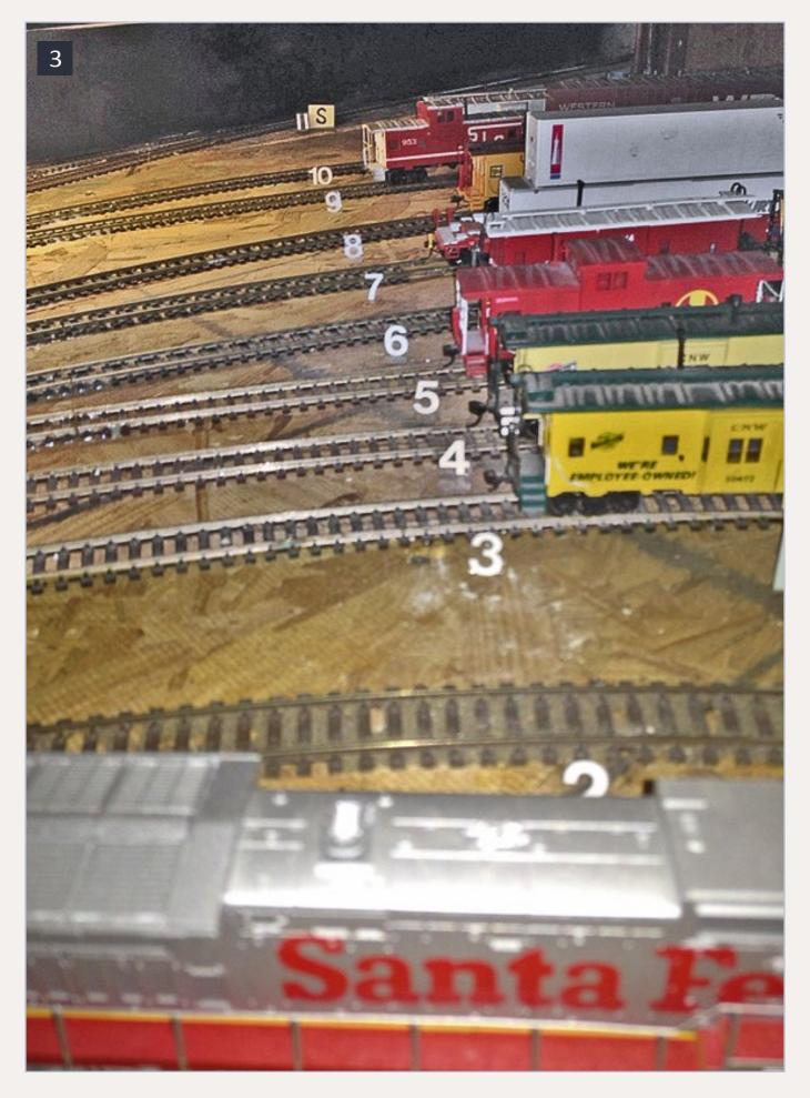
3. Labels cut from plastic packaging provide durable identifiers for staging tracks.
