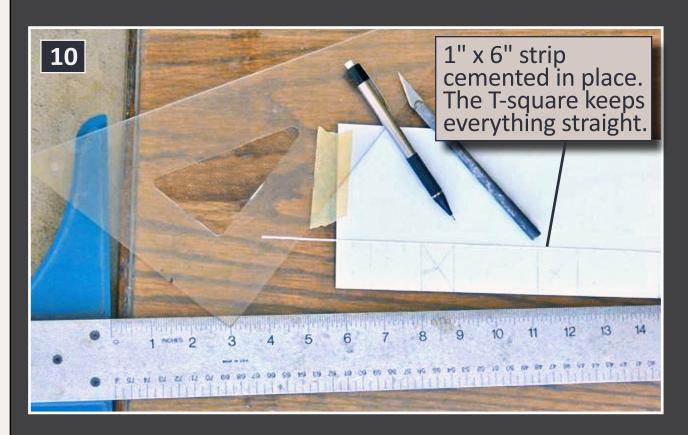
10: Now it is time to begin adding the details. I added the 1" x 6" strip across the top of the 9' – 3" car sides. Using the T-square I made sure that the 1" x 6" is straight and parallel with the bottom of the car. If it's not it will be visually noticeable.
