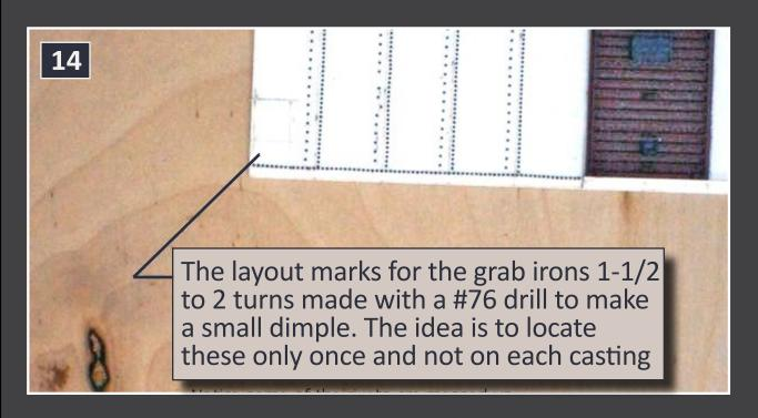
14: I will be making castings of the sides, so I took the time to layout where the grab irons will go. I use Detail Associates freight car grab irons part #229-6209. I began by marking the lower grab iron location up 2'-2" from the bottom of the car side. This will be where the top part of the bracket will be mounted. The second bracket was located 4'-2" up from the bottom of the car. I drew horizontal lines on the sides of the car.
