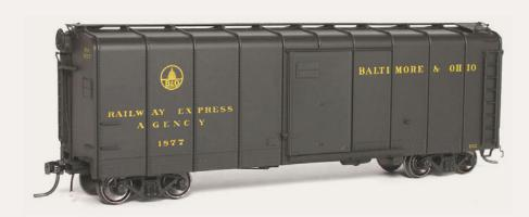
The HO scale ready-to-run model comes with Kadee® #58 couplers, and 50-ton Barber S-2 solid bearing
