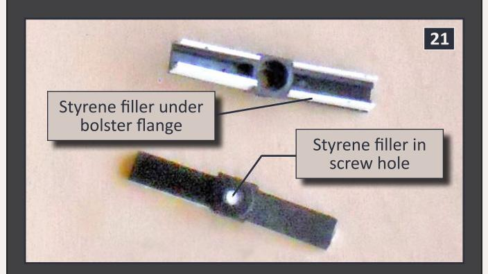
21: Since I did not want to attempt to scratchbuild the bolsters I attacked one of several old Athearn blue box kits (again) that I have laying around. The bolsters were separated from the frame and the area under the flange was filled in to make a smooth side. Since this will be one of the deepest parts of the mold undercuts are a major no – no.
