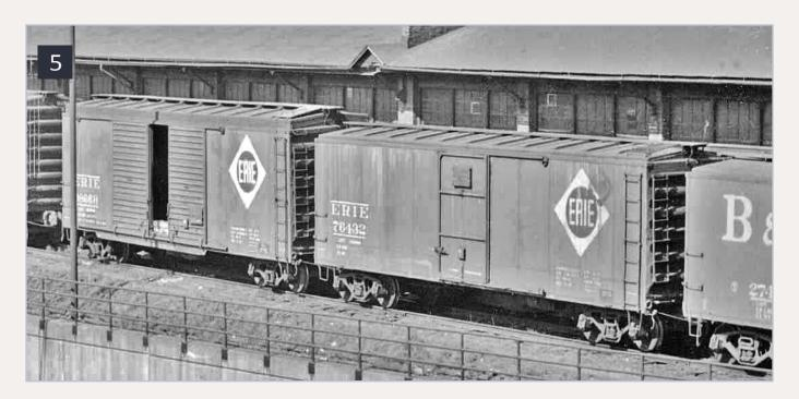
5. Erie 76432 at Akron, OH in April 1959. Note that the original door has been replaced with a Superior door. The car has been repainted at some point in time, most likely when the sides of the car were repaired. The small diamond has been replaced with the larger Erie diamond, however the small Erie Diamond can be seen ghosting through the new paint. (Authors collection and used with permission of George Elwood Fallen Flag Railroad Photos.)
