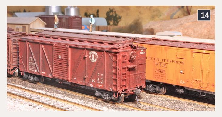
14: Boston & Maine 72597 represents a 40-ton box car, an ARA XM-1 design with plate ends. There were 2000 of these boxcars for this relatively small railroad and they are a good example of a signature freight car. The model was built from a Sunshine resin kit.
