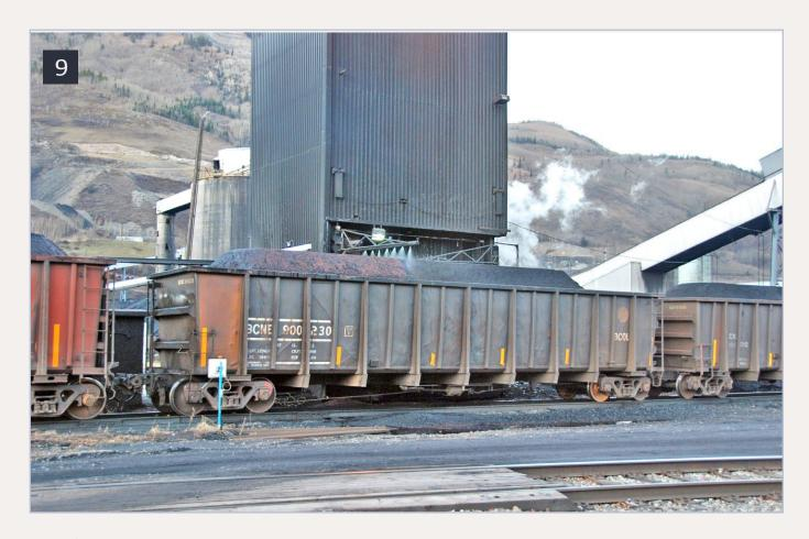
9. Coal load being sprayed with latex to reduce dust.
