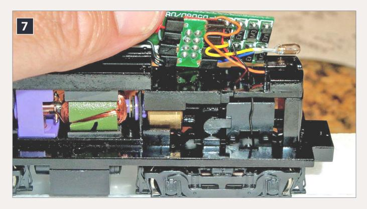
7: Life-Like Proto 2000 S1 (HO-scale) light board and DCC socket.
