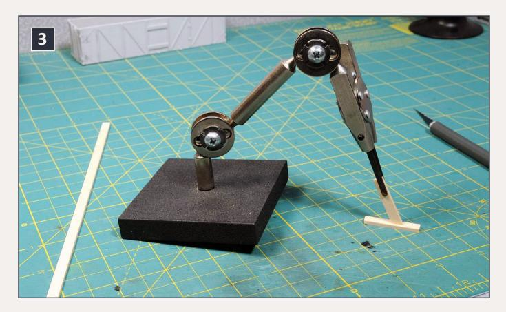
3: Clamping pieces together using a third hand allows you to make sure that they are properly lined up and also hold them together while the glue dries. This "staged" example shows another trick I've used—the clamp is pushed down enough to raise the base slightly off of the workbench. This applies downward pressure on the pieces, insuring a tighter joint.
