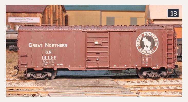
13: This model of a 12-panel Great Northern boxcar, with a diagonal-panel roof, represents thousands of such cars built by and for GN after World War II. It has Pennsylvania Railroad (off-line) reweigh and repacking data from a Sunshine decal set.
