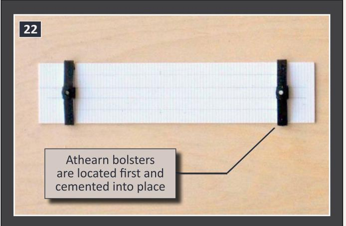
22: After the cement had set I trimmed all of the excess styrene so that it was flush with the bottom of the existing bolster. With that task completed the bolsters were cemented to the floor. The outside face of the bolster is located 3'-9" in from the edge of the floor. When finished the distance between the bolsters should be 30'-4" center to center.
