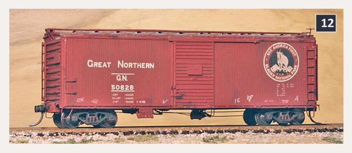
12: The Great Northern chose to build its 1937 AAR standard boxcars with tongue-and-groove wood side sheathing. This Sunshine resin model captures all the details of that distinctive car, along with the "front-facing goat" emblem in use when the car was built in 1937.
