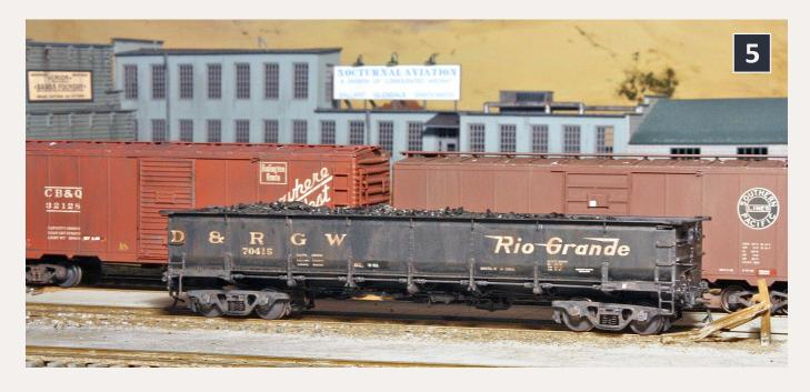
5: The distinctive 46-foot D&RGW gondola fleet, all drop-bottom or GS cars, is represented by this brass model from W&R Enterprises. The correct clasp-brake trucks with outside brake hangers were provided with the car. The cars were predominantly used in coal service, and Southern Pacific received Utah and Colorado coal in cars like these for domestic stove use in depots, section dwellings, cabooses, and so on.
