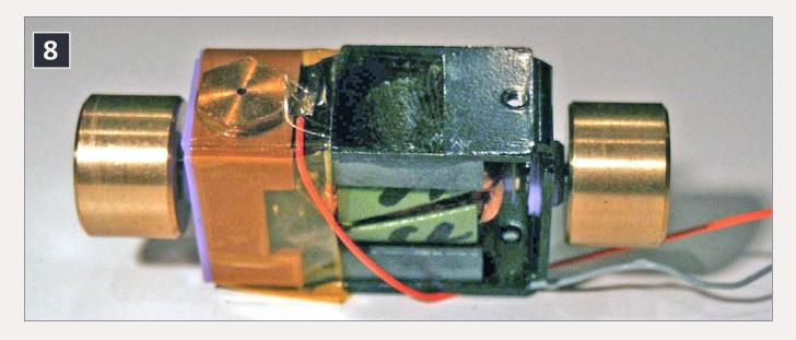
8: Life-Like Proto 2000 S1 (HO-scale) motor after insulation – bottom view.
