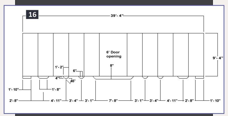
16: Tab spacing diagram drawn to assist with the construction and location of the tabs.
