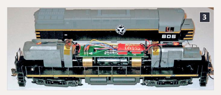
3: Digitrax DN163PS decoder installed in an Atlas C424.
