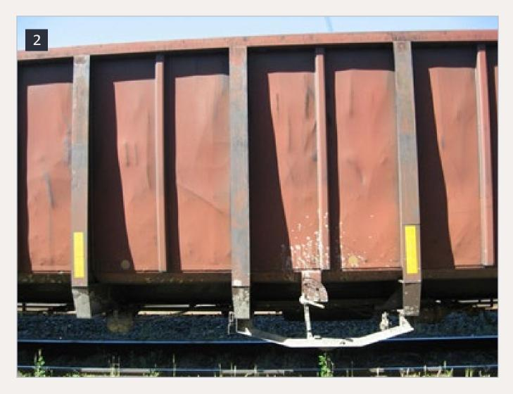
2. Load-empty feature - Newer cars had the same feature that was mechanically-applied when the car was loaded. Norman Skretting photo.
