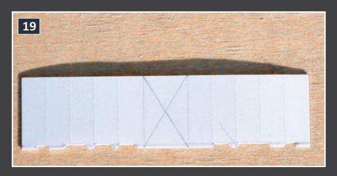
19: The tabs have been placed on the cars sides. The top master is complete with the lower master needing some additional work. The X marks the location of the door. The doors and the top guide rails are yet to be installed.
