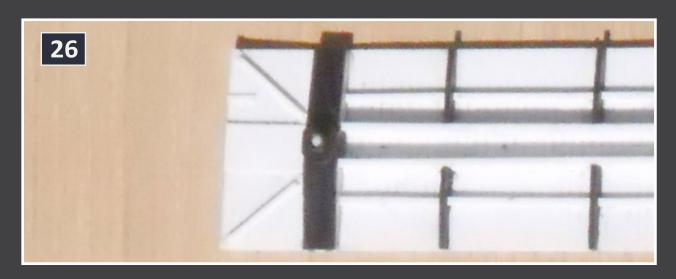
26: Finally, if you noticed in previous photos there are lines drawn at the ends of the car from the centerline to the corners of the cars, these were located incorrectly. What I ended up doing was to cut 8 pieces of 1" x 3" stock with a 45° bevel on one end.
