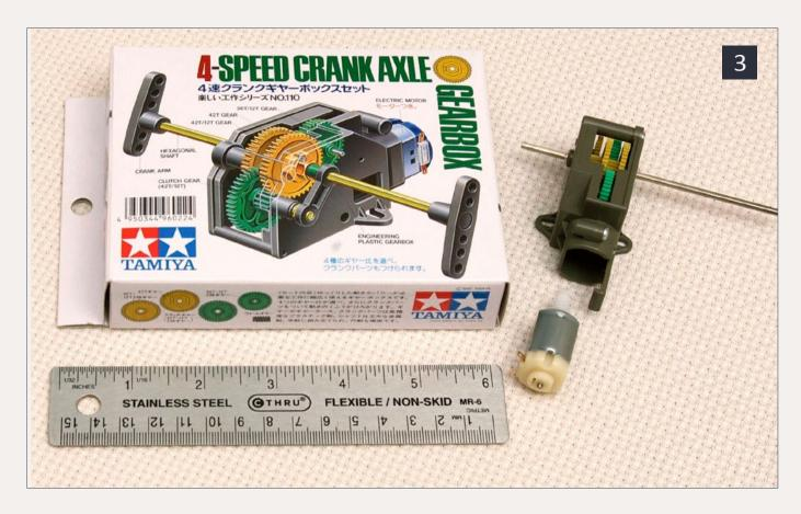
3: The Tamiya 4-speed gearbox that is the heart of the working conveyor.
