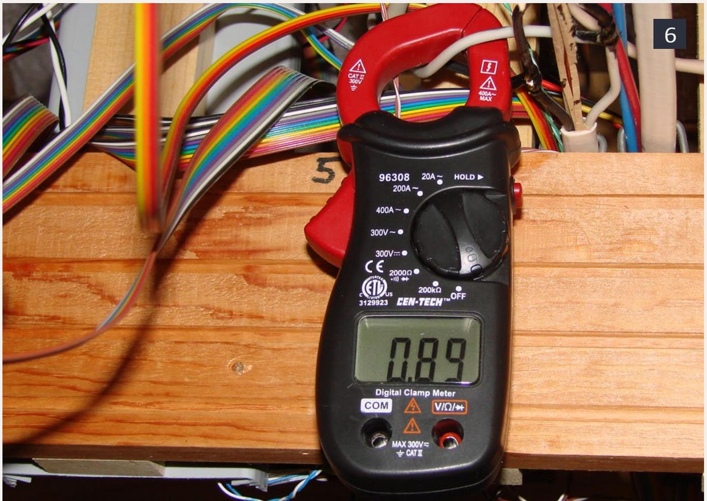
**6: At this point we discover that the short circuit current is flowing in the branch feeder. Even in cramped spaces, it is easy to follow the short circuit current without disconnecting any wiring.**
