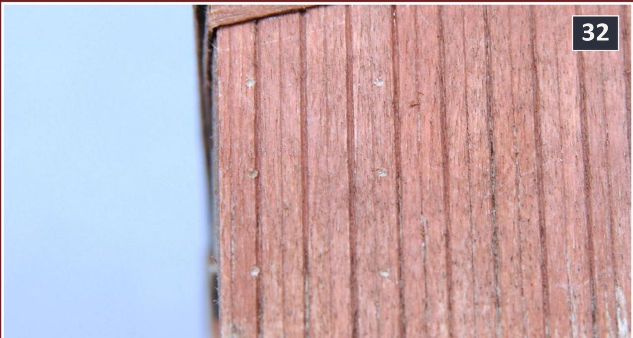
32: Lightly twist a #78 drill and lightly drill at each hole in the template, drill just enough to mark the surface of the sheathing. After removing the template, find your marks and drill the holes to depth.
