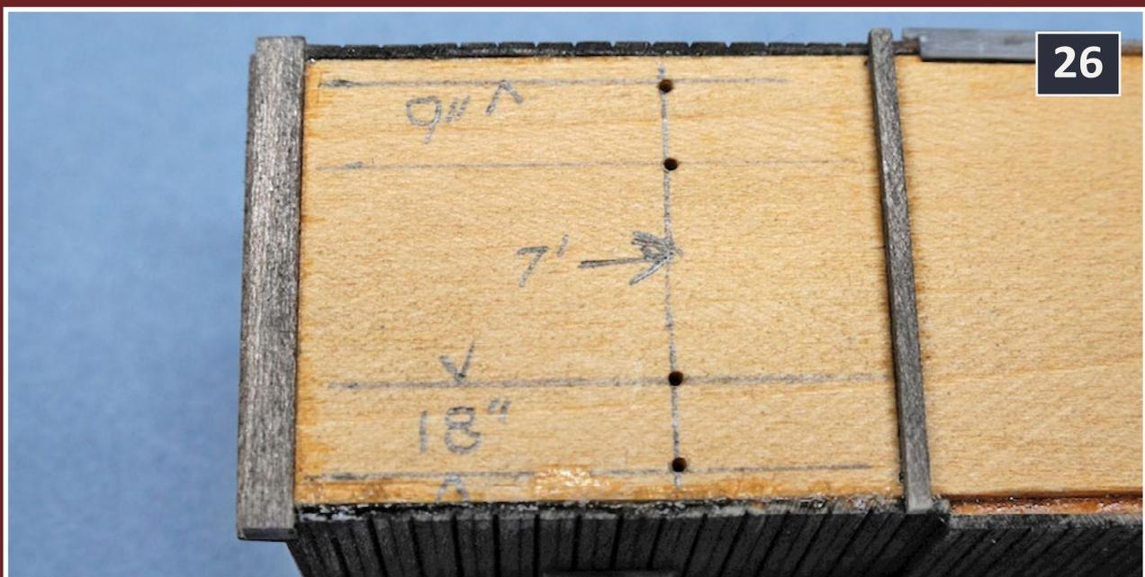
26: Use the dimensions indicated and drill four holes on each end of the underbody for the truss rods. Thread nylon fish line through the holes and over the needle beams. Glue them in place.
