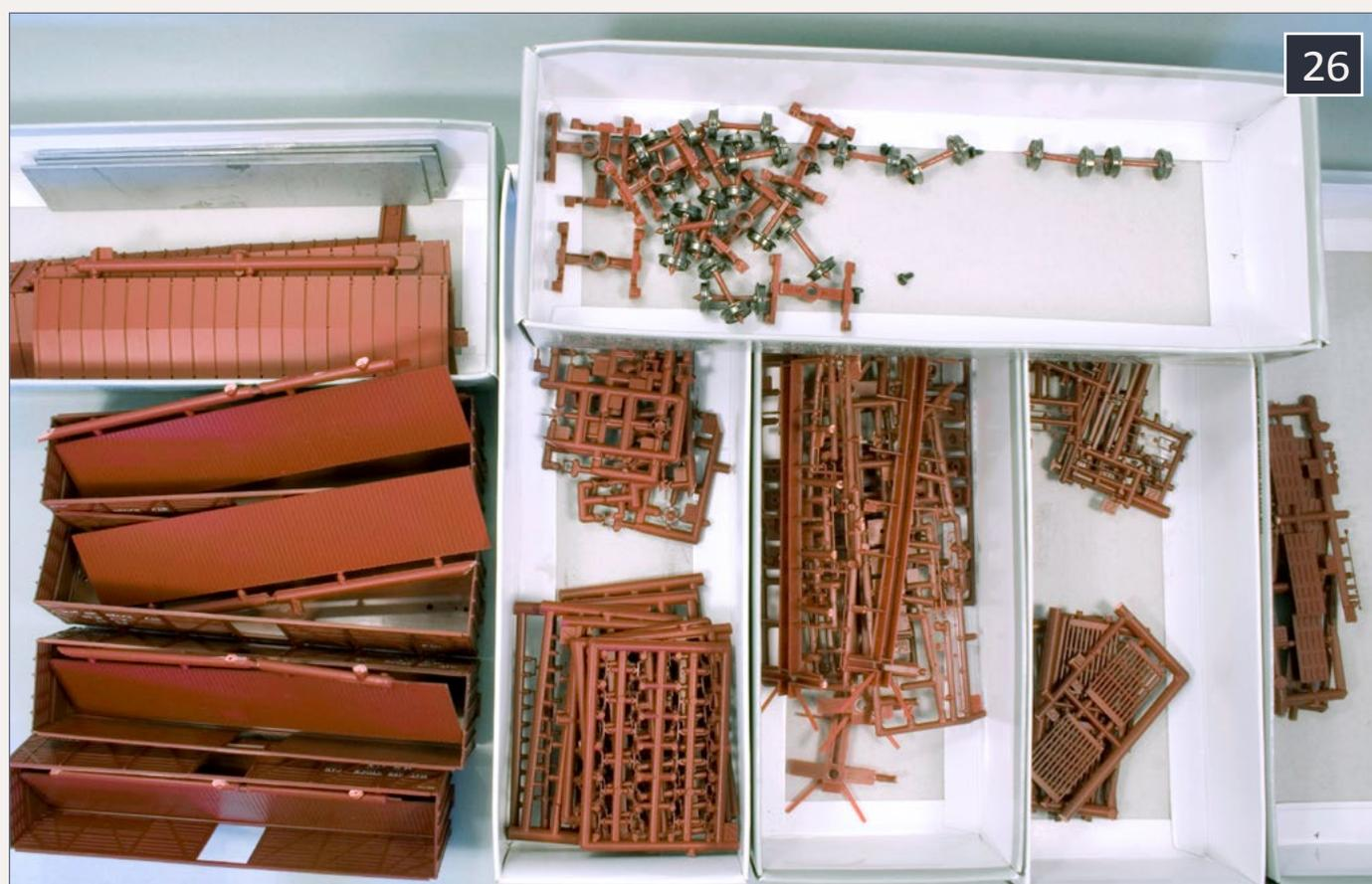
**26-27: All of the parts for our stock car build are sorted into boxes. Kit boxes work well for this. The photo on the right shows the sort for a build of 12 refrigerator cars – notice that the car ends with the reporting marks and car numbers are kept with the corresponding car body.**
