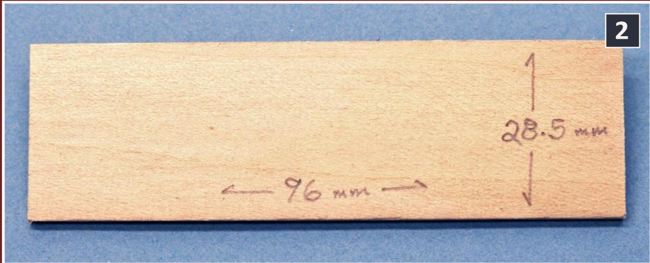
2: Cut a floor to the dimensions shown from 1/8" thick basswood. These dimensions account for the thickness of the sheathing material. I find that my accuracy in constructing models is greatly enhanced by the use of a dial caliper. My caliper is calibrated in millimeters, and I will give measurements in that system. For me it is more precise to measure 10mm on a caliper versus 2'-10" on a scale ruler.
