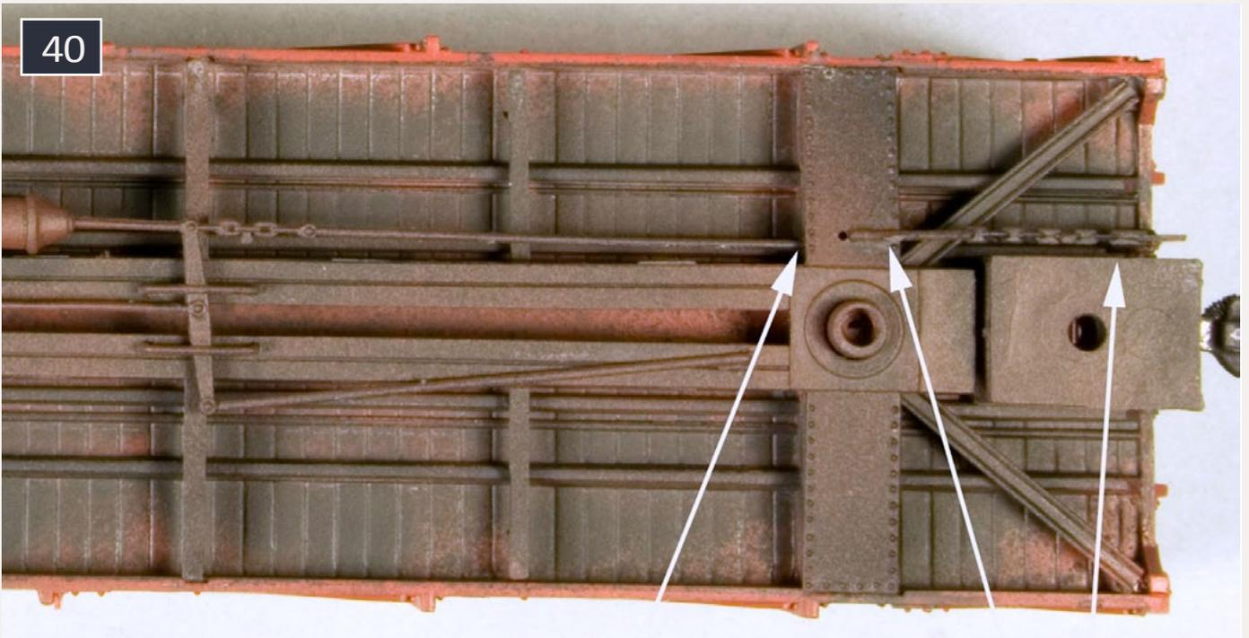
**40:** Arrows show where the brake rigging was cut and tucked under the body bolster frame to keep it from interfering with the truck swing, and seating on the frame. The chain assembly was removed between the two arrows on the right for the same reason.
