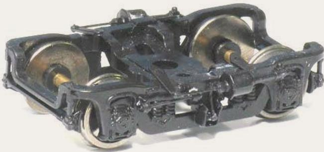
A popular four-wheel passenger truck with inside-swing hangers was General Steel Casting's model 41-N-11 (above). Rapido's HO scale version, item 102012,
