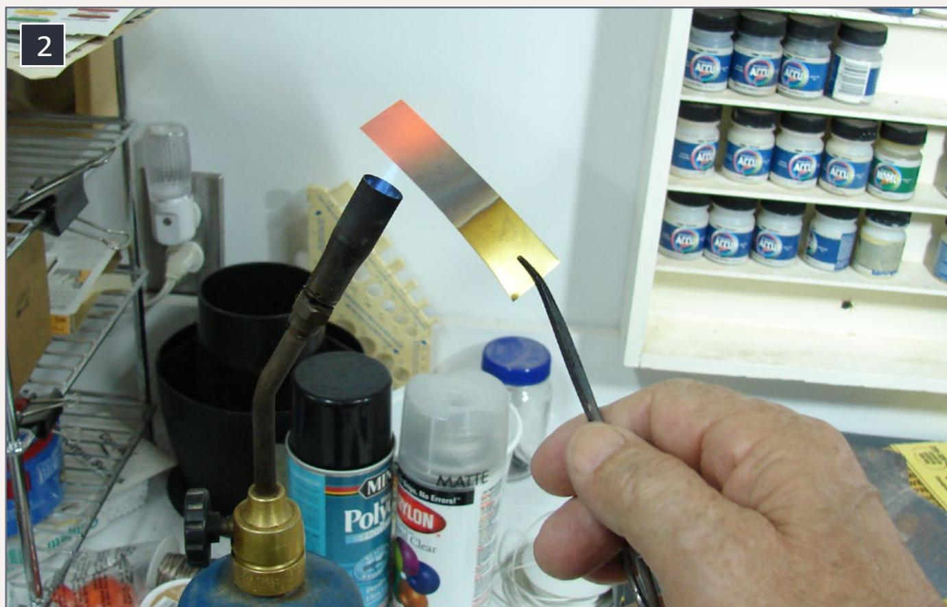
**2. The brass is heated with a plumber's torch, near a bowl of water to quench the brass, to make it very soft.**
