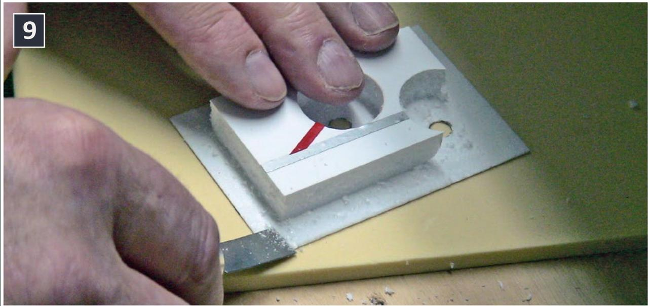
Using a 1/2"-wide flat X-Acto blade, carefully scrape the filler off the veneer to allow the panel to set flat on the fascia.
