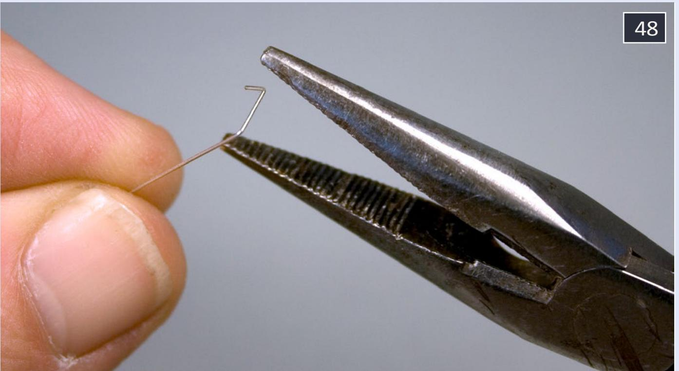
**48: Pliers may also be used to form grabirons. Experiment with the placement of the wire on the jaw until you get the desired size. Mark the spot to produce consistently sized grabs.**
