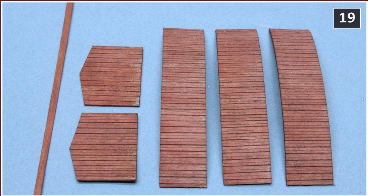
19: This figure shows, from left to right, a scale 1x6 that will be used as a fascia strip, the car ends, and the roof sections. The roof pieces are 17mm wide, and will be trimmed to fit later in assembly.
