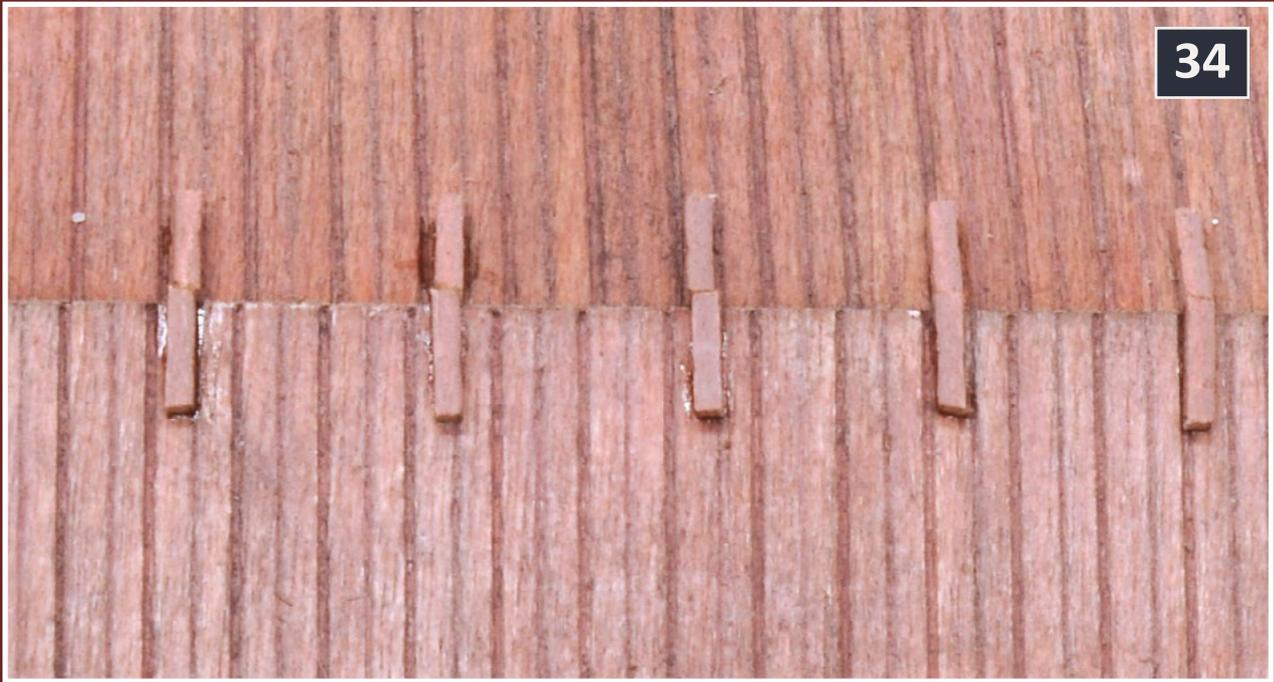
**34:** Add the running board supports. They are made from scale 2x4 stripwood cut into 12" lengths. Each pair is spaced 24" apart; the 2" dimension is bonded to the roof. Omit the supports directly above the windows; this is where the stove stack will exit the roof.
