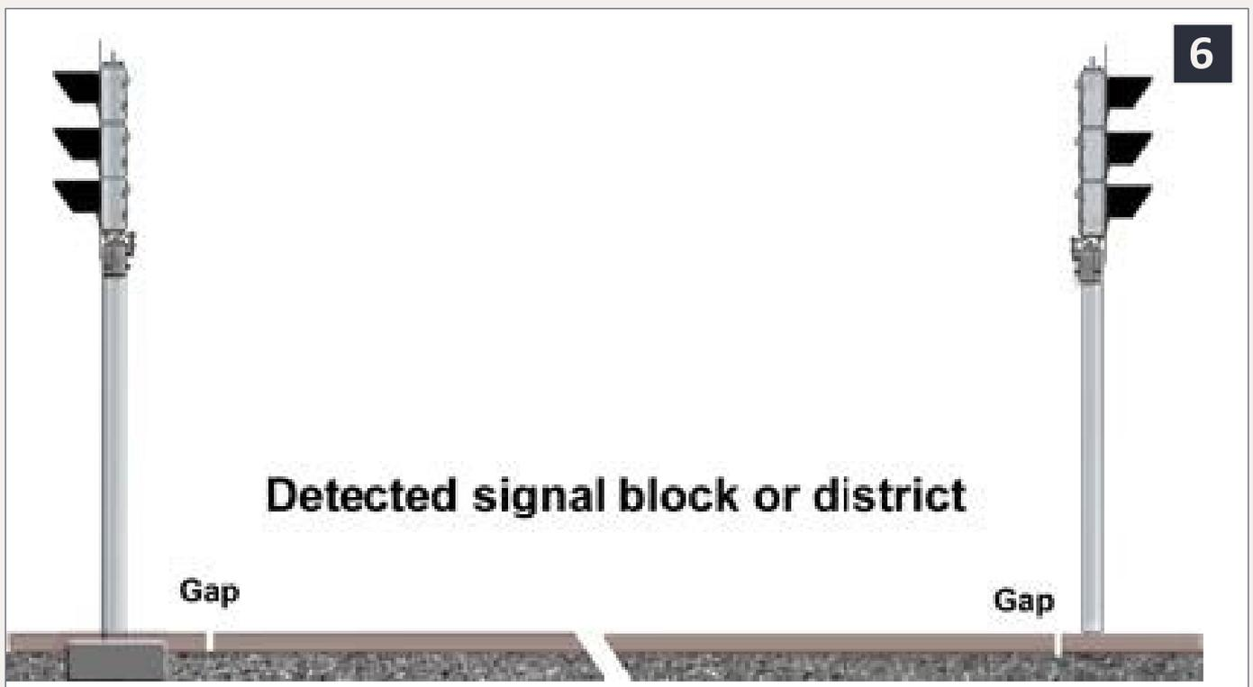
**6: Drawing of a detected track block with signals outside each end. The split in the middle represents the missing portion of a long block. If DCC detection is used, gaps will be needed just inside the signals.**
