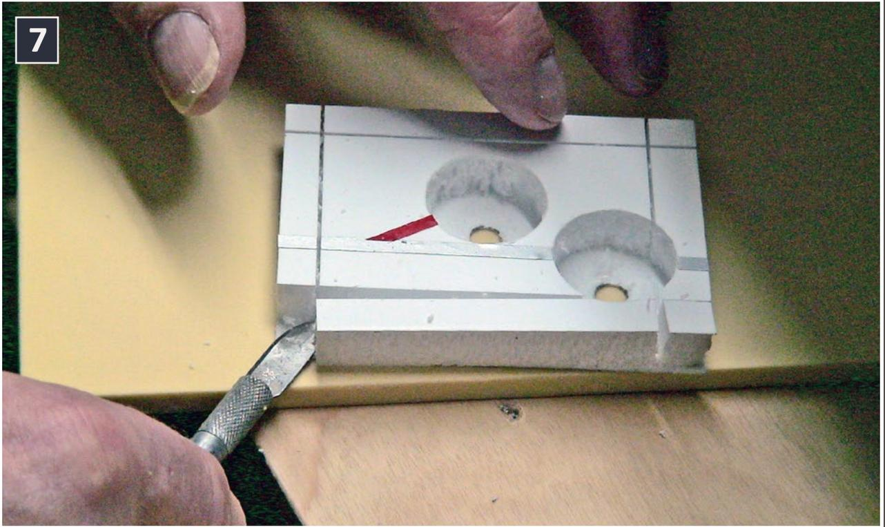
Using an X-Acto knife, I carefully cut the filler from the veneer. Note the placement of my left hand.
