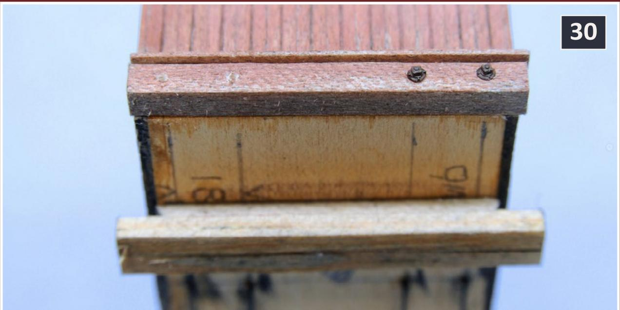
30: Drill #72 holes in the middle of the end sill, aligned with the truss rods. Add Grandt 5093 NBW castings. Paint them black.
