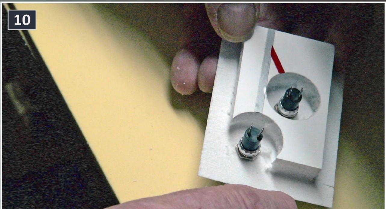
Finished panel ready for mounting. If making a panel for flush-mounted switches, increase the size accordingly so holes do not get cut, as in this picture.
