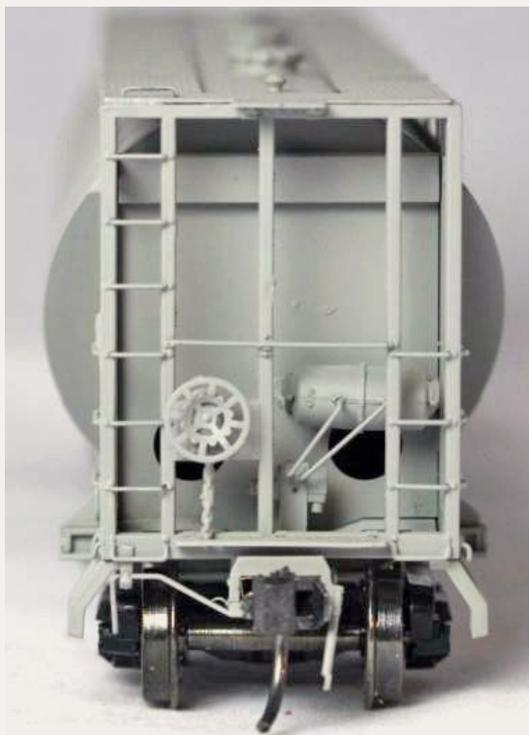
Additional options include three different ends, two styles of etched metal roofwalks and three different gauge housings. The HO scale ready-to-run model features wire grabs, and Kadee® couplers with screw-in coupler pocket covers. The MSRP is \$54.95. Visit the above website for a complete listing of variations available for each road name.
