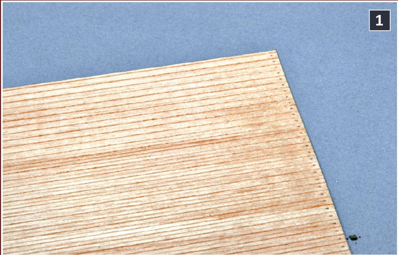
1: In reviewing photos of 19th century boxcars, I observed that quite a few had milled shadow lines in the cars' sheathing. There appeared to be one or two shadow lines present in each board. To create single shadow lines, mark the centers of the  $3/32$ " scribes. Use a steel scribe and impress a new groove between the manufactured ones. Use moderate pressure on the scribe, as this new shadow line should not be as deep as the manufactured grooves.
