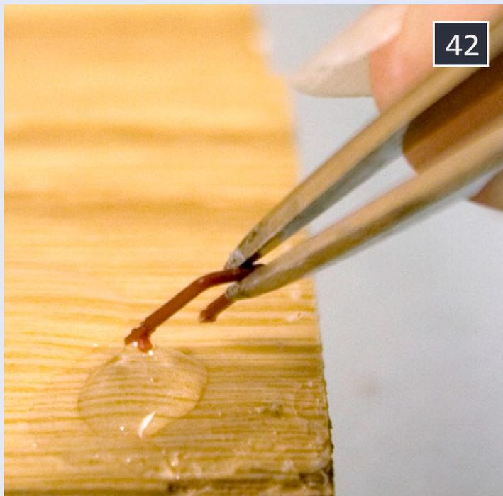
**42:** The part is dipped in the glue on the area that will attach to the model. I usually touch the part to a paper towel before attaching, to get rid of any excess glue.
