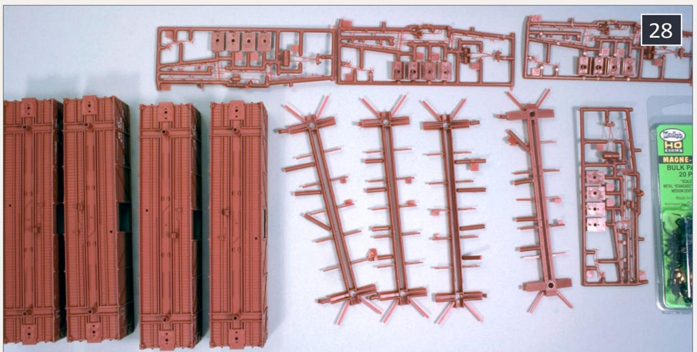
**28: Here are all the parts on the left for the underbody, while on the right are all of the cut parts.**
