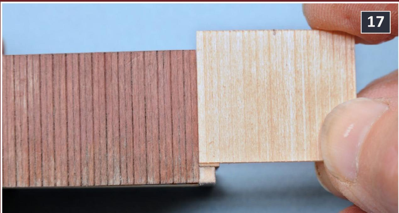
17: Using the side sheathing for the ends creates a roof peak one foot above the eave. Mark the eave height on both edges of the end. Determine the center of the end, and cut the roof slopes.
