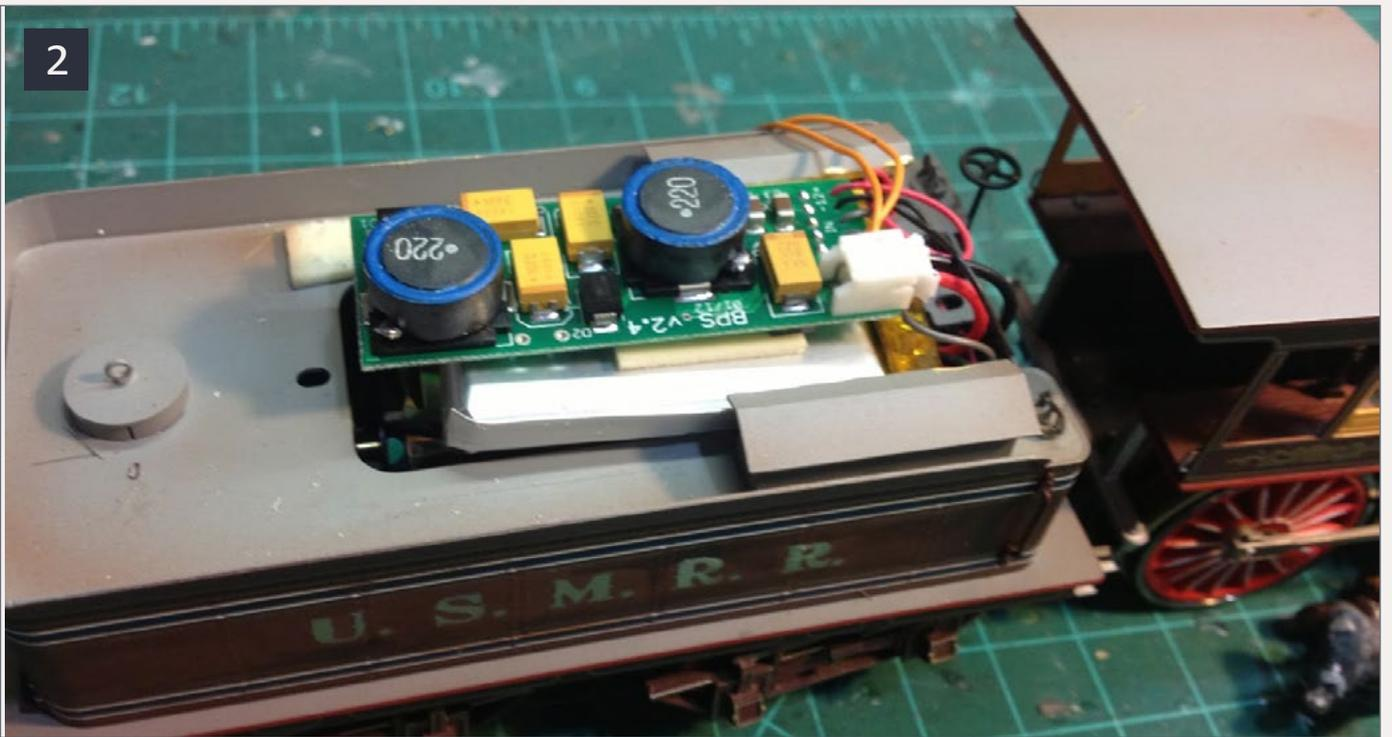
**2: The battery power supply and battery fill most of the space on top of the motor in the tender. It took a full pile of wood to hide it.**
