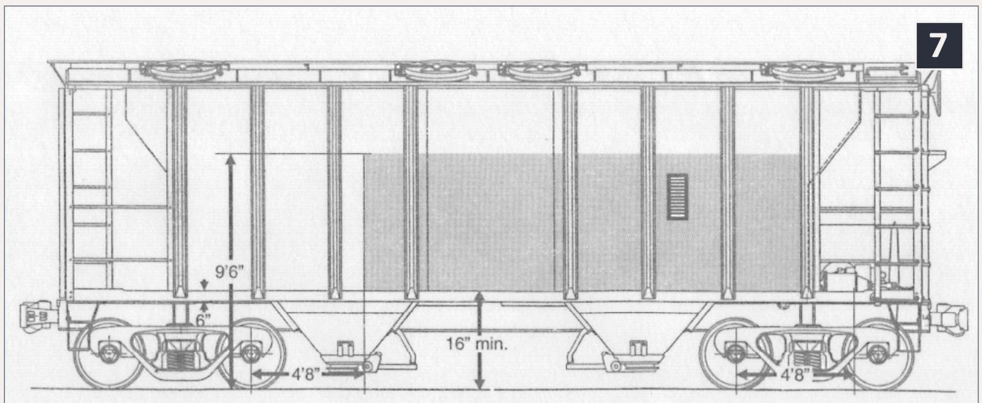
**7: The shaded zone indicates where color-bar ACI labels were to be placed so they could be scanned by a trackside reader. Microscale.**
