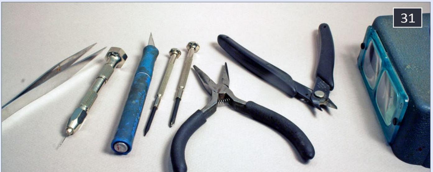
**31: My well-worn tools include tweezers, pin vise, knife, screwdrivers, pliers, sprue nippers, and an Optivisor. There are other items that may be needed, depending on the type of kit you are building.**
