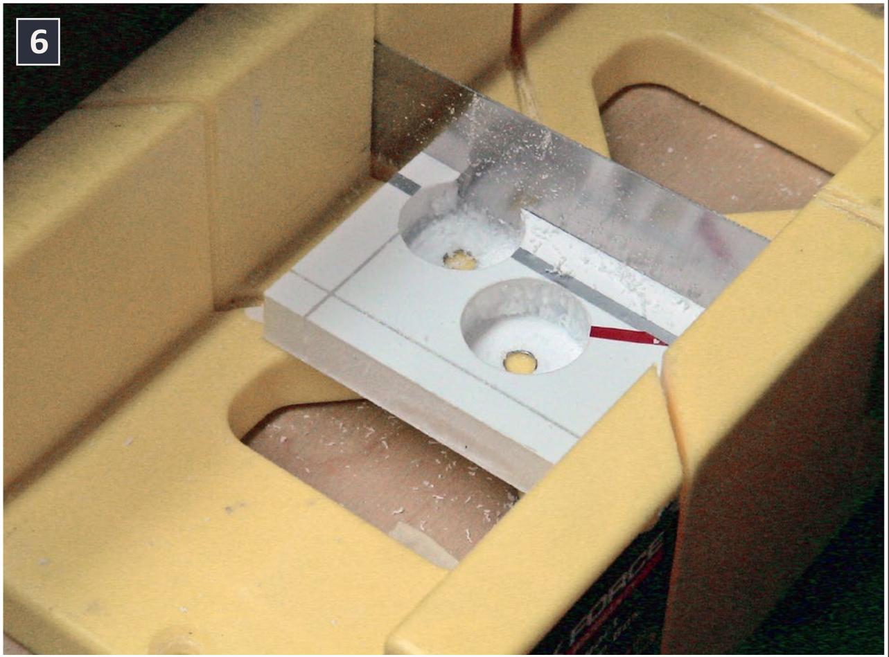
I use a miter box and a fine-toothed pull-saw (my preference for smooth cuts) to cut around all four sides, about 3/8" back, and just down to the front veneer. If you use a light touch, you can cut right to the tough veneer, but not through it.
