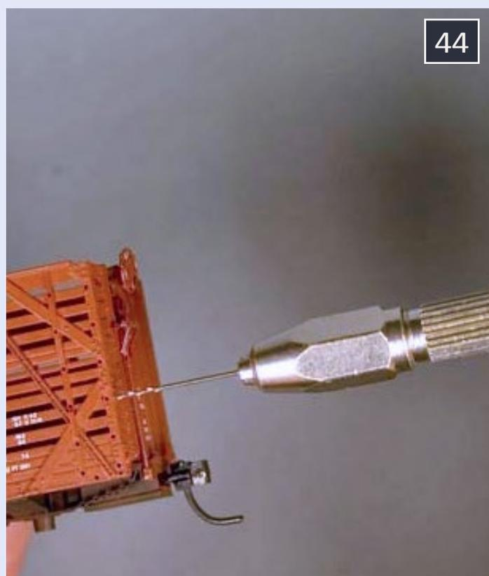
**44: A pin vise with a #76 bit is used to open holes that have been filled with paint by the manufacturer.. Keep the drill perpendicular to the work, and apply light pressure as you drill. You can expect to break some bits regardless of how carefully you use them. I stock up with extras so I won’t be looking for a bit to finish a model on Sunday when the local hobby shop is closed.**
