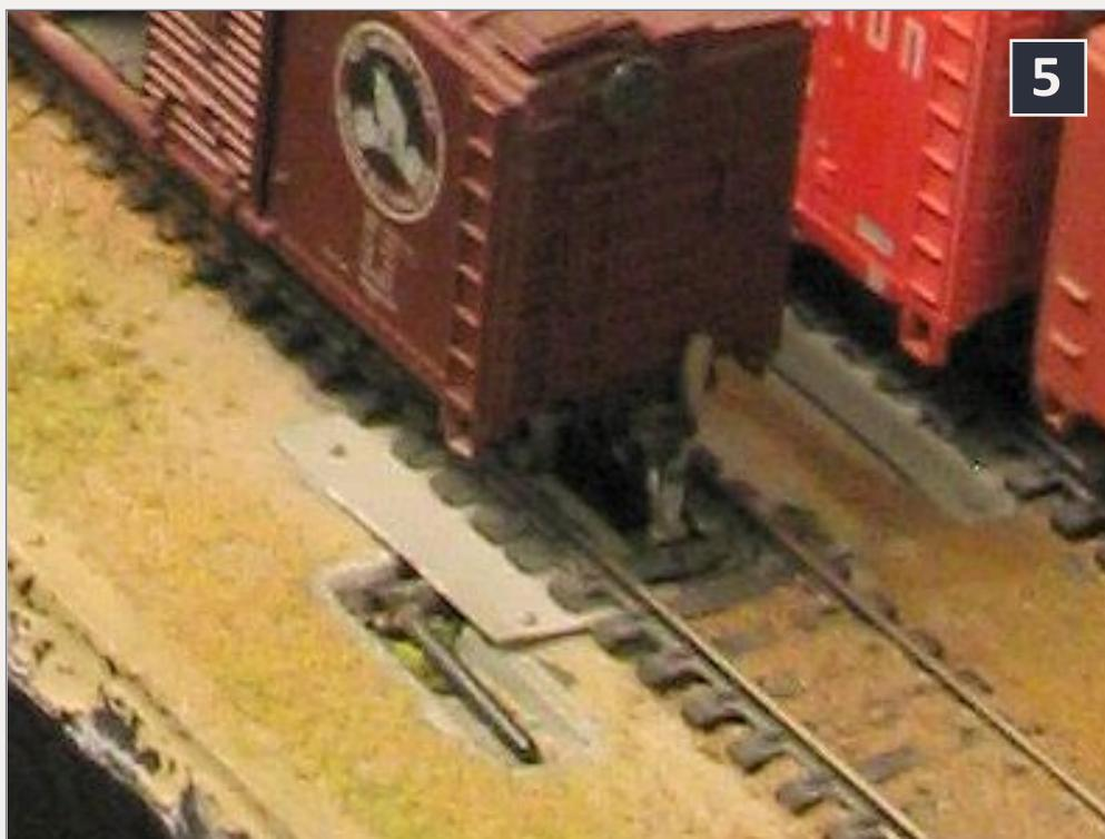
**4-5: A surplus eraser can be trimmed to fit snugly between the rails, holding cars in place until it is removed. Another brake combined two L-shaped wires to create a flip-up car stop. George Booth.**
