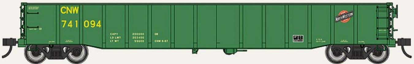
A 53' gondola based on another Thrall prototype is scheduled to be released to dealers this month. The Proto™ series model will be available decorated for ICG/CN, CSX/NYC (ex CR), Green Bay & Western, and CNW as shown here. The HO scale ready-to-run model has an MSRP of \$31.98.
