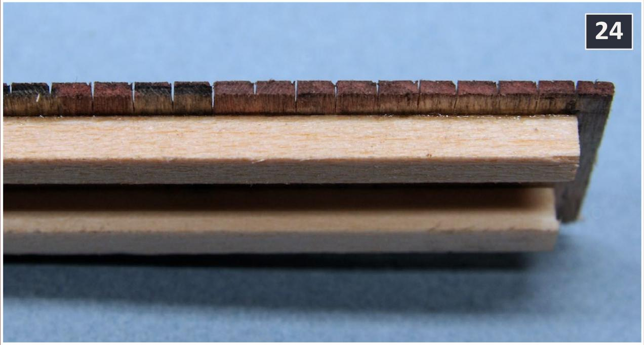
**24:** To enhance the roof eave, use a knife blade to slice into the manufactured scribes. Now create the other roof half.
