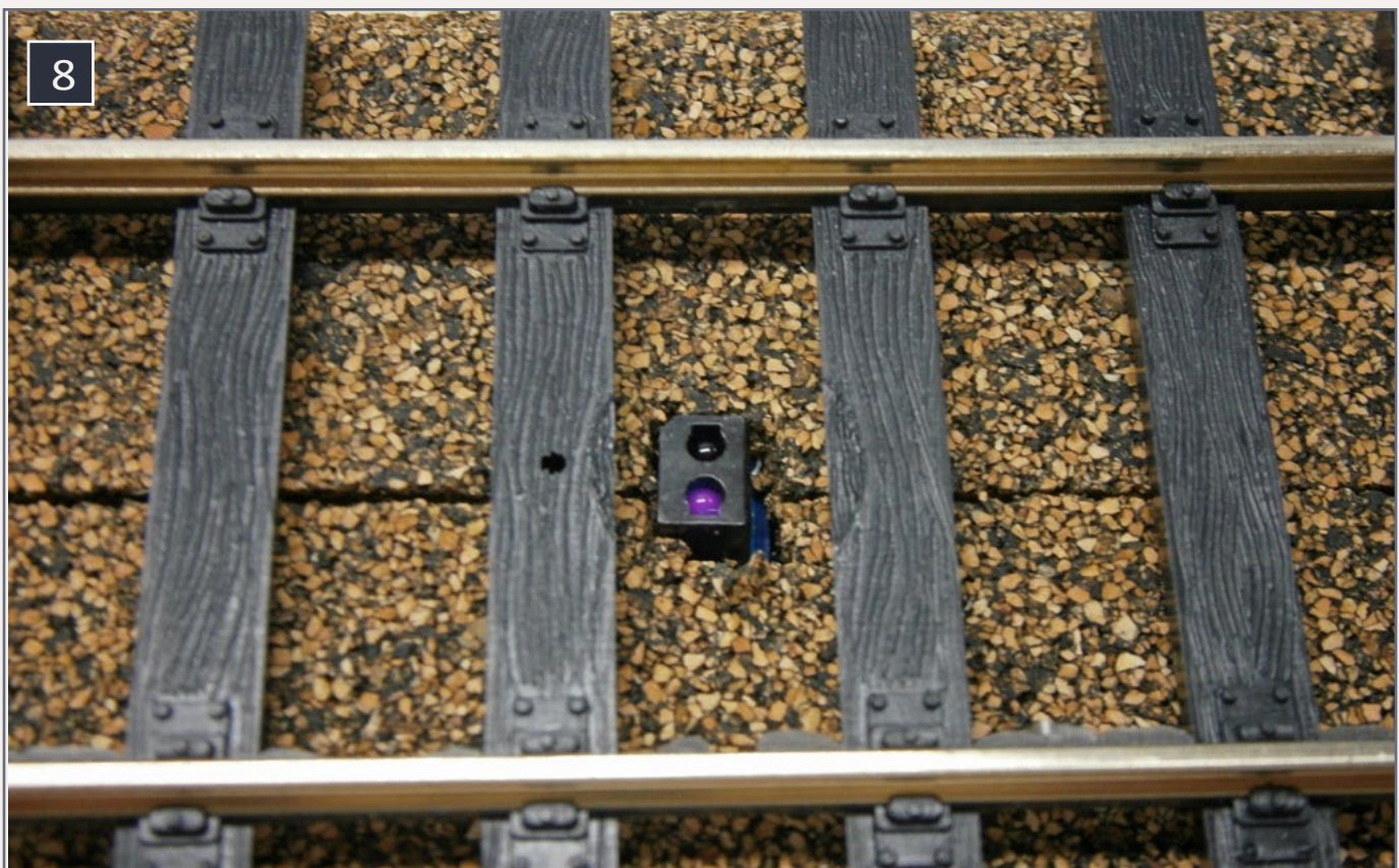
8. The sensor mounted below the track.
