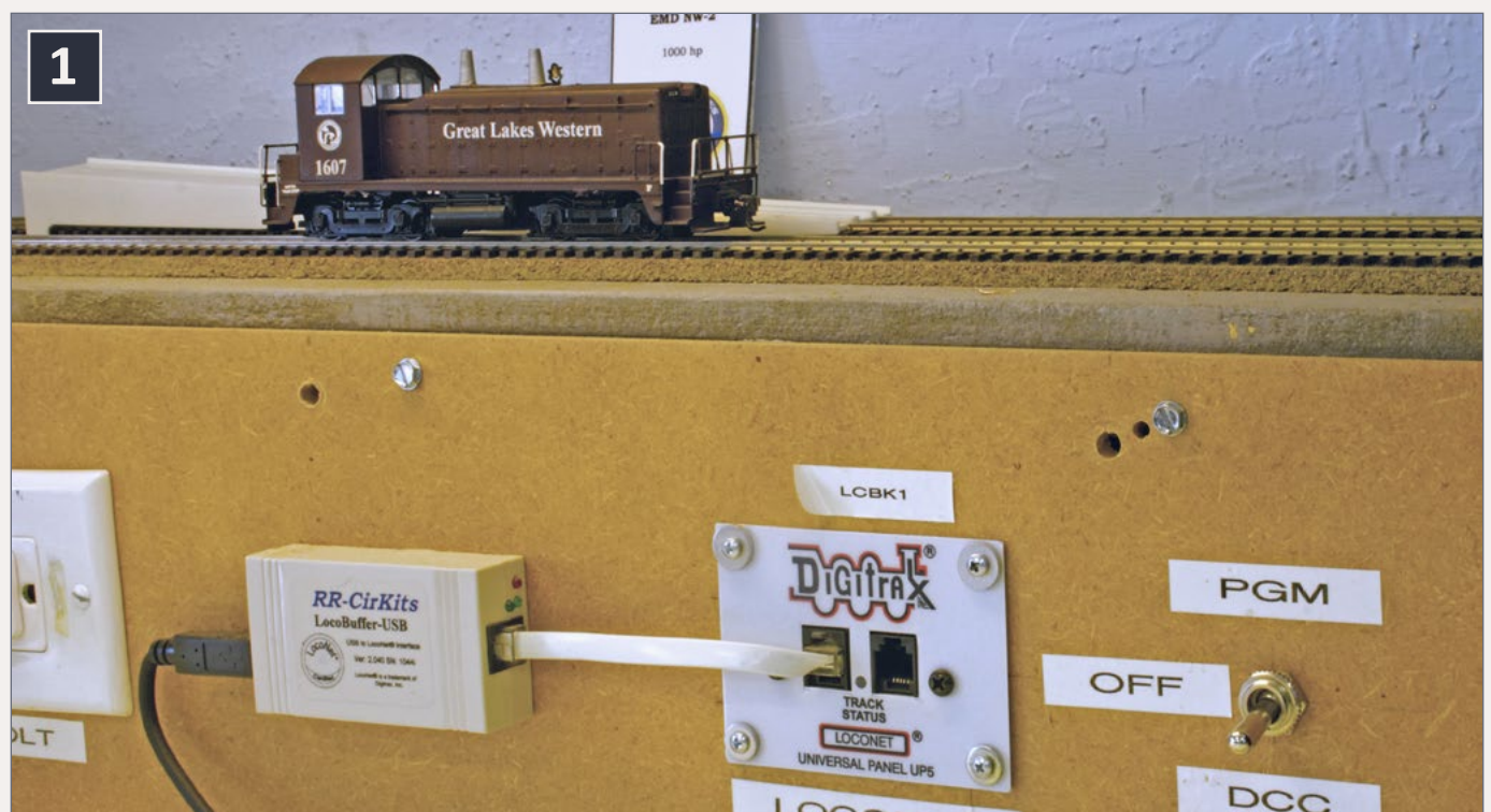
1. The programming track station and selector switch at the PebbleCreek Model Railroad Club.
