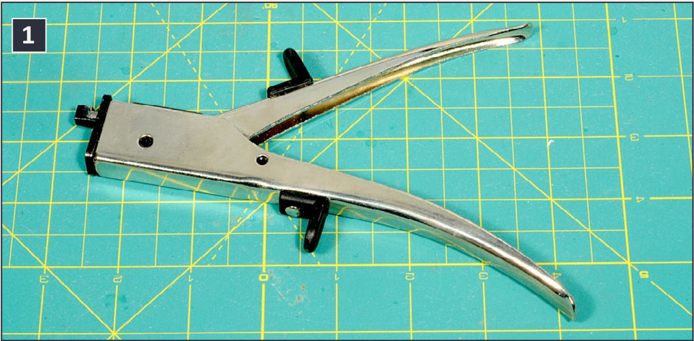
1. This is my nibbler. If purchased from Radio Shack, it is a “nibbling tool” but if purchased from Micro-Mark it is a “nibbling cutter.” They appear to be identical.
