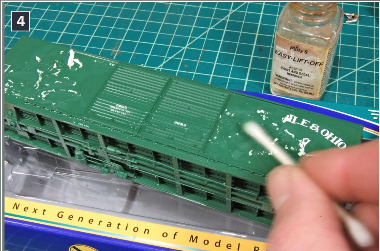
4. Polly S Easy Lift Off decal and paint remover takes away the factory lettering. Since Polly S Easy Lift Off may be hard to find, another option is to soften the lettering with a piece of paper towel that is soaked with 91% rubbing alcohol place on the car side for about 10 minutes.
