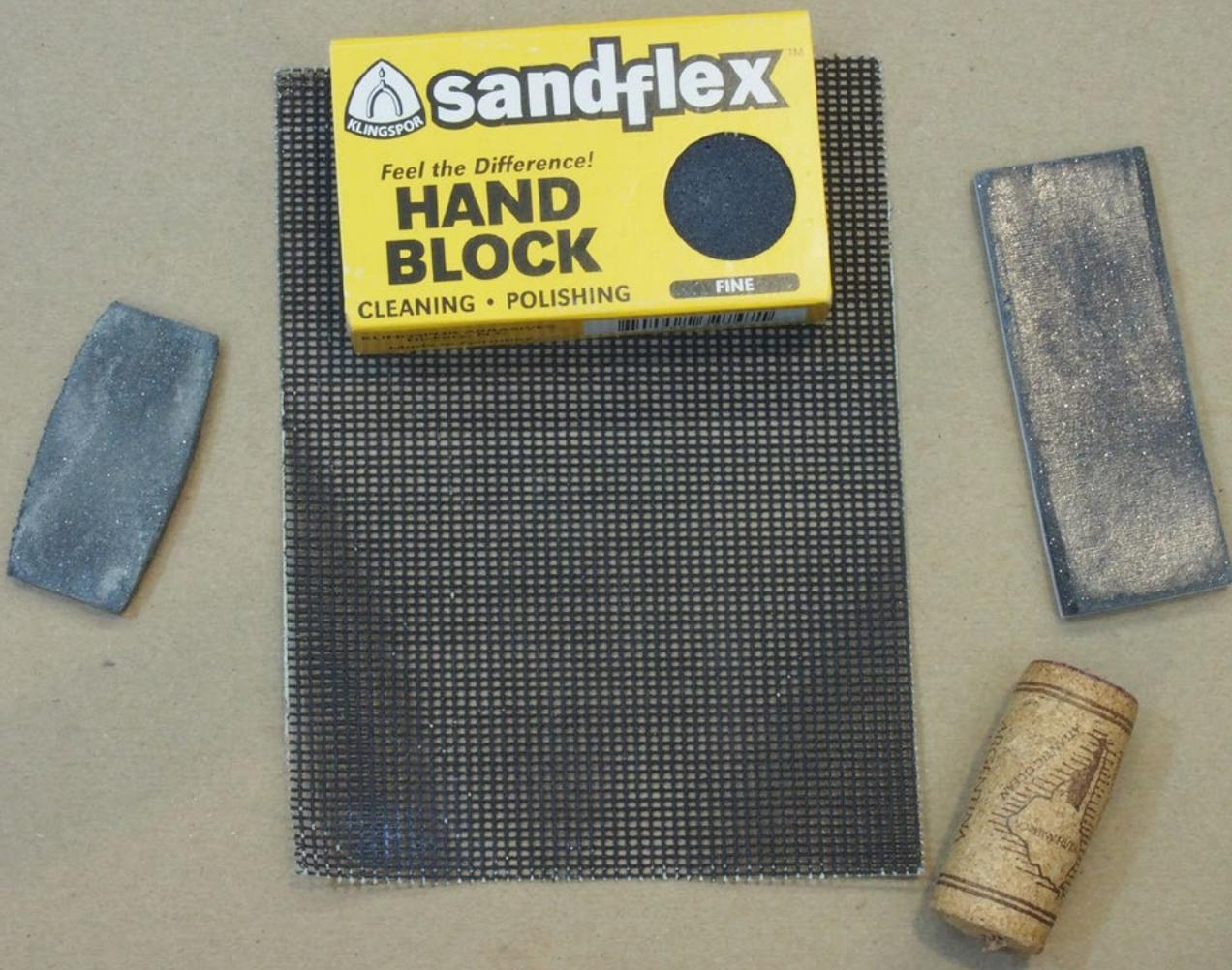
**2. A number of abrasive cleaners: PECO track eraser, rubber sanding block, Scenic Express eraser, fine mesh drywall sandpaper, and a cork.**
