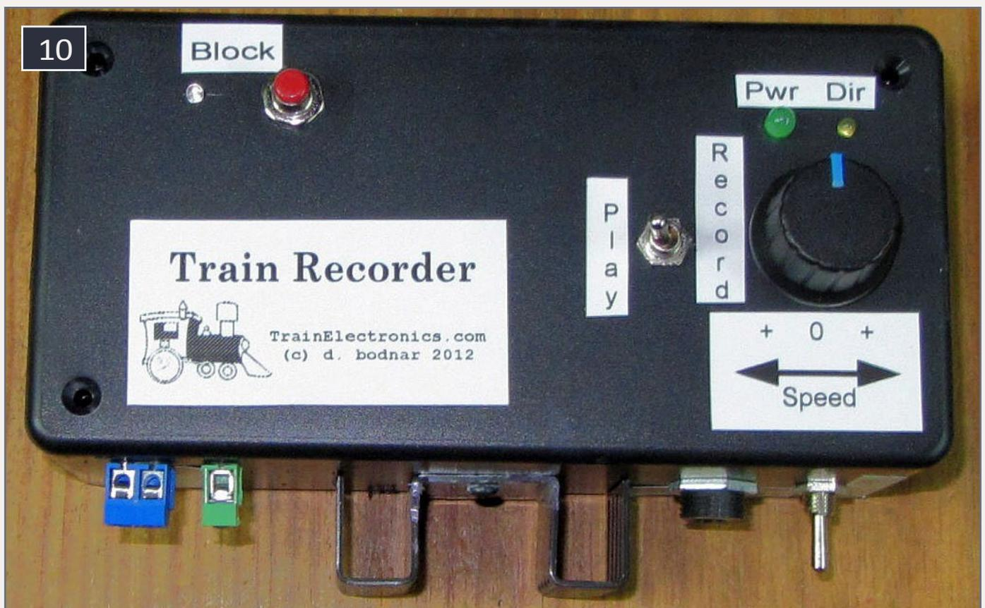
10. This is yet another unit with simplified controls. Speed is adjusted with the knob on the right. The larger green LED shows the power level, and the smaller LED next to it indicates direction. The Play/Record switch is to the left of the speed control. The LED and switch in the upper-left are for the block sync relay. When the relay is active and the block is unpowered, the LED is lit.
