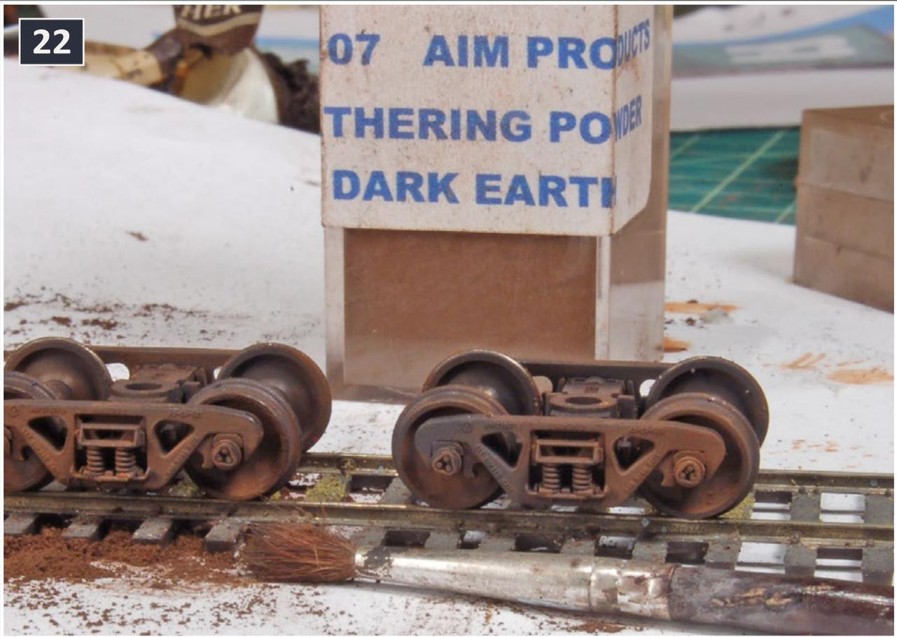
22. Kato 601 roller-bearing trucks, airbrushed with Floquil Grimy Black and finished with AIM Dark Earth weathering powder.
