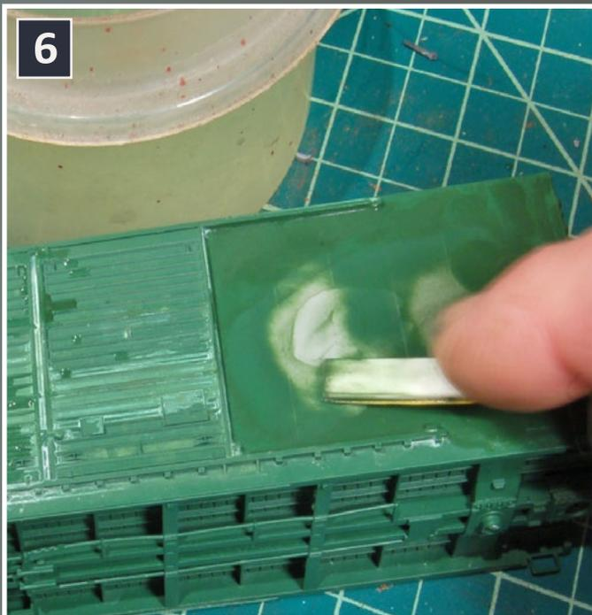
6. Remove the cast-on weld seams using 400 and 600 grit wet-dry paper.
