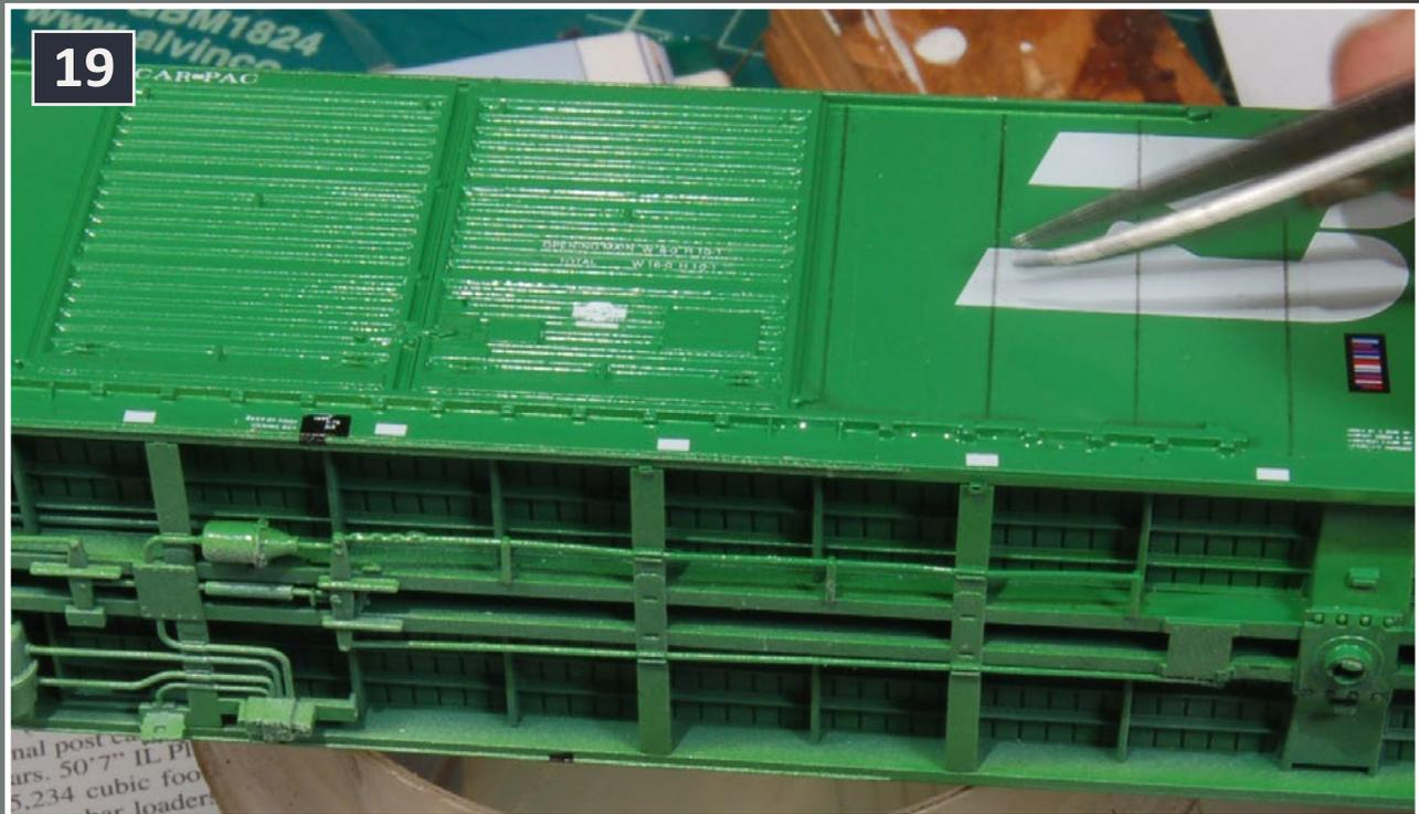
19. Fine-tune and adjust the seams before applying decal solution.
