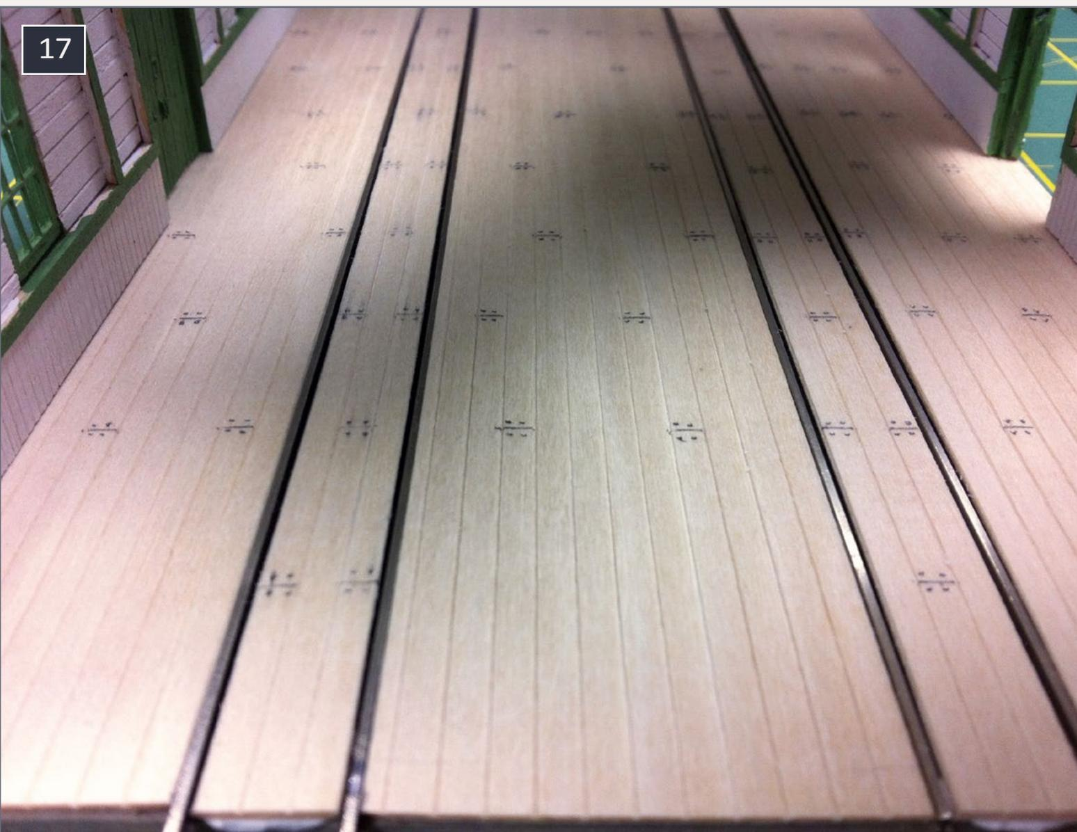
**17. I laid out the individual boards and punched nail heads into them. Now to stain the floor and give it that well used look.**
