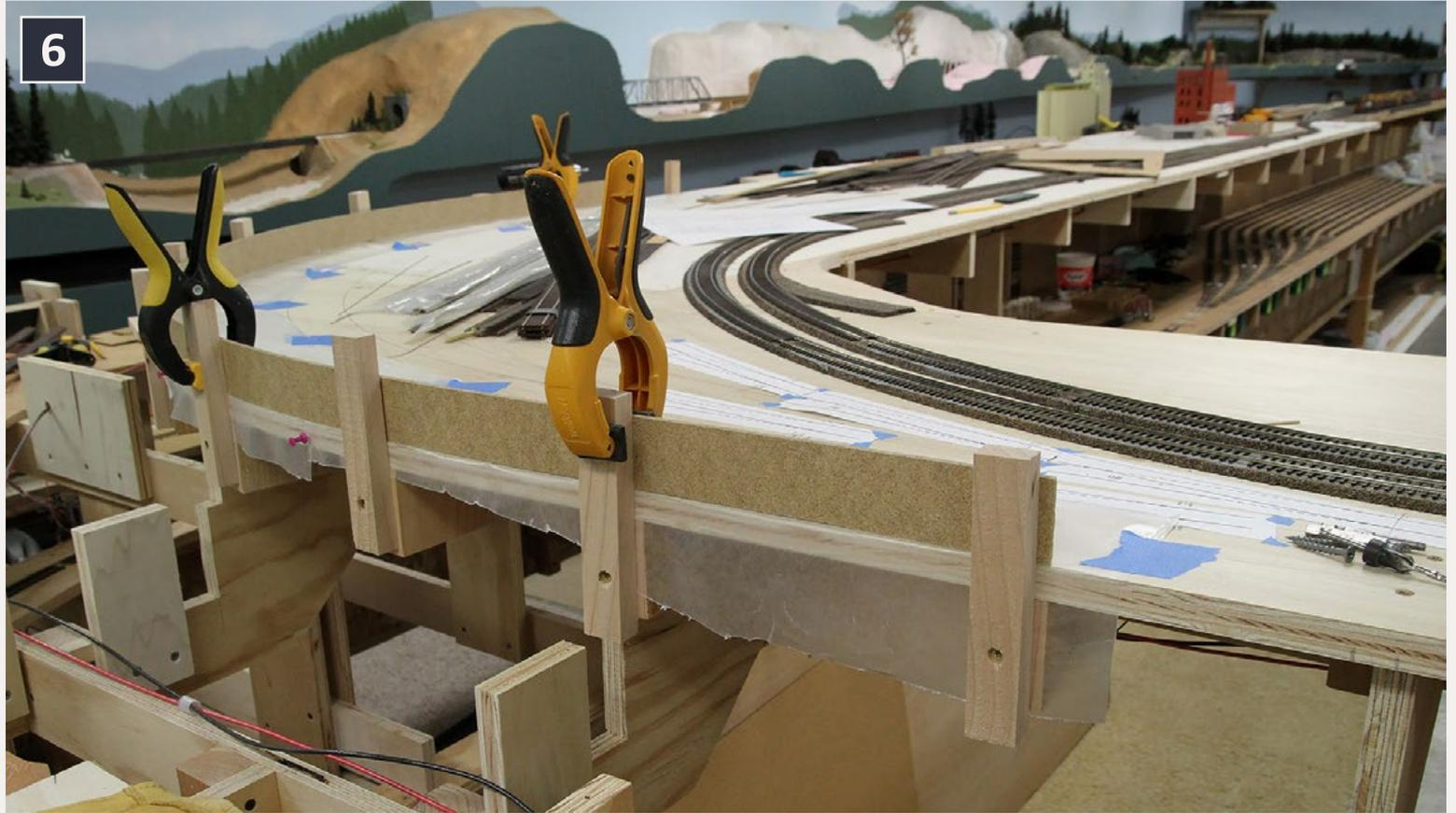
6. I screwed cleats to the edge of the sub-roadbed. By clamping the splines to them, the resultant Masonite serpent matches the curvature of the sub-roadbed edge.
