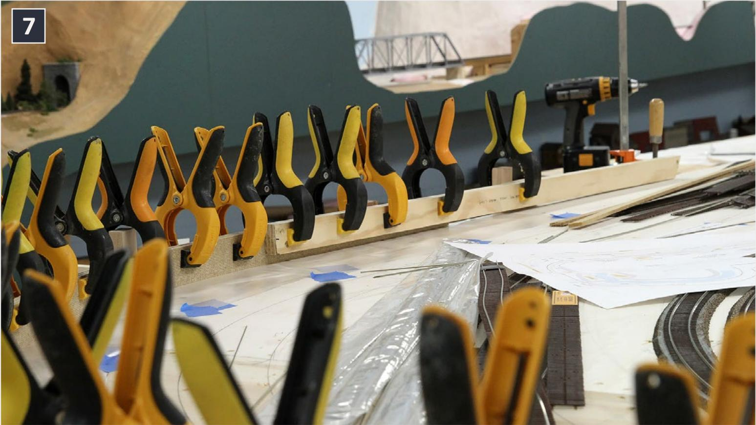
7. At the end of the curves I clamp the splines to a straight piece of scrap wood. If splines are not clamped to something straight while the glue cures, they won't end up straight.
