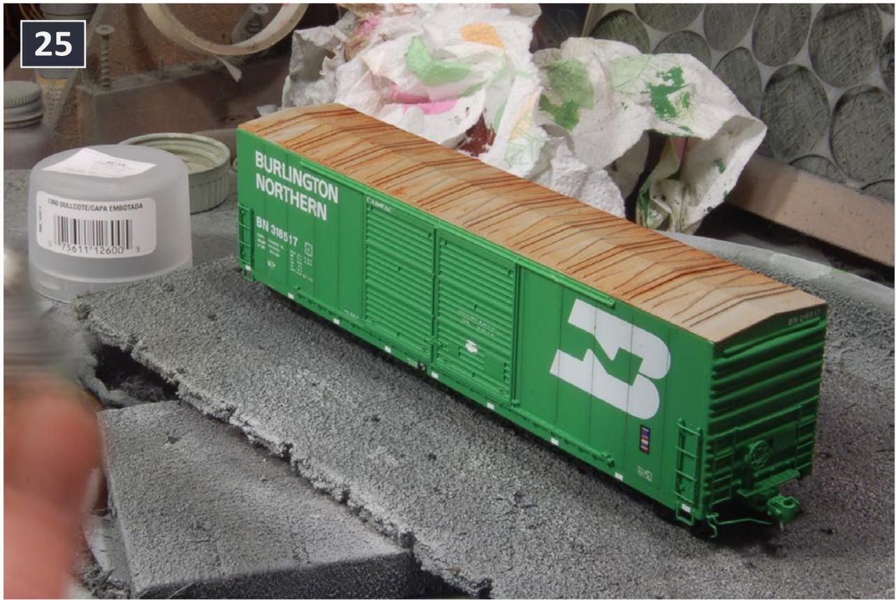
25. I spray the car with Testors Dullcote to hide decal edges and give the model a correct-looking dead flat finish.
