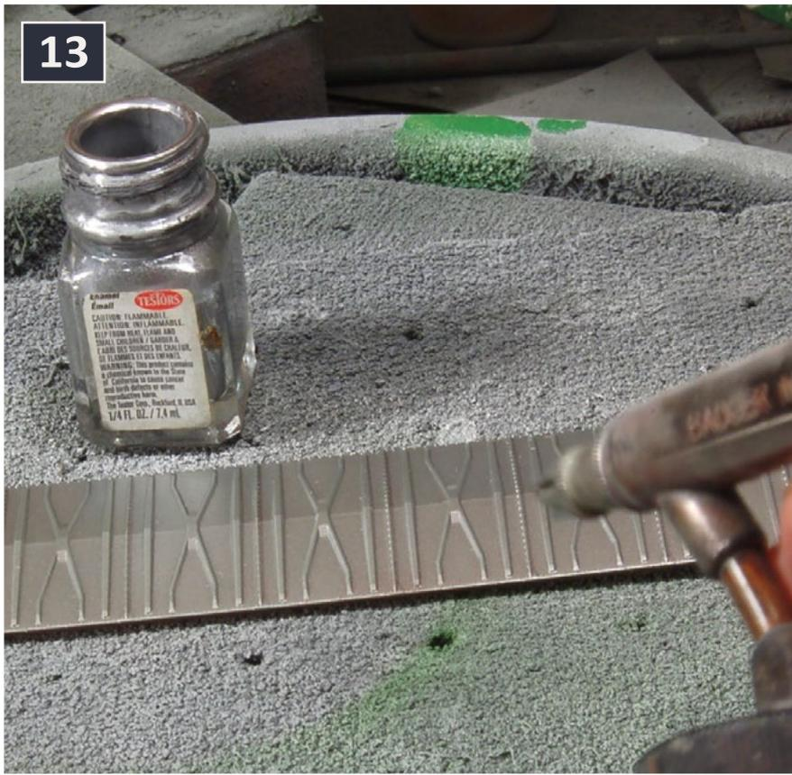
13. I decided the best way to capture the look of the galvanized aluminum roof was to first airbrush Testors Silver.
