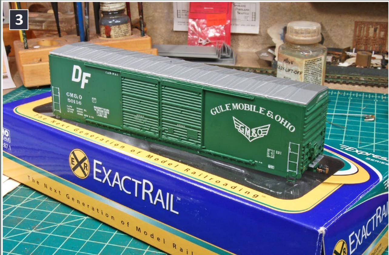
3. The factory GM&O ExactRail model will be repainted and decaled as BN 318517. I start by removing the cast-on side ladders and will install new ones from Detail Associates.
