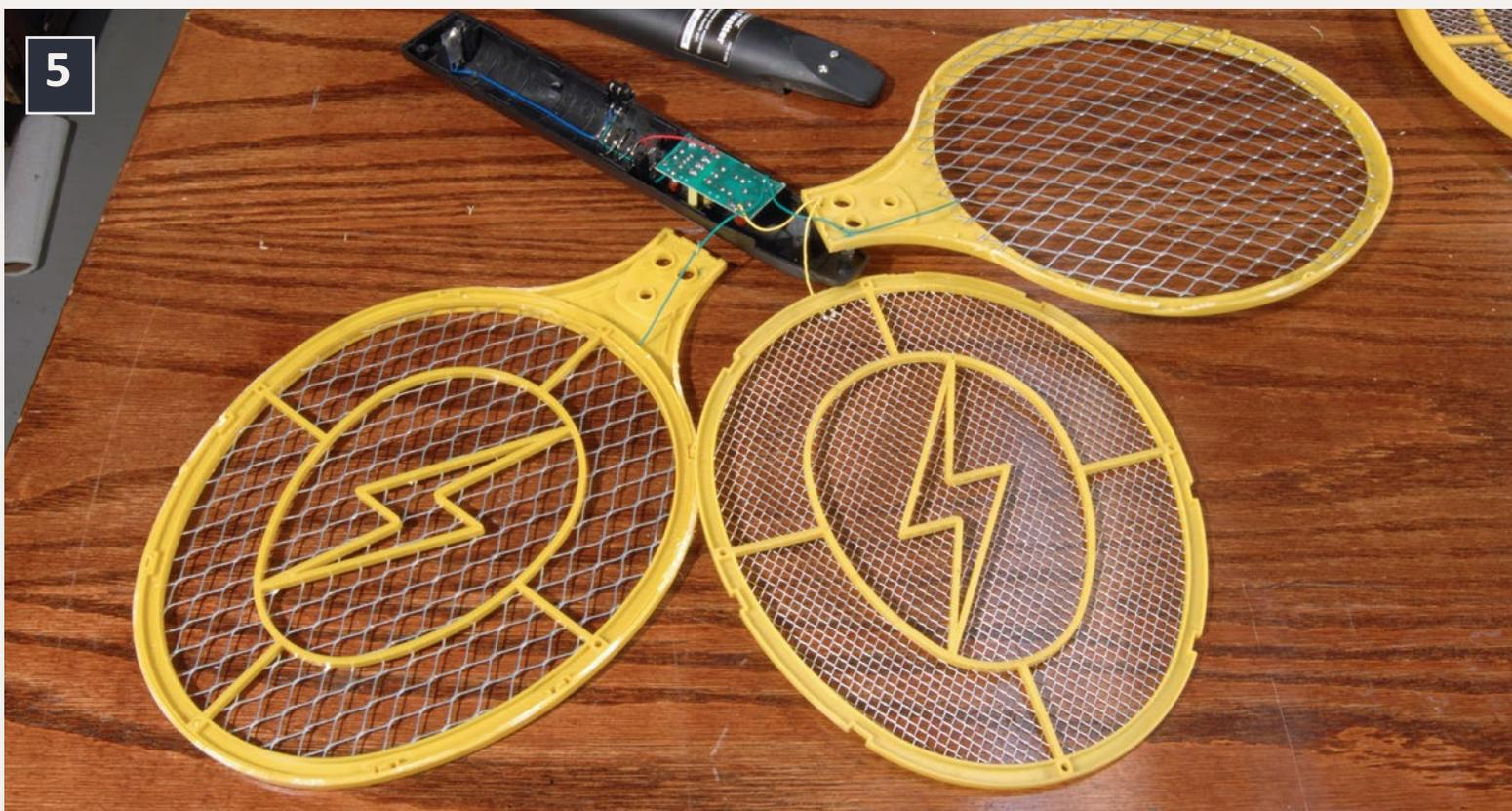
5: This is the unit cut apart. Save the screens for sifting rock and dirt. The outside edge was cut with a jewelers saw.
