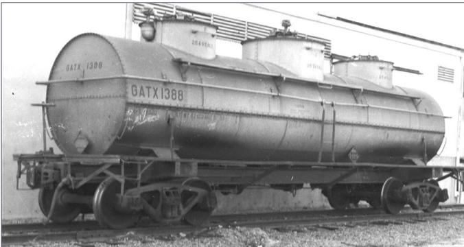
28. Some three-compartment cars that had been converted from single-compartment cars (note the larger center dome) also
