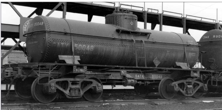
2. 4,000 gallon tank cars were more common. This one, built by General American in January 1928, was still in revenue service when photographed at Los Angeles in the early 1970s. Note the two-horizontal-section tank, the substantial wood blocks between the bolsters and small diameter tank, and the underframe design which, with minor revisions, was later designated by GATC as the Type 30.
