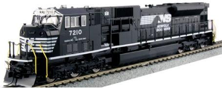
Kato's HO scale version features operating ditch lights, and directional headlights. The models have numerous detail parts that are to be installed by the consumer, including grab irons, MU hoses, and individually molded windshield wipers. DCC models feature factory installed ESU LokSound DCC/Sound. DC models come with a standard 8-pin plug to ease installation of an aftermarket decoder.
