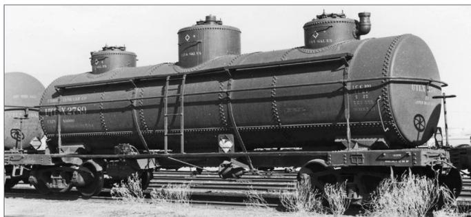
24. Another single-compartment car converted to three compartments was UTLX 2789, Again, the large center dome reveals
