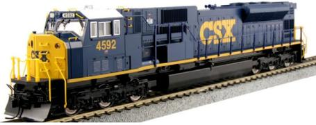
purchased them new from EMD in 1996. Notable features of the big prototype locomotive are its 5,000-hp capability and ease of operating at 75 mph. They are equipped with the special high-tech radial trucks designed to reduce the angle of wear between wheels and rail.
