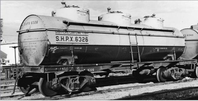
25. Both General American and American Car & Foundry built multiple compartment tank cars specifically to transport bulk
