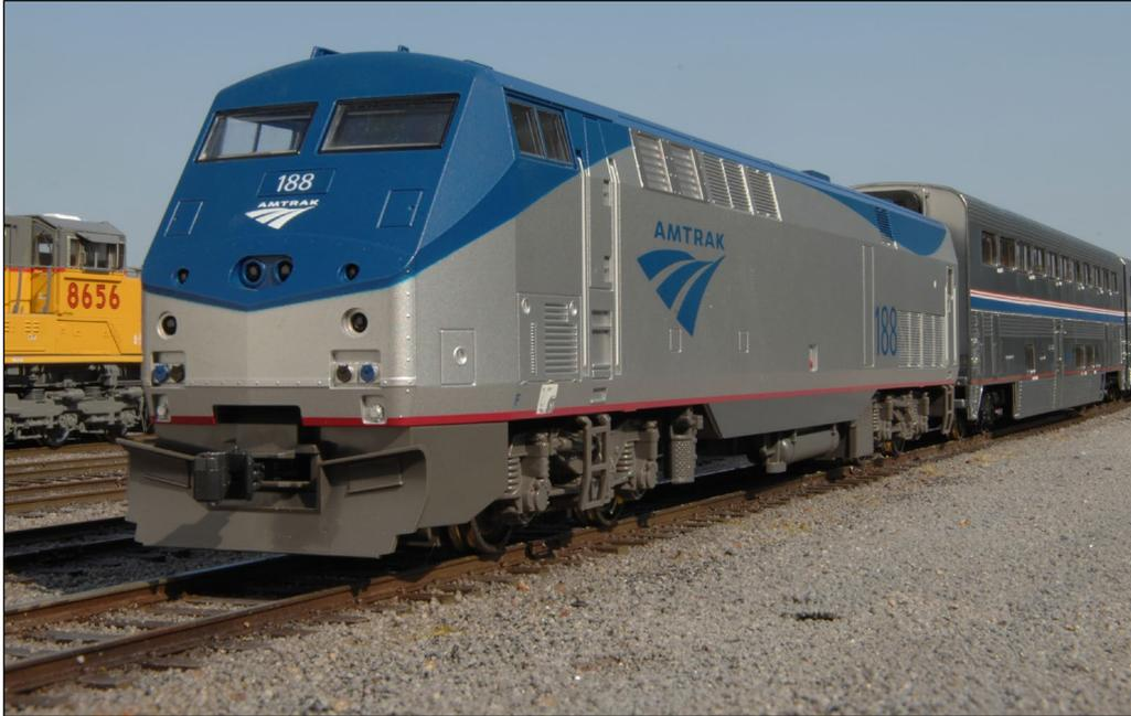
6-7. Kato's new Amtrak locomotive has its motors in the trucks. I bought one a few weeks back just to see if this design could hold up to hours of mainline service. The motors are only  $\frac{1}{4}$ " in diameter but they can pull your walls down with their torque. The latest coreless motor technology is what led to this design, and I'll bet we will see more manufacturers go this route.
