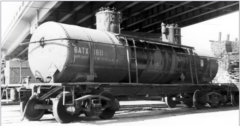
10. Built by General American in January 1926, GATX 1611 was a 6,000 gallon two-compartment car. Again, note the small diameter domes with safety valves on elbows. Oil spills like those shown here were common when cars were being loaded. This car was still in revenue service in the early 1970s when photographed at Bakersfield, CA.
