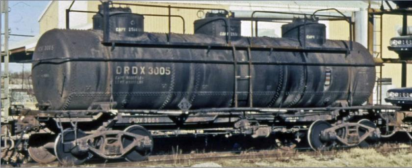
11. This 6,000 gallon three compartment car, built by General American in the mid-1920s, is seen here in the 1970s with elaborate handrails added to the dome running boards and lots of rust showing. DRDX was the reporting mark for the Duredo Co., a tank car lessor which first appeared in the late 1940s and specialized in refurbishing older second-hand cars. Duredo was a subsidiary of Chicago-based John H. Grace & Co. Lloyd Keyser photo
