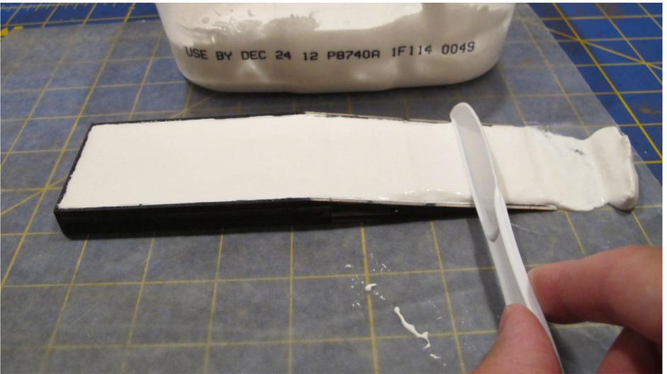
15. Once the frame was filled I used a plastic knife to gently level the Hydrocal on top of the ramp.
