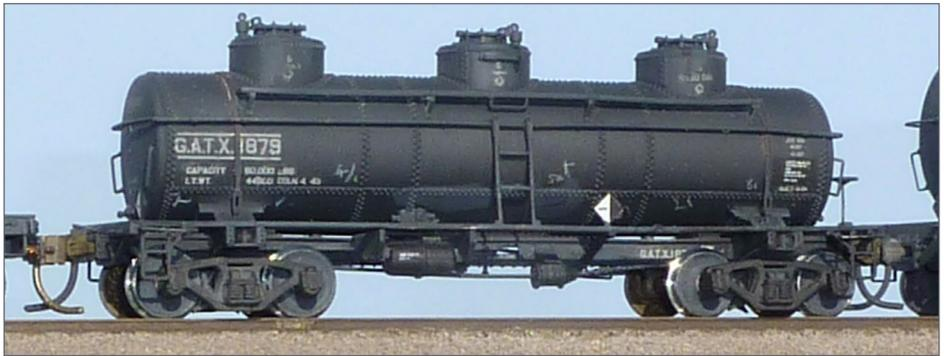
35. An assembled but undecorated Tangent model was painted and lettered with Black Cat decals to represent a car repainted before 1946 with lines above and below the reporting marks and numbers. Weathering includes dirty wheels with treads polished, rust stains around the tank bands, chalk marks, spillage on the domes, and rusty couplers. Model and photo by the author.
