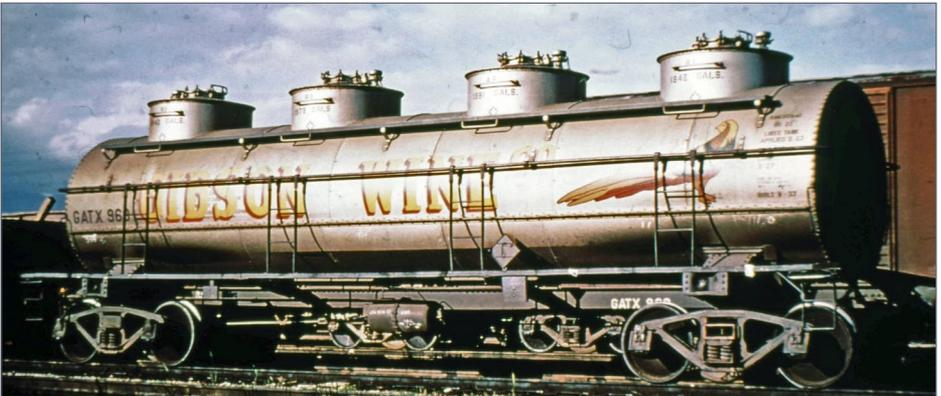
26. Four-compartment wine tank cars were usually of about 8,000 gallons total capacity. GATX 969, built in 1937, was on lease to the Gibson Wine Co. in the 1950s with colorful Gibson stenciling on its aluminum painted tank. Jim Gerstley collection courtesy of Dan Smith
