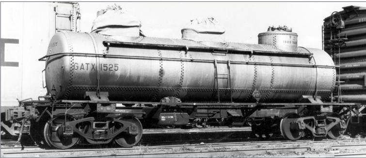
16. The tank was painted aluminum on GATX 1525 when photographed at Schiller Park IL in May 1968, so weathering is even more visible than on black cars. Note the mismatched trucks. Canvas covers over the domes, or safety valves, were often used when the tanks were empty to prevent the safety valves and manway covers from being contaminated. Bill Raia collection
