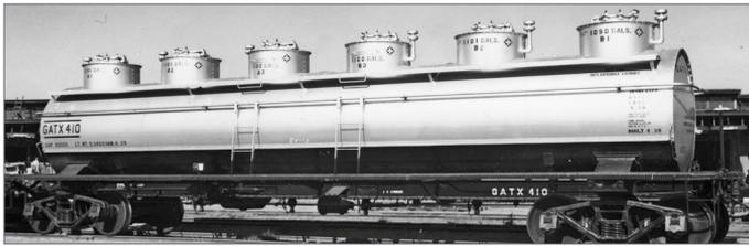
27. Six compartment wine tank car GATX 410 was built in June 1939 and is shown
