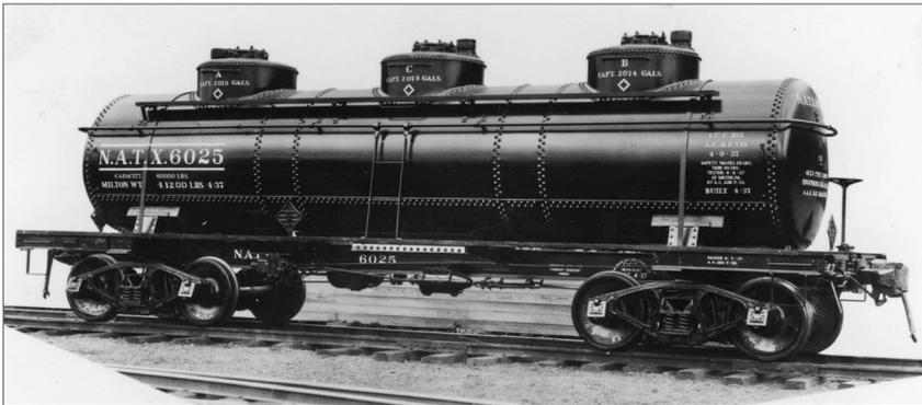
20. This American Car & Foundry builder's portrait shows a three-compartment 6,000 gallon car built on an AC&F Type 27 underframe in April 1937 for North American Tank Line. Mechanical equipment included AB air brakes and Barber Stabilized S-2 trucks with spring planks. Hawkins-Wider-Long collection
