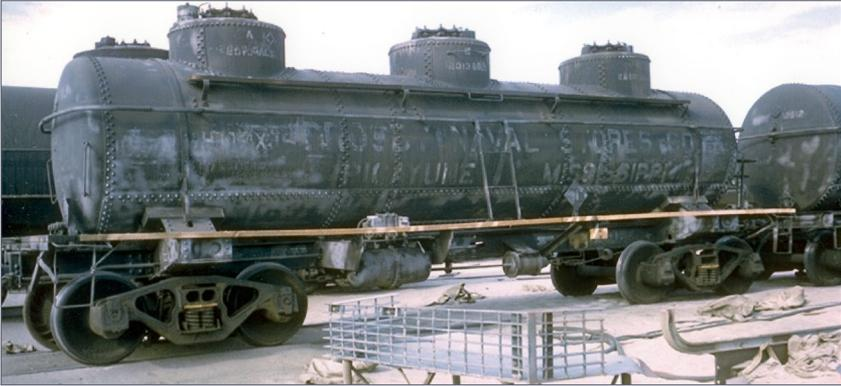
19. The number is illegible on this 6,000 gallon three-compartment General American car because it was in the process of being sandblasted and repainted at GATC's Colton CA maintenance and repair yard. A new wood running board had also just been installed. This car had formerly been in the service of the Crosby Naval Stores Co. of Pickayune, MS, a supplier of turpentine and other products made from pine sap.
