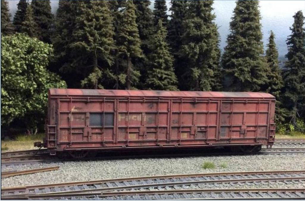
5. Jappe Vander Bort posted this photo of a Walthers ready-to-run Thrall all-door boxcar. He detailed the car by adding grab irons, Cal Scale air hose, Kadee #158 couplers, and Kadee ACL Barber S-2 roller bearing self-centering trucks. He weathered the car using artist oil paints in layers. He also used weathering powders diluted with hairspray to add some micro texture. As Jappe says, "no photo was used to copy the weathering, just common sense."
