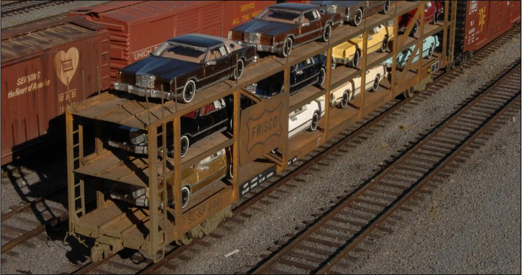
8-9. Mike Budde stopped by with some finished autorack loads he just completed. These are HO 1974 Lincoln Mark V models made using 3D prototyping. He hollowed them out to cut out the windows, sanded and primed the exterior, and painted them the actual colors from the correct color chips for their year. Vinyl roof skins, window stickers, foil trim and clear tape windows finish these models to a contest quality like I've never seen. The freight car is scratchbuilt and assembled with white glue.
