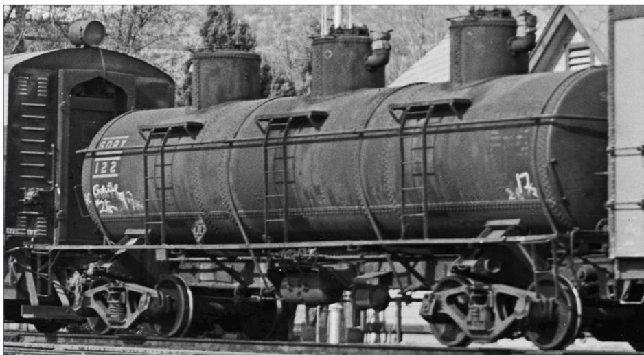
4. The Standard Tank Car Co. built this three-compartment car for the Sinclair Refining Co. in the early 1920s. Small diameter domes with elbow-mounted safety valves were common practice at that time. Note the STC underframe's distinctive bolsters. Most Sinclair cars had billboard "SINCLAIR" stenciling on their tanks, but maneuvering that large a stencil behind all the ladders on this car would have been a serious challenge.
