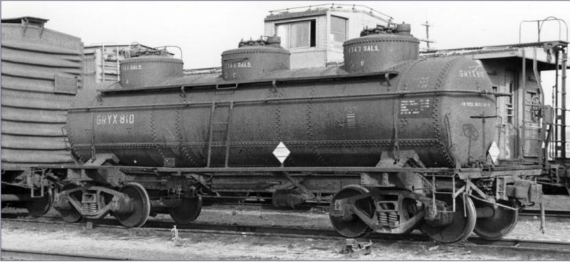
17. Another car owned by John H. Grace and Co., GRYX 810 was photographed on the Union Pacific in Wyoming shortly after its tank, heater coils, and safety valves had been tested in February 1972. It was loaded with a hazardous commodity, as attested by the “Dangerous” placards on the placard holders. Frank Peacock photo
