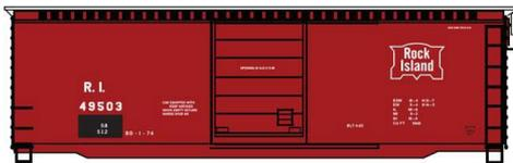
Also new from Mask Island are decals for a Rock Island 40’ boxcar with a roof hatch for bauxite loading (above) and a Texas & Pacific 40’
