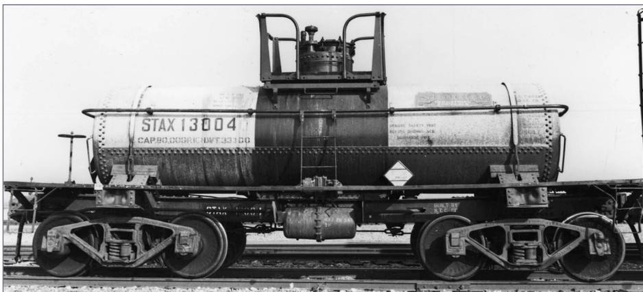
1. There were few 2,000 gallon capacity tank cars, but here is one. This acid tank car was built for the Stauffer Chemical Co. in the late 1920s and photographed at San Jose, CA in November 1956. W.C. Whittaker photo
