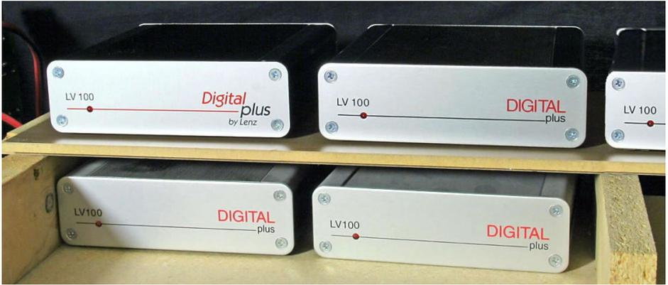
**9. On my HO Siskiyou Line, I use centrally-located Lenz LV100 boosters, rated at 3.5 amps each, for my five power districts. However, as I add more sound units to the layout, I'm finding a need to move up to 5 amp boosters. Because I'm using sub-block current limit protection wiring, moving to higher amp boosters won't cause any problem.**
