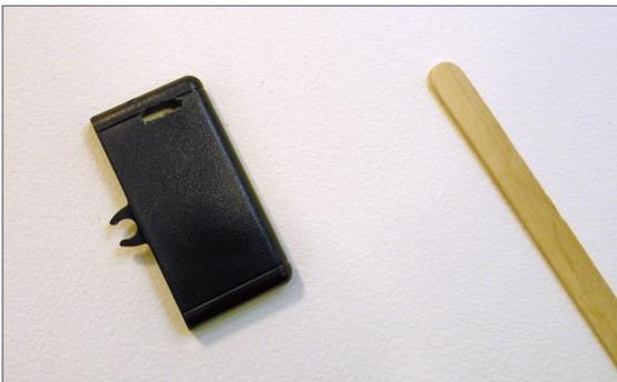
Using a jeweler's saw or one of the small bits for the Dremel motor tool, or even a series of drilled holes, cut a slot for the popsicle stick to slide through. Sand the edges of the slot smooth.
