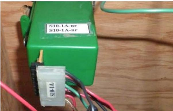
27. Identification labels have been applied to the switch machines and plugs.
