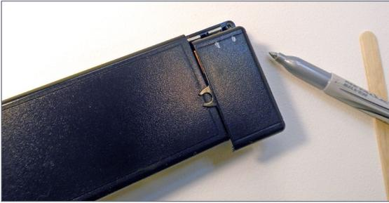
Take the battery cover, and mark where the positive electrical contact lines up. Make it wide enough for the popsicle stick.
