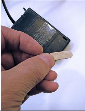
Now when you want to use the throttle, simply pull the popsicle stick out and put it in your pocket. That turns the power on. At the end of the session, slide the popsicle stick back in, and your batteries will be saved for the next time you use the throttle. That is a lot easier than pulling the battery cover off and taking the battery out, or reversing the battery and putting the cover back on again!
