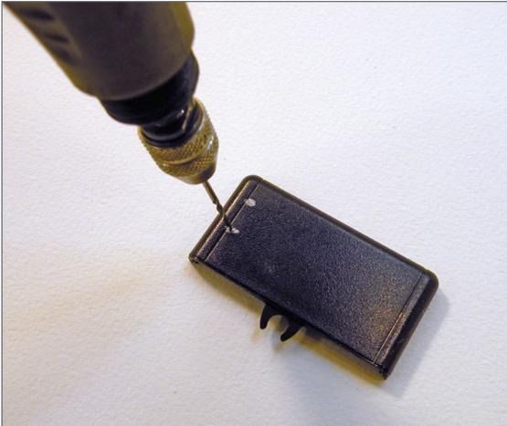
Drill holes at the marked locations, note that there's already a groove molded onto the back of the cover. You want to drill just inside this groove. Marking the starting position with the point of a hobby knife will help to get the holes in the right place.
