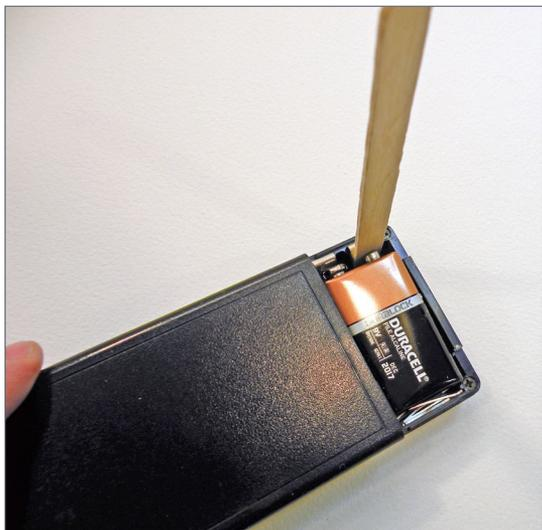
If you have it thin enough, the popsicle stick should slide easily between the positive terminal on the battery and the electrical contact. You have just turned the power off!
