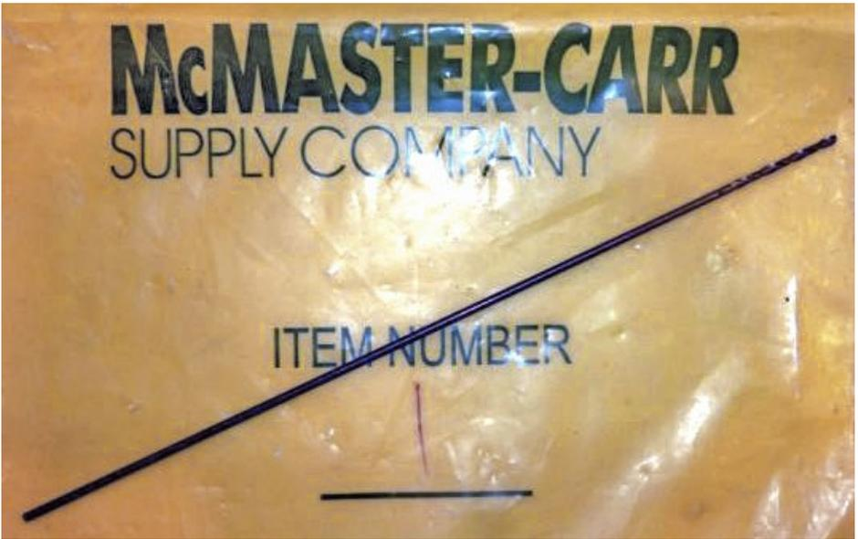
3. Six-inch drill for feeder wires.
