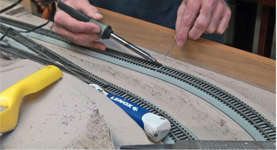
I use resistance soldering to add jumper wires to garden railroad track. It works well on code 250 rail without melting because it produces a great amount of heat in less than a second. The rail quickly gets very hot at the joint, without spreading very much. This tool also works great for fabricating brass models.
