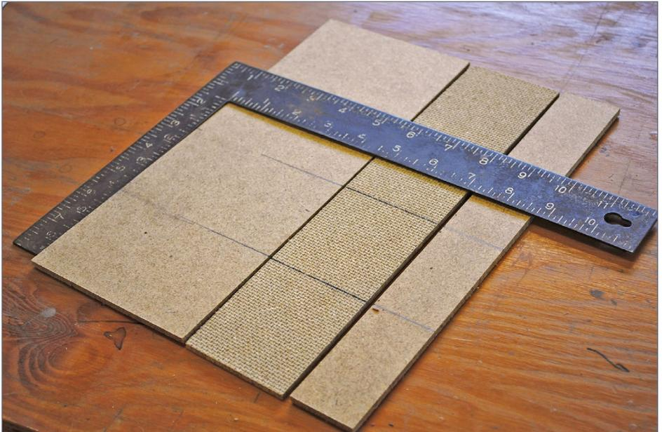
4-5. Cutting the dividers, and marking the glue lines.
