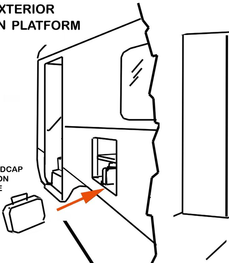
13. Baggage elevators were used to prevent delays at stations. In lowered position they could be accessed from the outside sliding door, and when raised, the carry-on luggage was accessible for passengers in the car.
