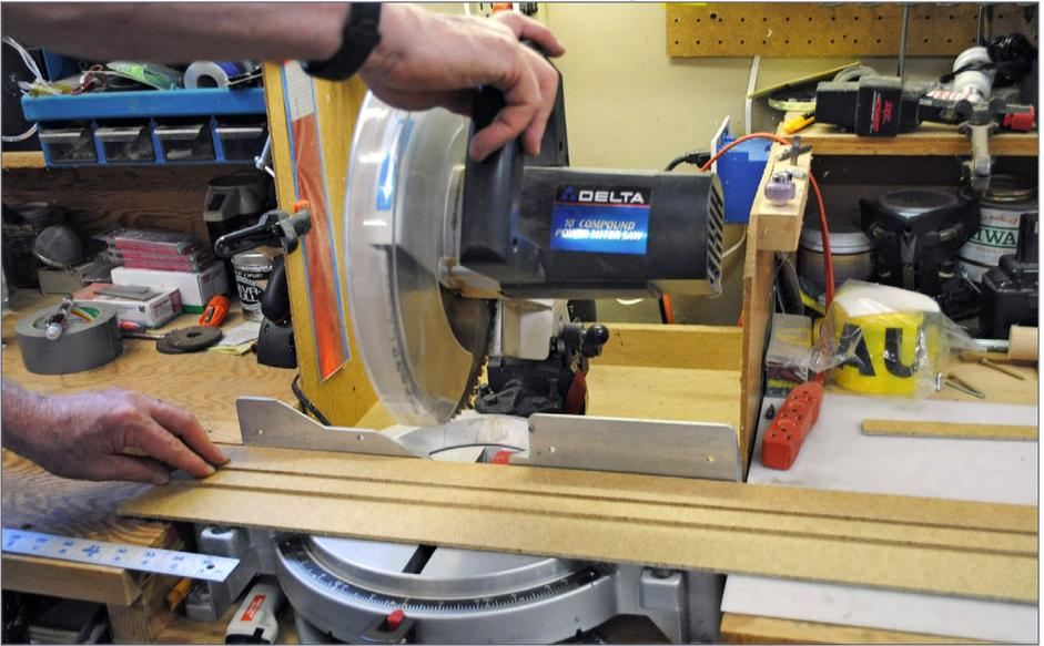
3. Chop saw cutting front, back, and bottom at one time so all will be the same length.
