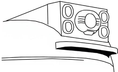
The center flush-mounted light was usually replaced with an oscillating Mars light. Some of the cars, as 2954, 2955 and T&NO car 951 had their Mars light set in a raised fairing while other cars such as 2950, 2951 and 2953 kept their flush mounting for the Mars light.
