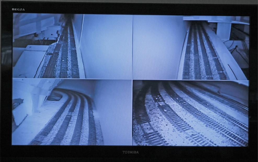
16. Infrared video cameras in the hidden staging areas are a real boon to monitoring what's happening in this trackage. Jeff installed inexpensive off-the-shelf surveillance packages, and the video feed plugs right into any TV monitor.
