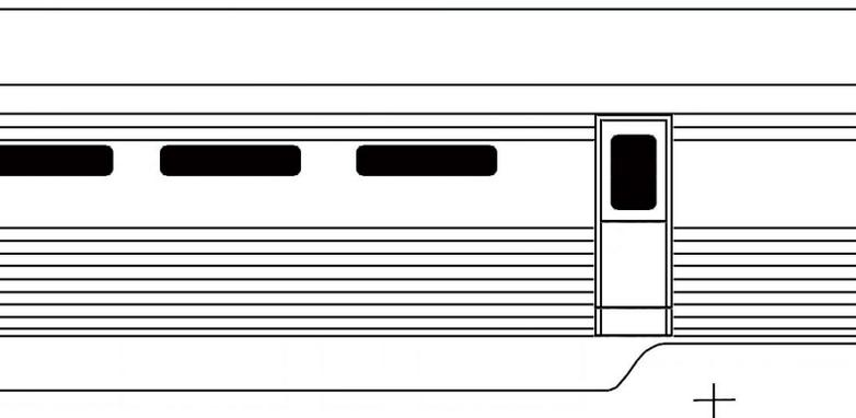
As built, there was a single kitchen door and two loading windows. This was changed with an additional door replacing each loading window.
