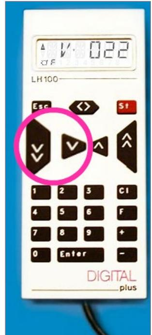
3. Lenz LH100 button control throttle – the down speed controls are circled, the up speed controls are the buttons on the right.
