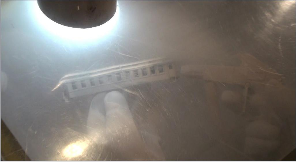
21. Here you see the inside of my North Coast sandblaster. I am using a full-size ceramic gun with 220 grit aluminum oxide. This size is very fine and will not pit the brass. I used about 50 psi of air pressure during this process. A vacuum system sucks the sand out of the air in the booth to allow a clear view of the work.
