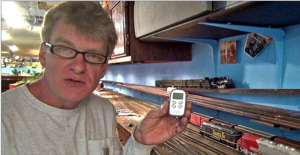
24. I can measure the pulling drag of any given train with this Micro-Mark digital weight scale that allows very fine measurements.
