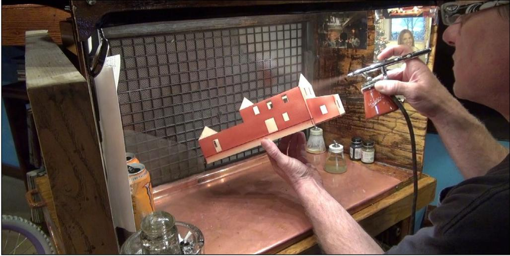
9. Using an airbrush, I painted the main walls with Floquil Tuscan paint. My formula is 25 psi of air pressure, and the paint thinned 50 percent.
