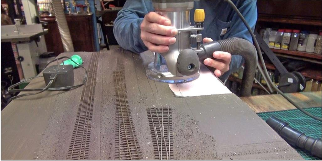
15. Turning my attention to the diorama where the building will sit, I used a router and a hot foam cutter to cut away the foam to the depth of the Plexiglas, making for a flush fit. I then glued the building to the Plexiglas base.
