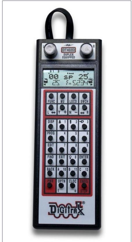
6. Digitrax DT400 series throttle with two encoder speed controls (black knobs) and a small display screen – the duplex radio DT402D model is shown.
