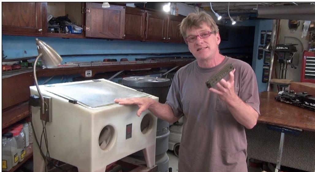
20. For this month's video tool tips, we discuss and demonstrate sandblasting brass models. Most models come with a lacquer clearcoat. When painted over, this can really cover up a lot of details. Sandblasting the model to remove the clear lacquer makes for a smooth finish with all the detail popping out at you.
