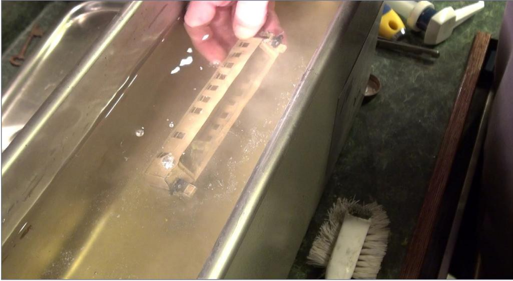
22. After blasting the model, I wash it in water from the sink and brush off the loose sand from the model. No matter how much you wash and brush the model, when you place it in the ultrasonic cleaner a dust cloud forms in the bath as all the dust from every crevice starts to float free. Now you have a clean model ready for paint. You can watch the entire process in this month's video in real time.
