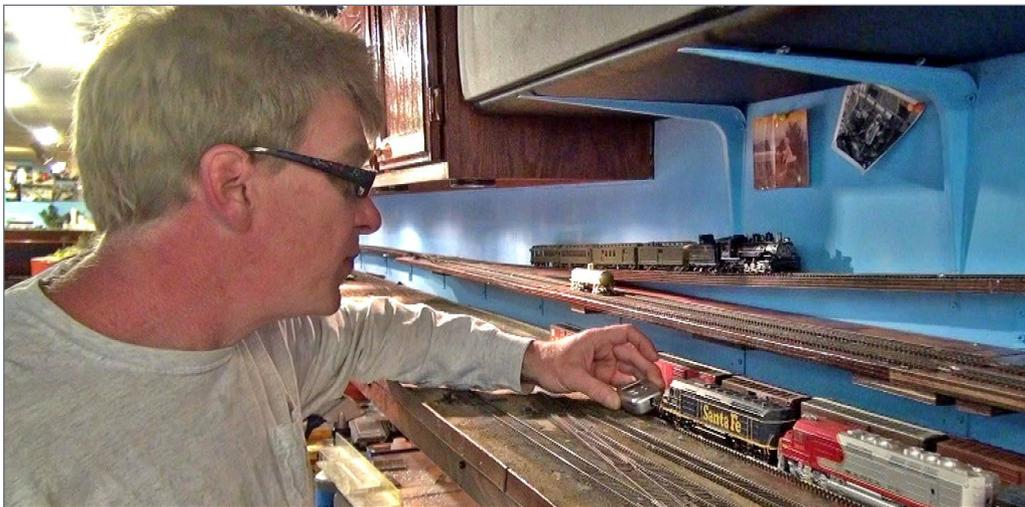
25. I adapted a Kadee coupler to the measuring scale so I could connect it to locomotives or freight cars and measure the dead drag or pulling ability of the models.
