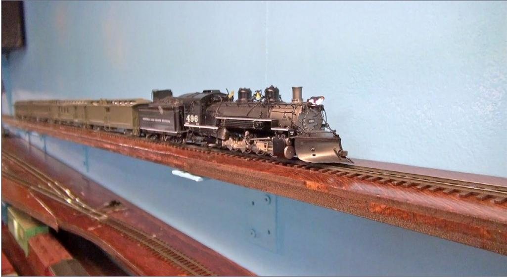
23. I have this K-37 scale brass model that could not pull four older brass passenger cars up a 4 percent grade. The brass trucks from the '60s don't roll very well and have a lot of drag. The solution was to replace the older trucks with free-rolling new Blackstone aftermarket passenger car trucks, reducing the pulling drag from 1.2 ounces to a half-ounce. Now the locomotive can easily pull the train up the 4 percent to the upper town.
