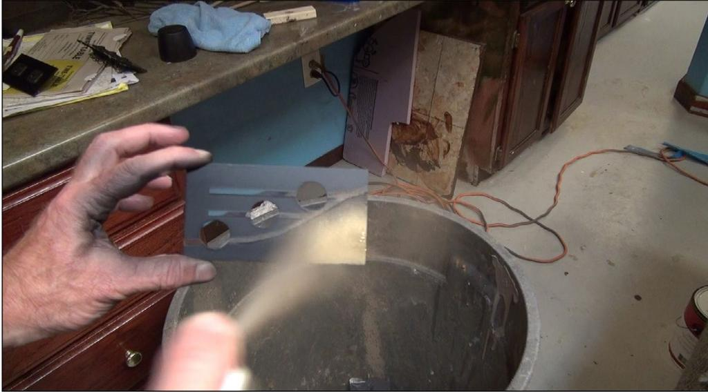
4. After removing the tape, I sprayed the back of the panel with gold paint.
