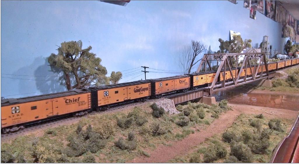
26. My HO scale 62-car reefer train had a pulling drag of over 4.5 ounces. By replacing the trucks with Kato after-market trucks I was able to reduce the drag of the consist of cars to 2.2 ounces – more than half. Trains now run better with fewer coupler separation problems.
