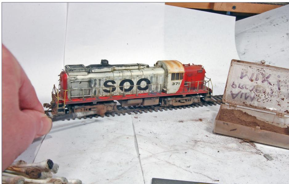
10. A common weathering pattern found on prototype Soo diesels were rust streaks on the cab roof. I simulate this effect by using quick passes with my airbrush and Floquil Rust.
