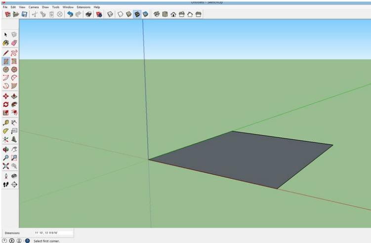
1. Here is the basic sequence used to draw something in 3D using SketchUp. Begin by using the Rectangle Tool (highlighted in the Tool Bar along the left side of the screen) to draw a rectangle.
