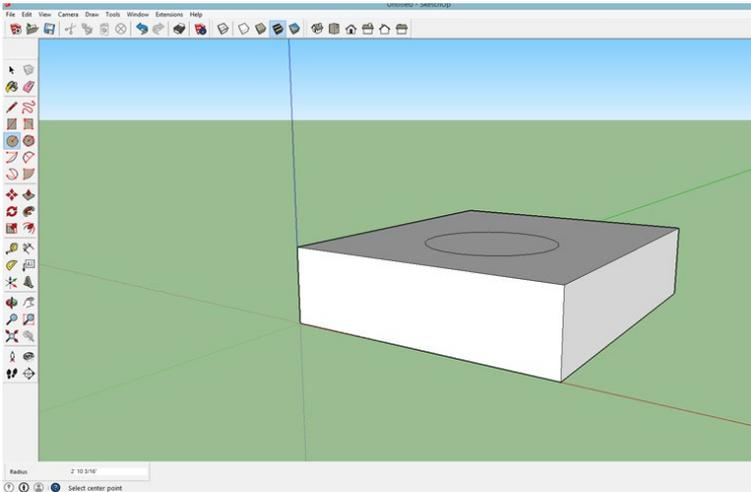
3. The same Push-Pull Tool is used to make circular holes. First use the Circle Tool to draw a circle on the top of the part.
