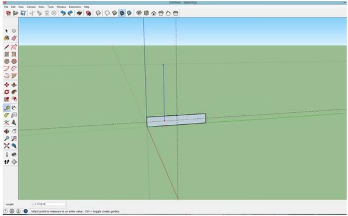
15. Select the Circle Tool and click on the intersection of the two last guidelines. Start drawing a circle and then type "48" into the measure box to create a 48-inch-diameter circle.
