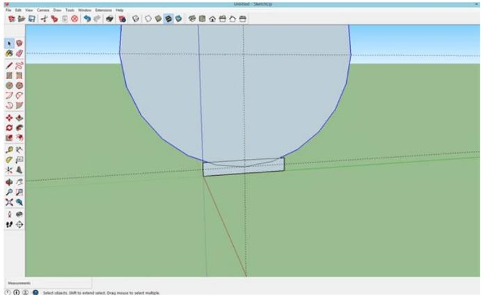
17. When one shape overlaps another shape, as in this case, it results in three parts which are 1, the large part of the circle; 2, the remaining small part of the circle; and 3, the remainder of the rectangle.
