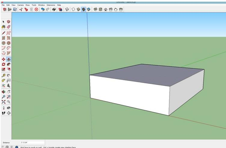
2. Then use the Push-Pull Tool (highlighted), click on the rectangle, and move the mouse upward, creating a 3D solid.
