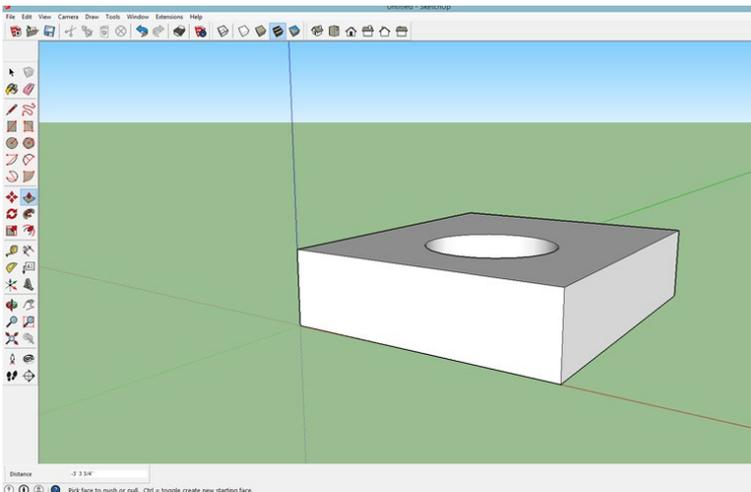
4. Click on the circle with the Push-Pull Tool and then move the mouse downward to create a hole.
