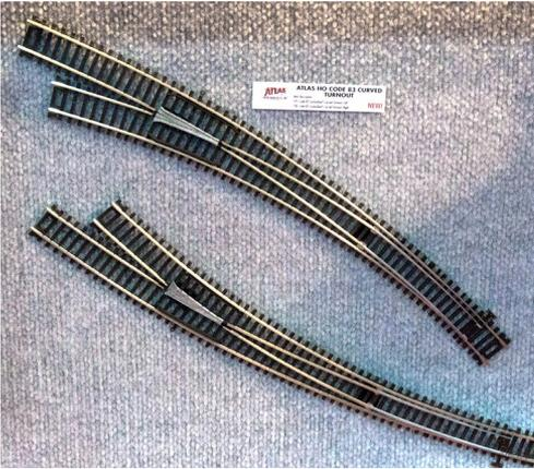
Atlas has announced plans to produce code 83 nickel silver curved turnouts. The HO turnouts have die-cast points and an isolated, die-cast frog with a power contact to optionally energize the frog and prevent momentary loss of contact when a powered model is passing through
