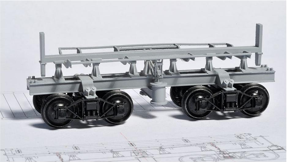
23. Here is the printed frame resting on the trucks. The bed itself will be built up with stripwood and the end levers and other small parts reproduced using photo-etching. As of this writing, the model is still under construction. But getting this far would have been impossible without using 3D printing.
