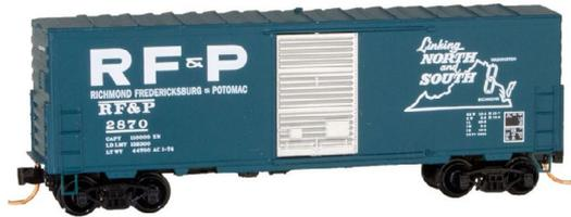
The prototype of this Richmond, Fredericksburg & Potomac 40-foot boxcar was rebuilt in 1974. The update included removing the running board and shortening the right-hand side ladder. For additional information on all Micro-Trains Line models contact a dealer or visit [micro-trainsline.com](http://micro-trainsline.com).
