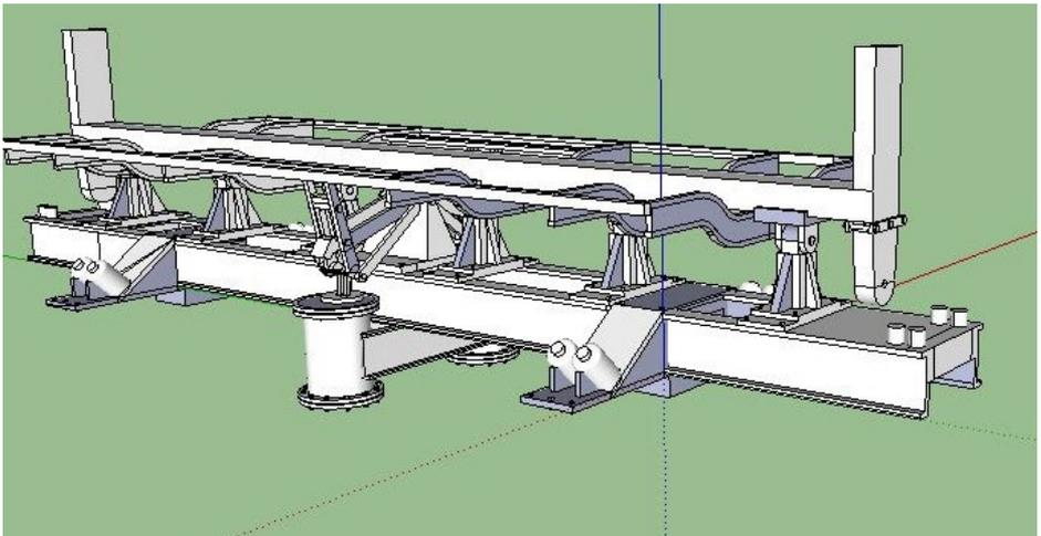
22. After starting with the pair of C channels, a bolster was drawn in line with and to the side of the frame. That bolster was then moved laterally to the truck centerline and a copy moved to the other truck centerline. The same process was used for the pedestals, air cylinders, bed supports, etc. This is a screen grab of the final frame which was printed as a single part.
