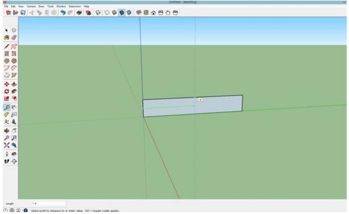
13. Using the same tool, start at the bottom of the rectangle and hesitate near the center. The tool will snap to the horizontal center of the rectangle. This centerline is also 3 inches from the bottom of the rectangle and thus the bottom of the 48-inch-diameter water tank.
