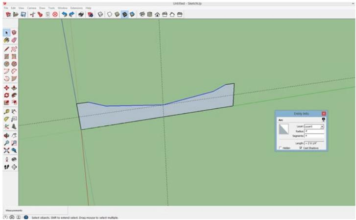
this view. Right click the remainder of the circle to open an Entity Info box. In the entry for Segments, backspace over the number and type in a larger number such as 24 in this case for just the remainder of the circle. If you are drawing a full circle, increase the number of segments to 96.
