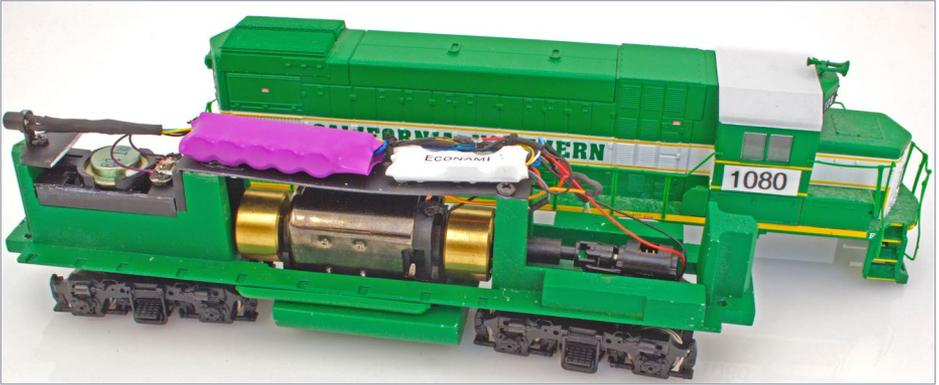
6. ECO-100 diesel and CurrentKeeper installed in a Walthers HO scale GP15-1, using a 16 x 35 mm 8-ohm speaker in a baffle arrangement.
