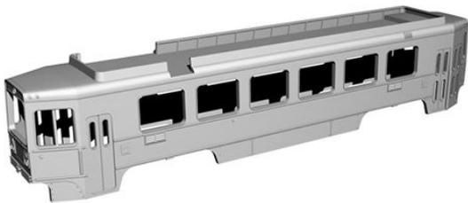
Here is a preview of a Kawasaki double-end Light Rail Vehicle coming soon from Imperial Hobby Products. The HO scale resin model will have injection-molded clear plastic windows. A 3D-printed underframe will be designed for a Bowser drive mechanism. Roof details will also be created by 3D printing and will accommodate a Sommerfeldt pantograph. For additional information visit [ihphobby.tripod.com](http://ihphobby.tripod.com).
