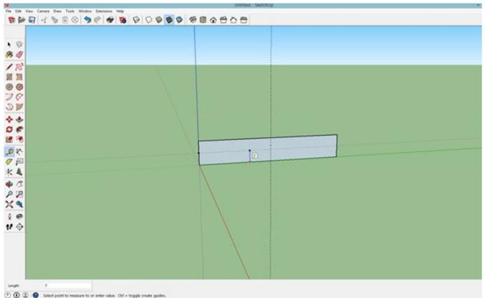
14. Now use the same tool and click on the horizontal line. Drag upward and type "48" into the measurement box on the bottom left of the screen. That will result in another guideline 48 inches above the centerline of the rectangle. That is where we need to draw the circle representing the 48-inch-diameter water tank.
