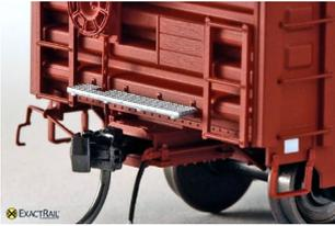
Additional features of this highly detailed Platinum series model include wire grab irons, separately applied door tracks and door locking bars, and Kadee #58 couplers. The model rides on 100-ton ASF Ride Control trucks with 36-inch
