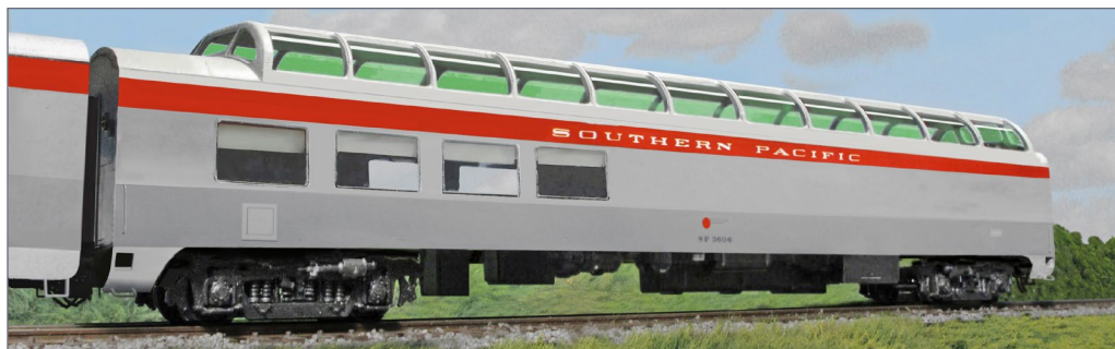
13. Dome lounge car model of SP 3606, showing the later appearance of these cars with stainless sides.
