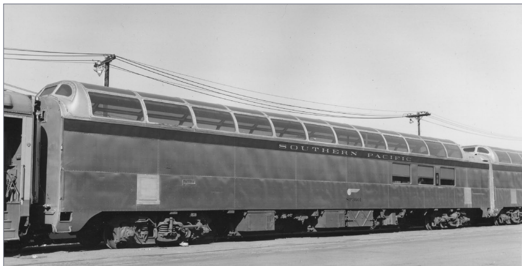
10. SP dome car 3601 in later years after the stainless steel fluting was removed and replaced with polished flat stainless steel side panels. Courtesy Bob's Photos
