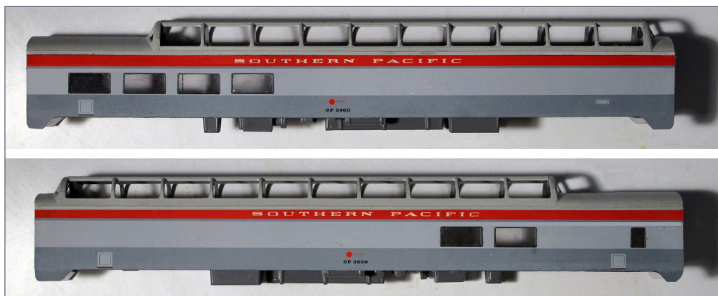
14. Body assemblies for late appearance of car 3600. Note low windows.
