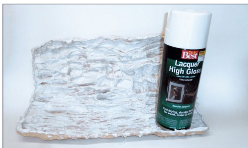
27. Spray the mold with white lacquer paint.
