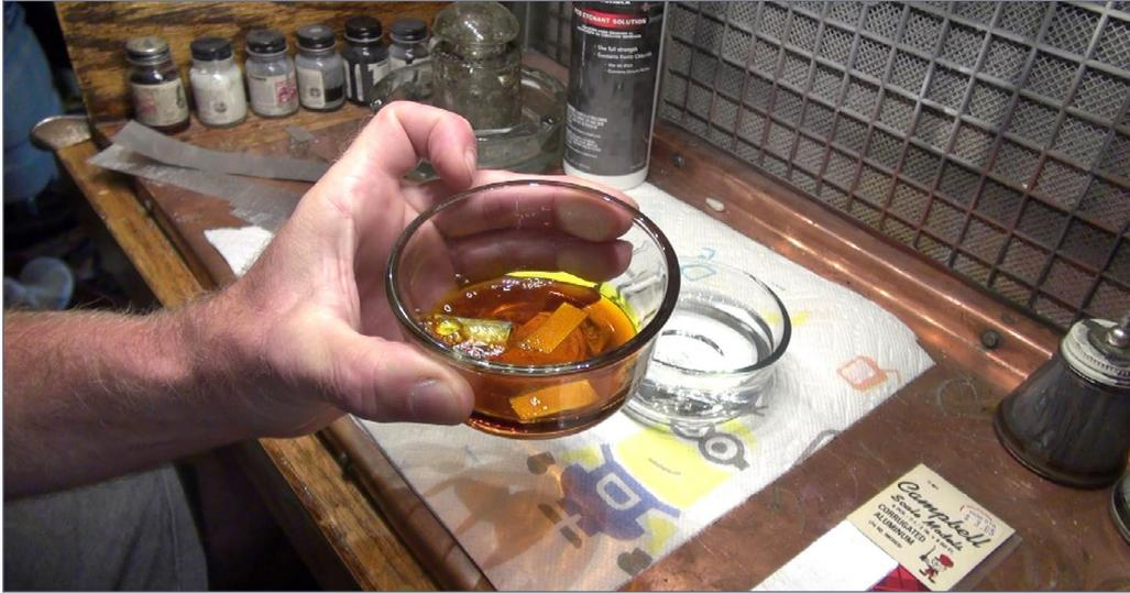
3. I place the metal in the bowl of etchant, and in 20 seconds the boiling process begins. Here you see the violent bubbles as the acid eats away at the metal's surface.
