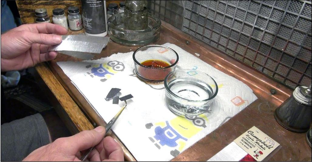
2. The corrugated metal is cut into 3x8 scale foot sections for HO. One bowl is filled with the etchant, and the other with water. The water stops the process.
