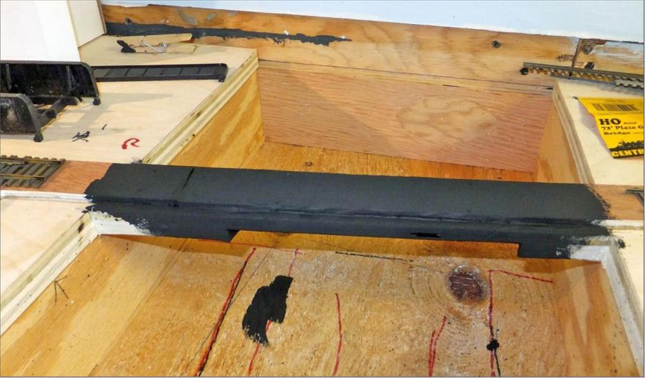
76. I painted the entire portion of sub-roadbed under and around the bridge with a brush and Floquil Engine Black. In relation to the weathered ties and girders, the sub-roadbed will simply look like shadow. Having the dummy open bridge in front also helps to disguise the fact that there is no empty space between the ties of the track in back.
