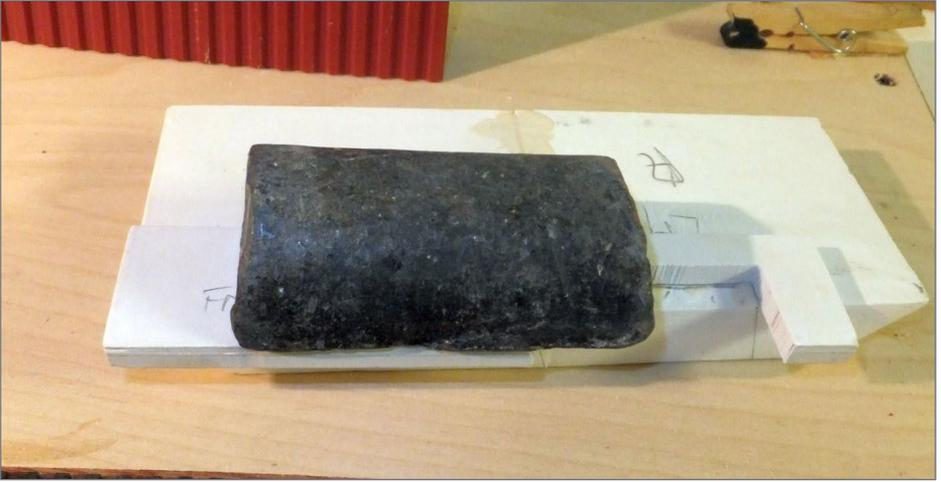
70. A lead weight holds the cut “retaining” portion of the abutment in place while it’s being glued to the abutment. This retaining portion holds back the land and ballast above the abutment height and is at the same level as the bridge shoes and the girder up to ballast level.
