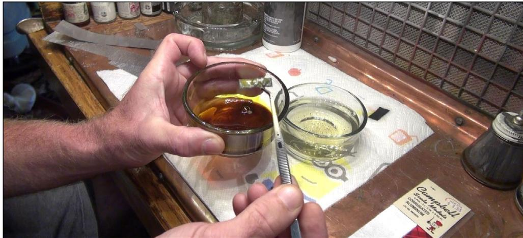
4. I use a pair of tweezers to remove the metal from the acid and place it in a bowl of water to stop the process. If you let it boil for more than 30 seconds the metal will dissolve completely.
