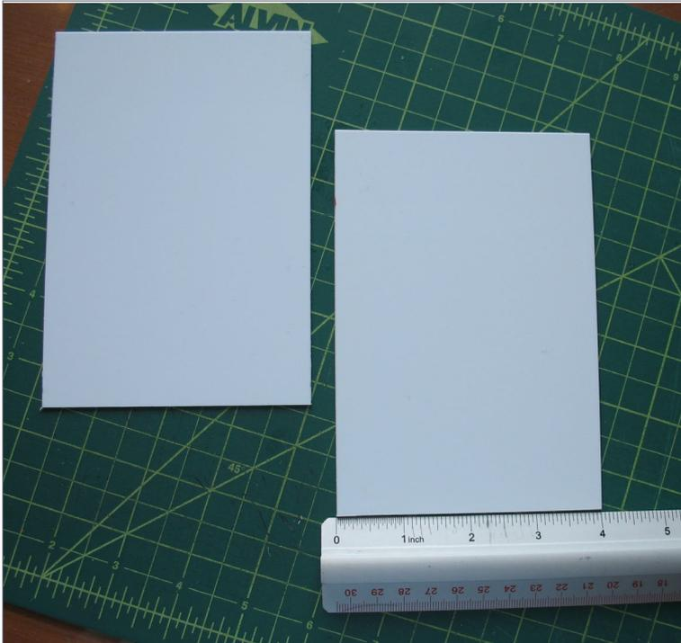
2. Both finished wheel mask sheet blanks, 4" x 6".
