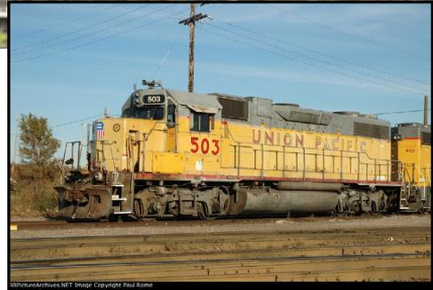
2. Joe Atkinson shared this photo of UP 503 that he took on his layout. Joe shared his work in a post [mrhmag.com/node/24092](https://mrhmag.com/node/24092). He added details, removed the factory lettering and relettered and renumbered the model. Joe faded the unit and weathered the trucks, fuel tank, pilots, and plow with Pan Pastels, but he faded the lettering and shields with yellow, gray, and white acrylics. After comparing the model to the prototype, it's safe to say "Joe, you nailed it".
