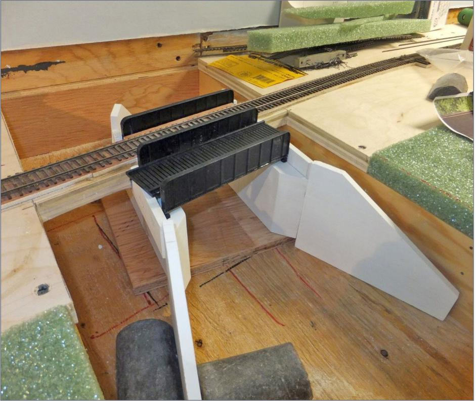
74. To get the feel of what I was doing, I needed to build the abandoned second bridge span, which went together easily. The Central Valley kits are a breeze to assemble with a good bonder such as Pro Weld, and lend themselves to kitbashing. I shortened the girder quite a bit to fit this purpose.
