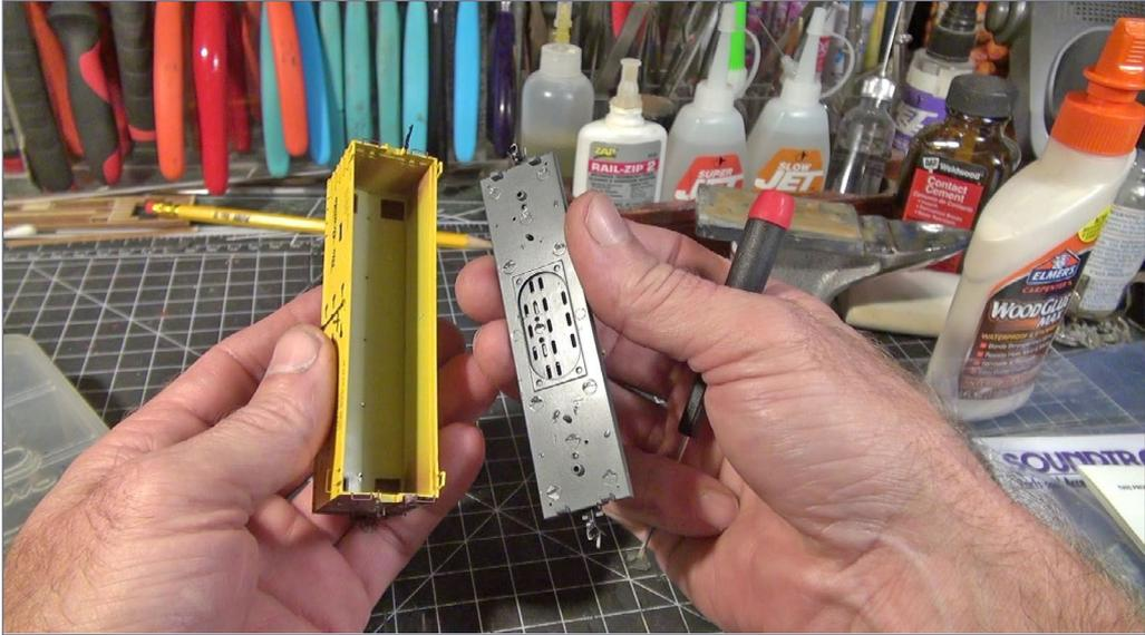
17. I used a screwdriver to carefully pry off the bottom of the reefer to reveal the speaker mount holes in the car's floor.
