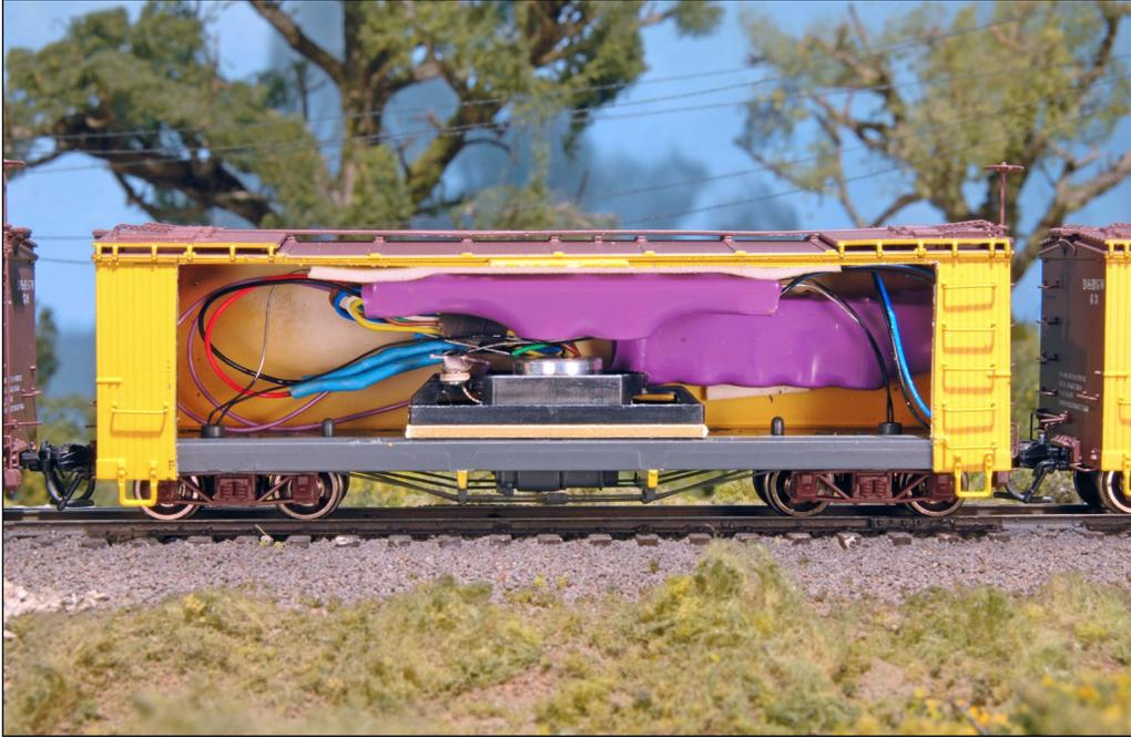
29. A cutaway view of the car shows the decoder and Current Keeper installed along with the speaker. It all fits perfectly. I programmed the car to run a few times with flange squeal and rail joint sounds in combination. Then I programmed it to run with just joint bar click-clack sounds so you can hear the difference in the video.
