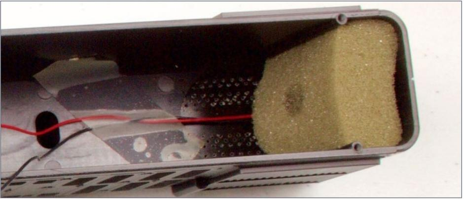
4. Close-up view of the interior, showing “magic” tape holding the bulb wires down. Also, notice the holes that the owner had drilled through the front fan grille.
