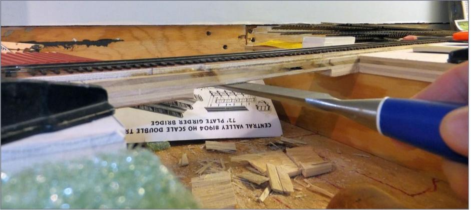
62. I wanted this bridge to capture the feel of the prototype through girder bridge. To have the girders high enough to look “right” to me, I decided to thin the subroadbed under the girders. I made saw cuts with a Japanese dovetail saw, and then chiseled out the area in between.
