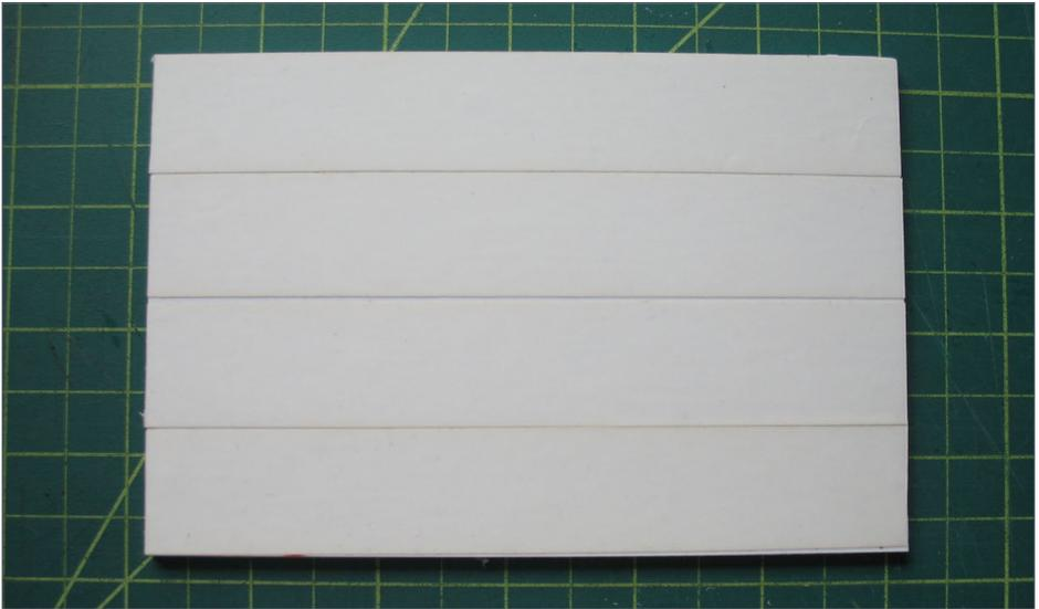
5. Double-stick tape applied to full face of plastic sheet set, to be attached to scrap wood base.
