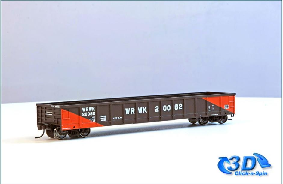
3. In 1975, the Southern Iron and Equipment Co. started building a 52'6", 100-ton gondola. Evans took over SIECO and continued building the cars through December 1981. A total of 1,730 cars were built with three minor body variations. This model represents the second version, and the most common.
