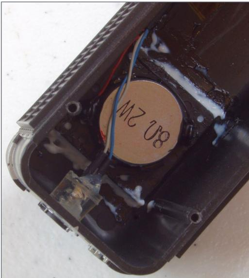
5. The 28 mm square high-bass speaker is mounted inside the shell under the drilled-out fan grille. It is sealed to the shell with clear caulk. The caulk is currently white, as it was applied just before this photo was taken. Note the white caulk plugging the mounting holes in each corner of the speaker. This keeps the sound confined to the side of the cone that generates it.
