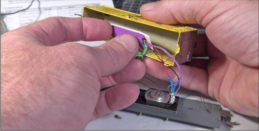
27. I use two-sided foam sticky tape to mount the decoder to the roof of the reefer, and more tape to mount the Current Keeper to the side of the car.
