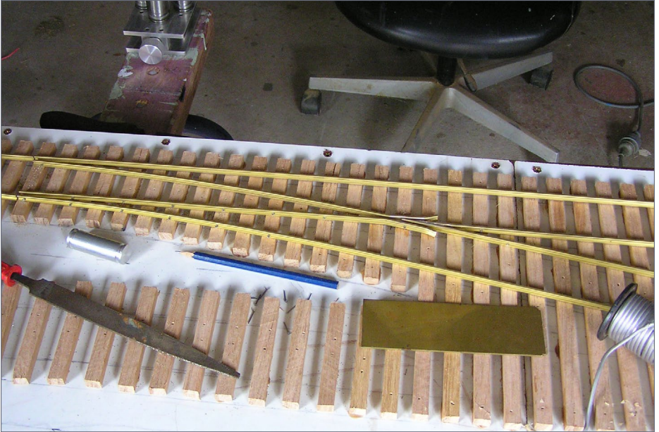
17. Both closure rails are now spiked into place.
