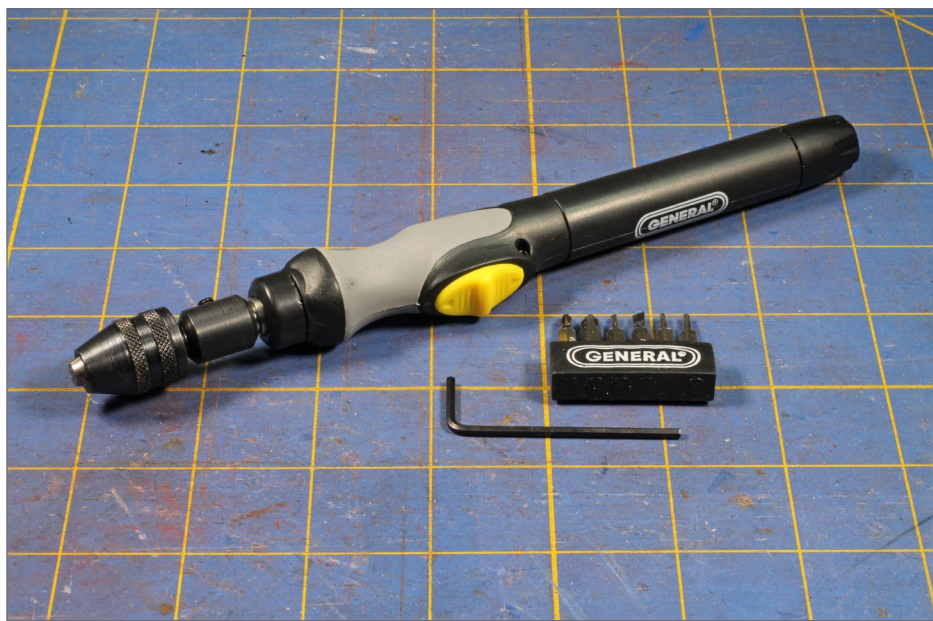
8. A great new tool. A power pin-drill driver.
