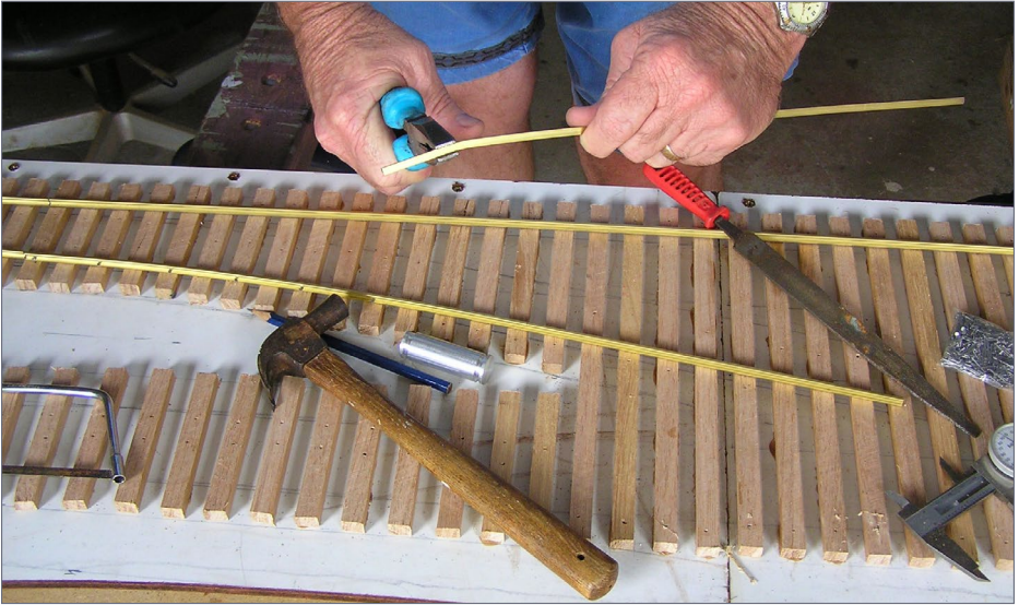
10. Bending the closure rail to form the guardrail.
