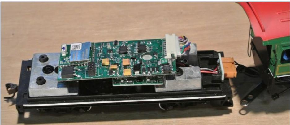
**3. BlueRail Trains' first board is plug-compatible with DCC locomotives using a 9-pin JST connector.**
