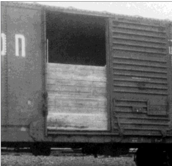
53. Boxcar fitted with boards for hauling grain.
