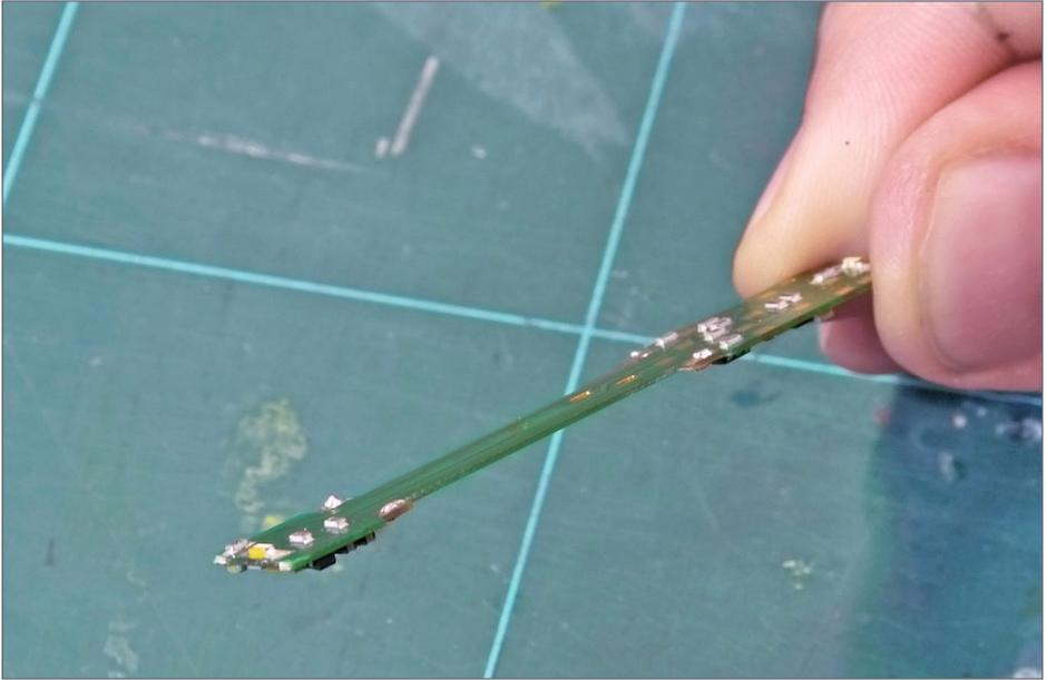
5. I used solder to build up a little dimple on each of the contact plates for reliable conductivity.
