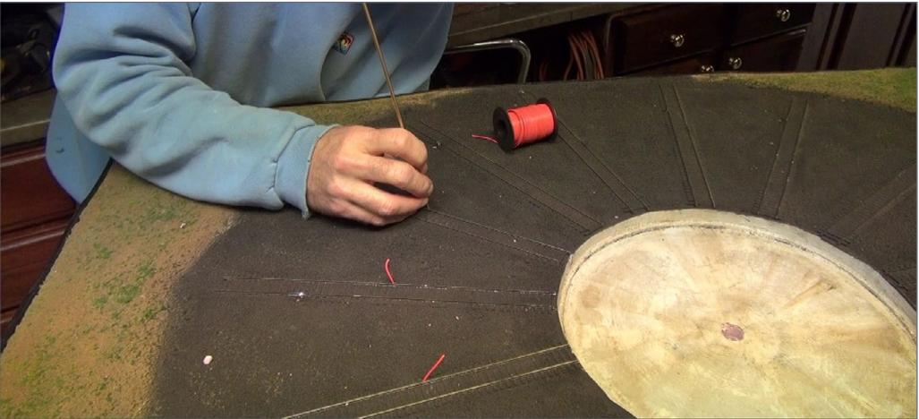
7. To start wiring up the Athearn turntable display, I pressed a brass tube through the foam base to feed a power wire from the rail to the bottom of the scene. I did this for all 22 rails around the pit.
