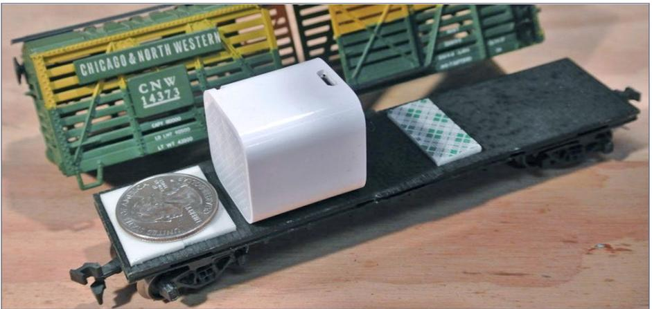
6. Bluetooth (Groove Cube) speaker installed in a stock car to be pulled behind the loco. Sound added for under \$20.
