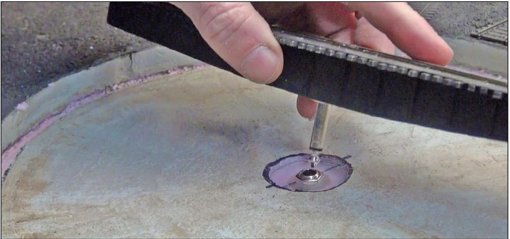
10. I cut a Plexiglas disk and centered a female microphone jack on it. This disk assembly was glued into the bottom of the pit to accept the male microphone jack attached to the turntable, as you see here.
