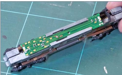
6. The decoder now fits in tightly. The motor contact is provided by the two long-hole notches on the decoder board.
