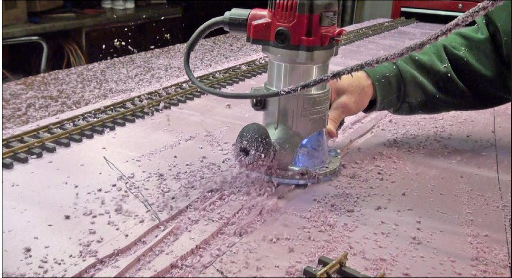
9. Using a router, I cut the foam to a depth of  $\frac{1}{4}$  of an inch to sink the Bachmann G scale track into the scene, saving on ballast.
