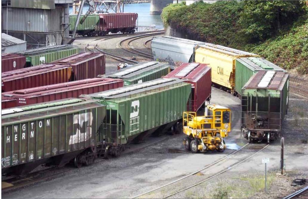
**1. Hopper cars at a modern rail-to-water transfer are moved by a Trackmobile which can maneuver on and off the rails as needed. *Graham Line photo***
