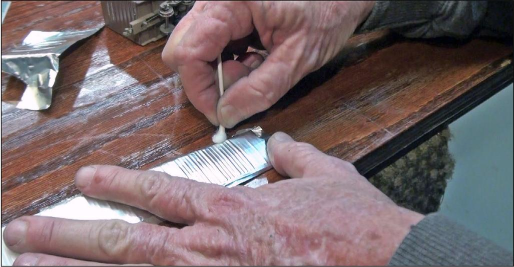
3. With a soft cotton swab, Mike embosses the freight car's detail into the foil. He then paints the foil the correct freight car color and decals it to match the car's lettering. Then he folds and crushes the foil part to match the prototype photos.
