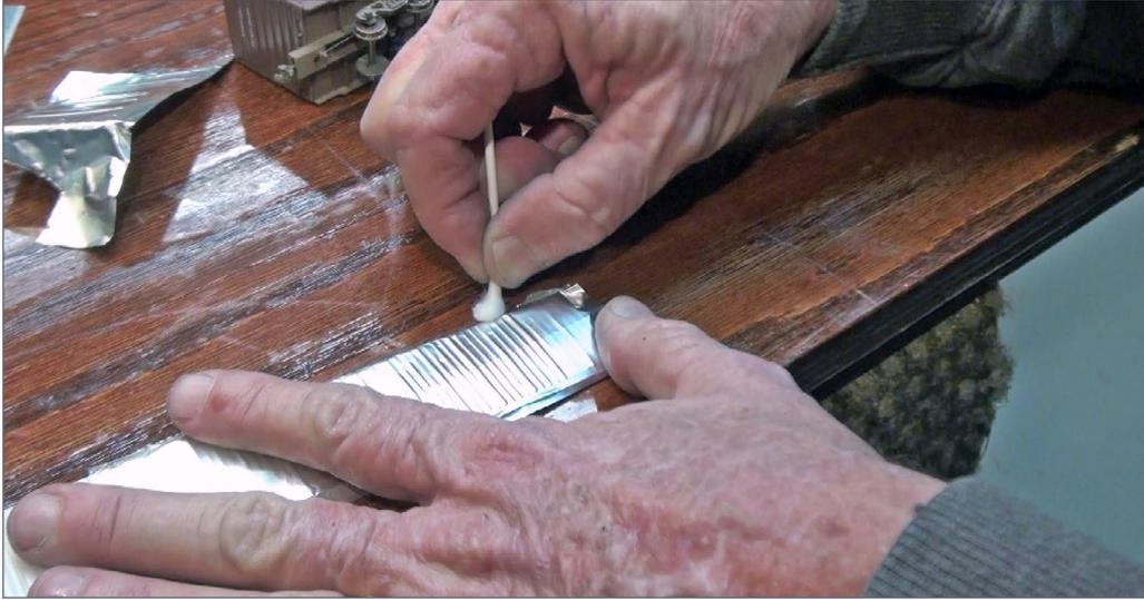
4. Mike makes a roof section from foil using the cotton swab to press and rub the aluminum into the roof panel detail.
