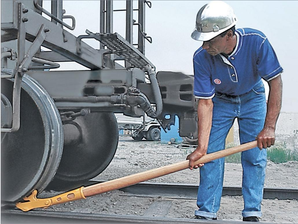
2. A manual car mover, sometimes called a railcar jack, allows a worker to move a car on level track. Shove the tool in between the railhead and the wheel, and push down. The joint at the head of the tool multiplies worker’s efforts through compound leverage. *Aldon Company Inc. photo*
