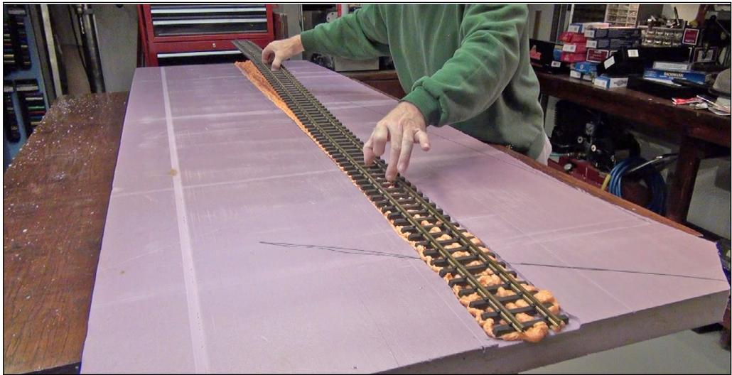
10. I glued the track down using Great Stuff Foam Pro, shaving off the excess foam with a wire brush after it cured.
