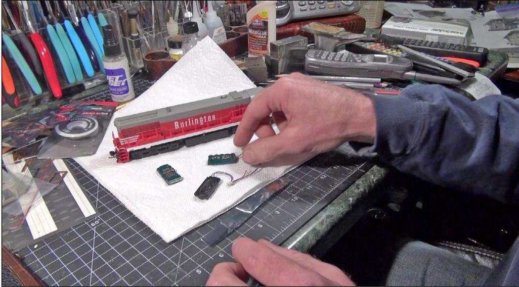
15. Korea Brass USA sent me locomotives without sound so I could demonstrate what goes into the sound decoder installation. Here you see the three components necessary for the conversion: a TCS WOW Sound 101 decoder, a keep-alive module, and a 16x35mm WOW speaker.
