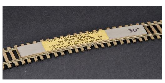
3. Ribbon Rail track-laying tools are machined aluminum templates available in several gauges and radiuses, and in several lengths for straight track. *MRH photo*
