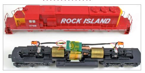
3. TCS T1 decoder installed in blue-box Athearn locomotive - if you wire the motor backwards, fix the wiring, don't change CV 29. See text.
