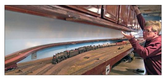
4. This valance hangs under the cabinets for the full 13-foot span of the yard. This provides even and dimmable lighting. It replaces the old puck lights and saves 100 or so watts in electrical use over the old system.
