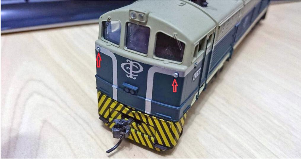
2. So far, lighting descriptions by other modelers have usually referred only to the lights that illuminate the front of the locomotive. Modelers use white or yellow microLEDs for these but have ignored these small rear red lamps, for understandable reasons. The technique presented here uses optic fibers and considerably expands the arsenal of tactics for modelers, as it dramatically reduces the size of the light source.
