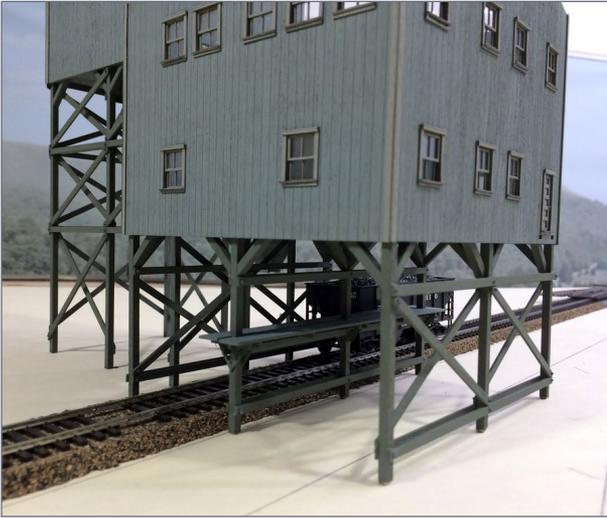
thing is going together nicely and the finish has the “look” that I was aiming for[13-14]. Once the assemblies are glued together, start adding all the detail. The floor is well braced but the walls will probably need bracing to keep them square and prevent warping. After gluing the main building walls together with Titebond, sit it on the base to check the fit. So far so good.
