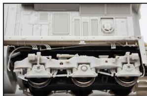
Separately-applied plumbing and traction motor cables.
