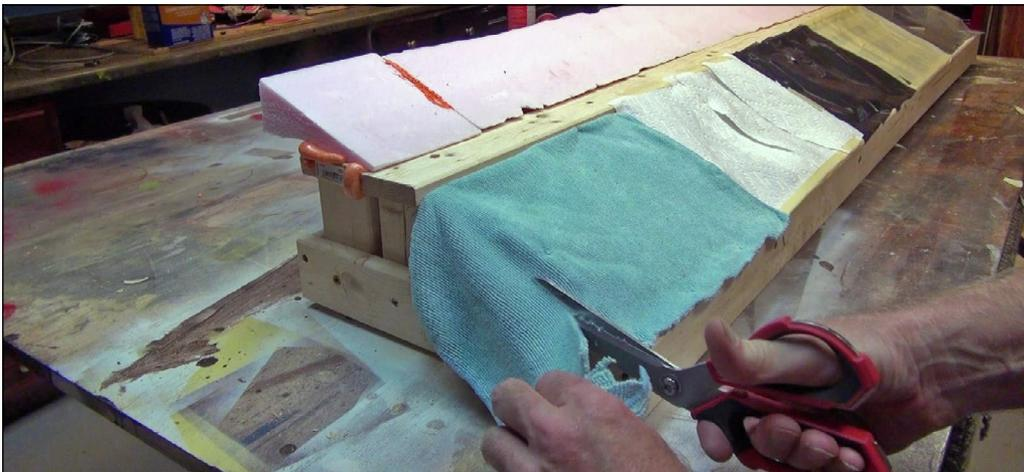
14. In this photo, you see all five sections of the layout with various sub-bases in place: window screen, masking tape, black duct tape, simple paper towels, and blue microfiber cloth. The cloth and wire screen are stapled. The tape sections and paper towels are held in place with tape.
