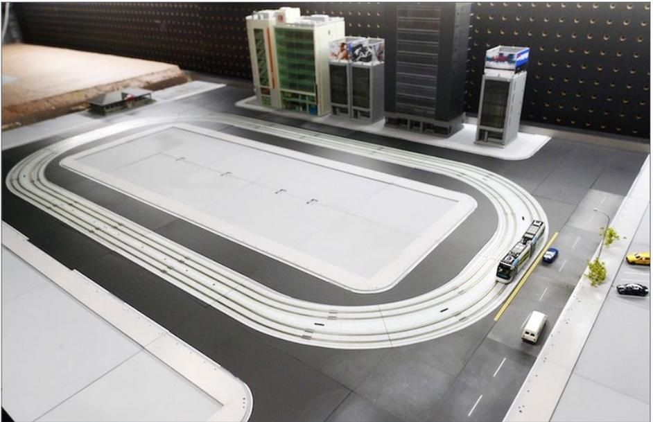
2. An N scale tram system is a major test of track maintenance – rails are buried in pavement, and the lightweight rolling stock has short wheelbases and small wheels.
