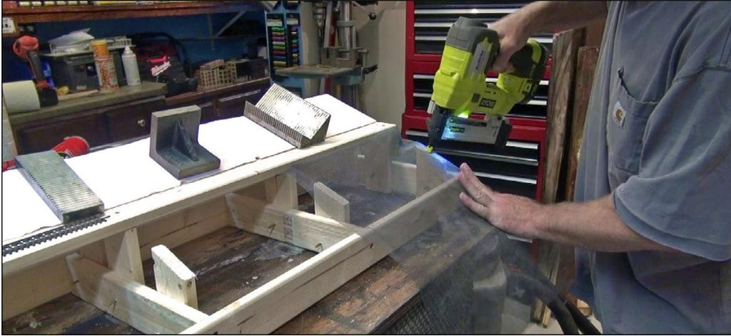
13. I started by stapling fiber window screen to a one-foot-wide segment of the hill. This screen will allow the foam to penetrate just a little, making for very strong foam hardshell scenery.
