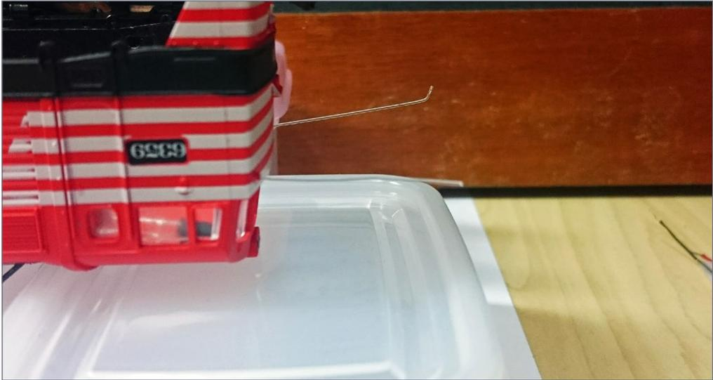
13-16. Remember that these micro lamps are intended to light up at the rear of the locomotive when it is moving forward. Test the lights for proper operation in both directions. After you verify that everything works, use a nail clipper or flush-
