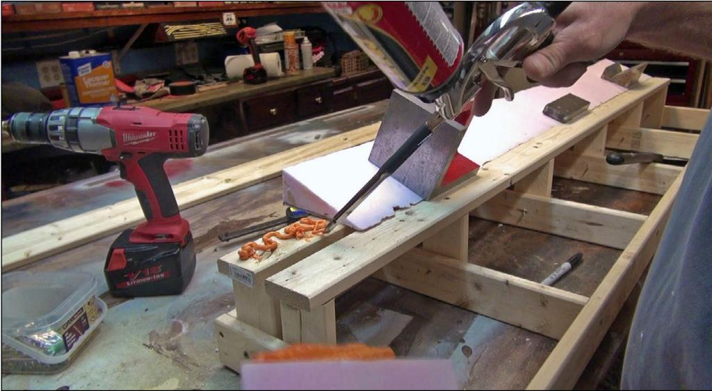
12. This month we experiment with Great Stuff Foam Pro, testing various subbases for holding the foam in place on open-grid benchwork. Here you see a 60 x 14 inch module with the track uprights in place and roadbed running the length of the scene. I glued precut pink foam to form the rear hill behind the track. The scenery on the hill in front of the module will be made up of various materials to hold the foam in place for our experiment.
