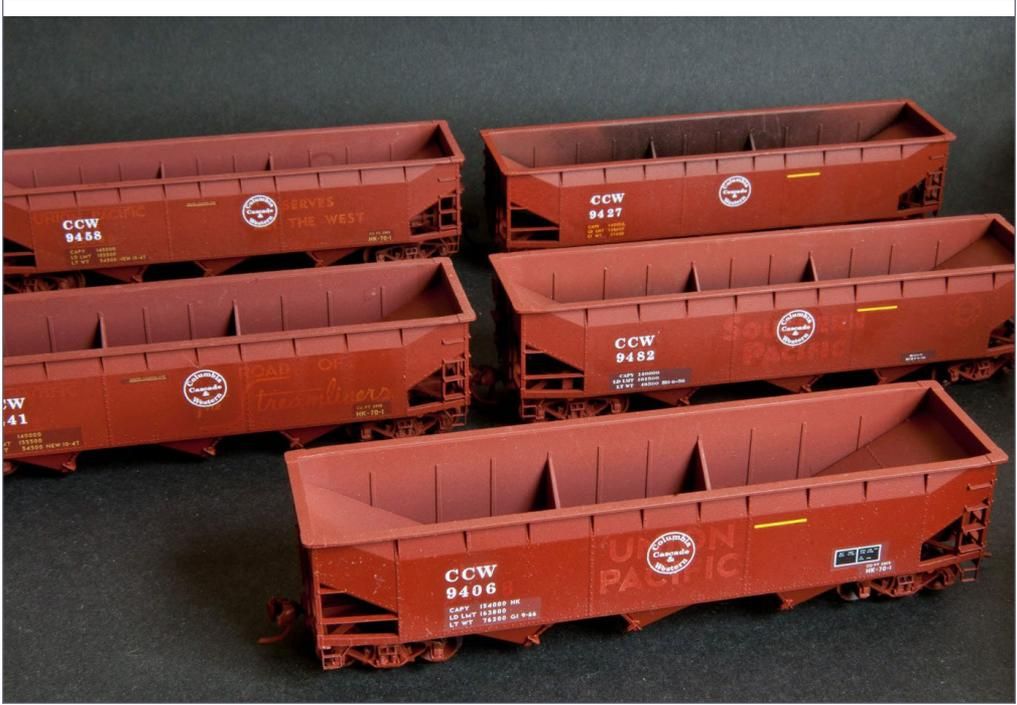
1. The CCW acquired its 26 rock cars on the secondhand market. Some cars got a light spray job with Krylon #1317 ruddy brown primer, and some are Southern Pacific freight car brown. The yellow lines indicate the maximum fill level for crushed rock and gravel. The models are Accurail 7500-series three-bay 70-ton offset hoppers, with Kadee #5 couplers and InterMountain 33-inch wheelsets.
