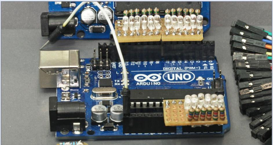
11. I wired all 18 LEDs shown here with 10k resistors, resulting in a total combined current draw for all the LEDs of less than 20ma – well below the Uno's 200ma board limit.
