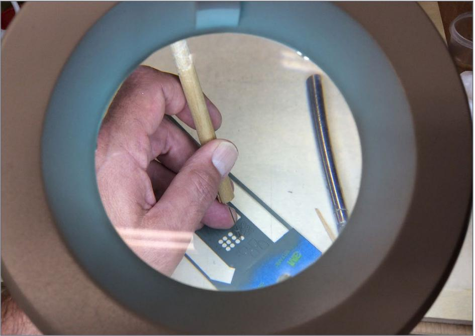
17. I use this tool a bunch – a needle glued into the end of a length of wooden round stock. The photo was taken looking through another essential tool, my illuminated magnifier.
