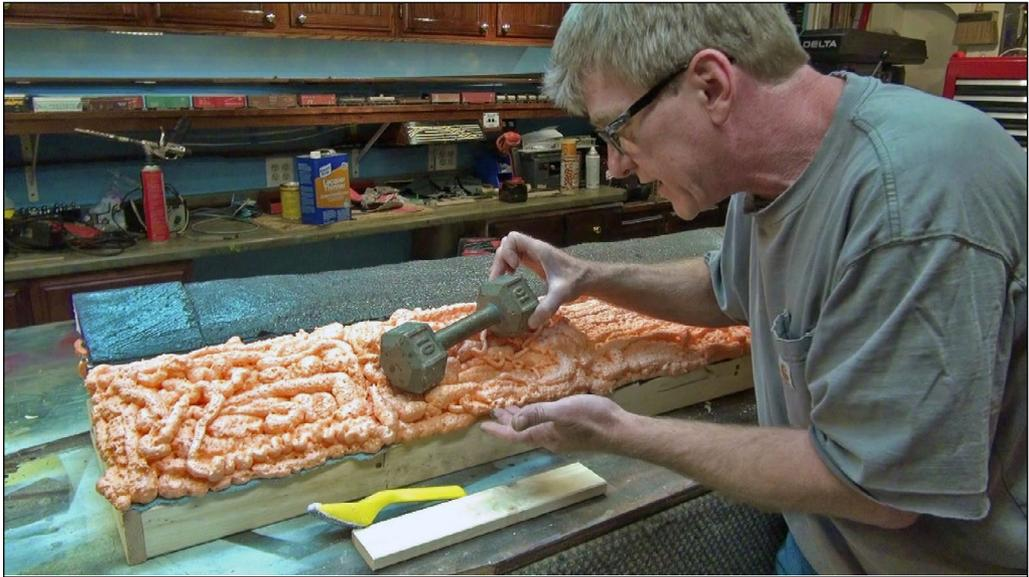
16. After the foam cured, I placed a 10-pound dumbbell to weight each section to see if it would hold up and could be used as a viable way to make scenery. All five sections held the weight without cracking.
