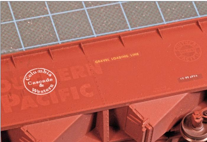
3. Rock is more dense than coal, so a smaller volume makes up a full load in a 70-ton car, and tops out several feet below the top chord. Cars assigned to aggregate loading are marked with a lettered notice or a 4-foot-long yellow line.
