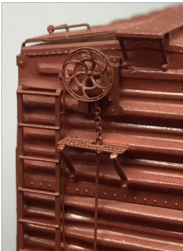
5. The B or brake end of a Sunshine SP B-50-28 box car, with Kadee Equipco hand brake.
