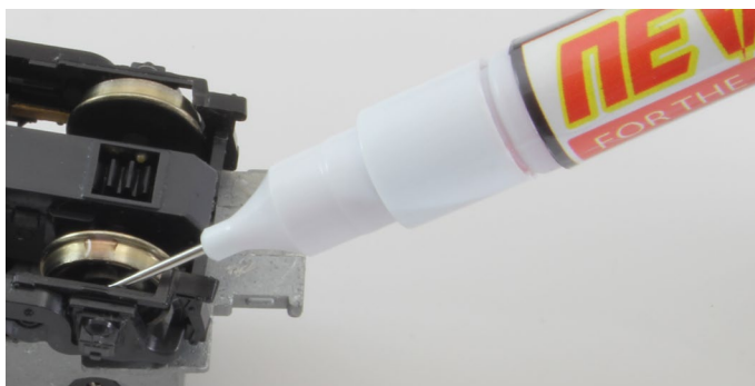
16. Applying Never-Still lubrication to the rolling contacts on the loco trucks.
