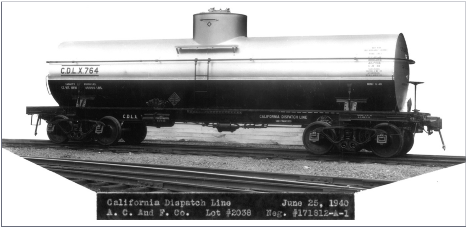
7. A California Dispatch Line insulated tank car, built for wine service, with National B-1 trucks. AC&F photo, courtesy Ed Kaminski
