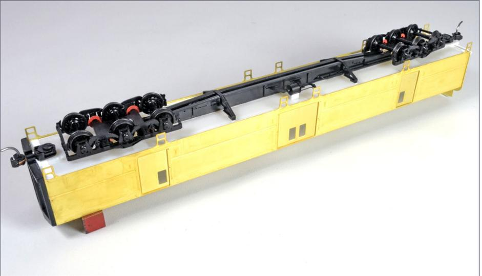
10. The center sill, air brake cylinder, trucks and couplers mount onto the carbody. Note that the brake cylinder points to the brass end.
