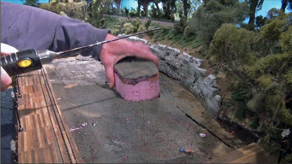
13. I used a hot foam cutter to cut a hole in the foam where the wires and light hubs will be installed. I also cut a hole in my plywood table top to match the area where the hole was cut in the foam.
