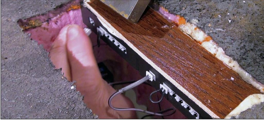
18. I plugged the other end of the connecting cables into each of the two light hubs. The hole in the foam provides plenty of room to squarely plug the jacks into the hubs along with great visibility to get the connectors in the correct hub plugs.
