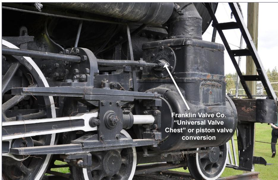
19. My prototype had an upgraded valve gear by Franklin Valve Co. I set about fabricating a new cylinder assembly to match this.
