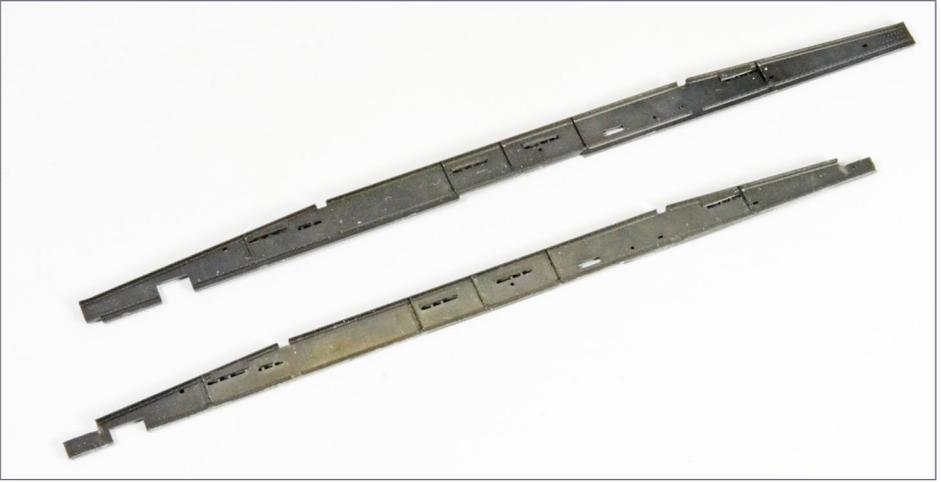
9. The center sill is modified by shortening and notching each end. In addition, the mounting tab is removed from each center sill's top.
