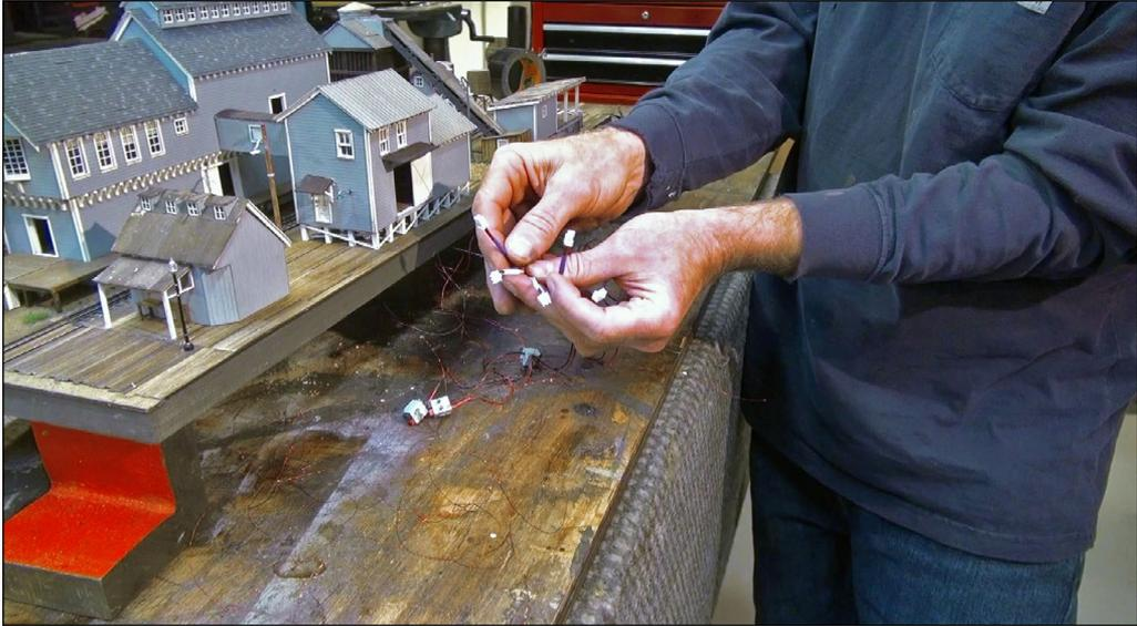
29. I twisted the light wires into groups of three as before and inserted the wires into the linker plugs until all the lights were wired. Be careful to match the polarity by color, red to red and black to black. This created a total of five sets of wires with plastic jacks on the ends which will be plugged into the light hubs installed in the foam module.
