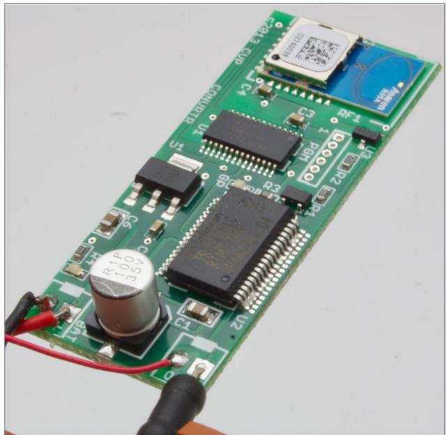
5. CVP CONVRTR-25 AirWire to DCC converter. The internal antenna is shown in the photo as the blue rectangle in the upper right. *Bruce Petrarca photo*
