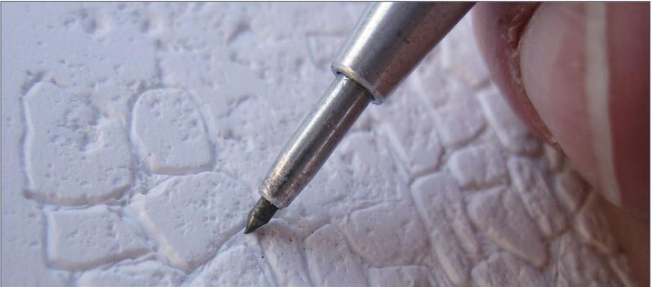
8. A standard steel scribe has many modeling uses. Here I'm using it to scribe the mortar lines on a stone wall.
