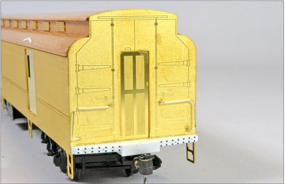
15. The brass end has fewer grabs, but Archer rivets, which shouldn't be added until immediately before painting.
