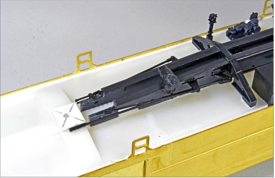
12. A closeup showing the brace beams, generator, and truck mounting plate.
