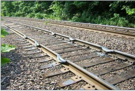
The lead engine stopped with brakes engaged and the remaining engine had to overcome not only the braked loco but trying to pull the entire load on its own. Once a slight railhead groove got established, the engine just spun in place and melted
