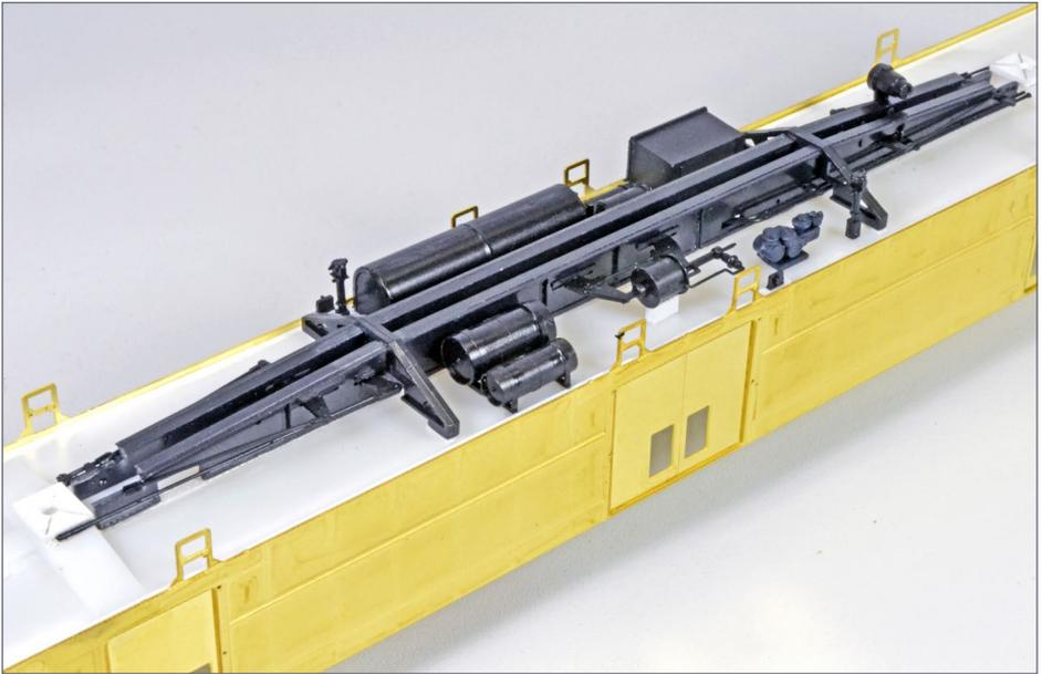
11. Underbody details are mounted to the underbody. After assembly, I discovered that the twin air tanks in the foreground should have been mounted closer to the brake cylinder, and a second battery box installed next to the cross brace, mirroring the battery box on the other side. C'est la vie!
