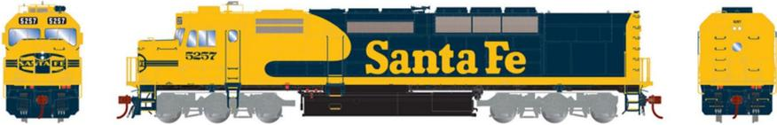
In 1984, Santa Fe traded some lower-powered locomotives to Amtrak for 18 SDP40F engines. They were reconditioned in ATSF's San Bernardino shops with new bolsters, the ballast and water supply were rearranged, and most importantly, they were regearred for freight service. Santa Fe christened them SDF40-2. Athearn's July release includes four Santa Fe road numbers.
