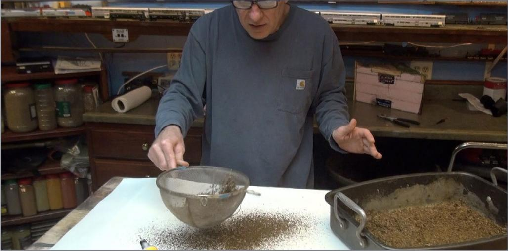
5. Bake for many hours at a temperature of 200 degrees, to end up with a pan of very dry leaf material. I use a colander with 1/32 of an inch openings in the screen. Sift the dry leaves through the screen onto a clean surface.
