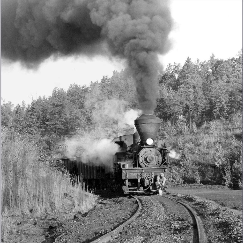
13. Shay No. 5 required extra sand to move just five loaded cars from the tipple over the 4% grade. The brakeman rode the pilot, pouring sand from a bucket to gain traction for the grade. *David Price Collection*
