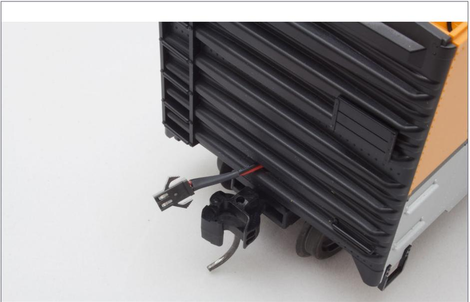
9. A-end of Piko battery car showing the male-pinned connector to mate with a loco. A bit of shrink tubing reduces the chafing on the wires when the connector is pushed back into the car after the loco connection has been made.
