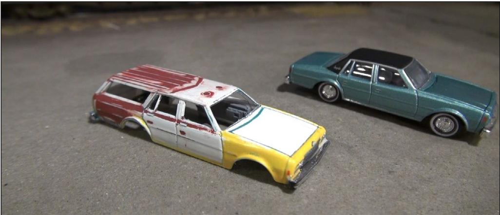
27. To make the station wagon, Mike cuts up a Mini Metals four-door Impala and adds styrene to form the body of the station wagon. He uses prototype photos as a guide. Mike then makes a rubber mold to cast 12 or so station wagons.
