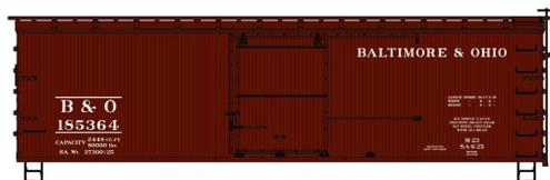
A 36-foot car with wood ends is available decorated for Baltimore & Ohio. It is based on a prototype built in 1925 and rebuilt in 1942.
