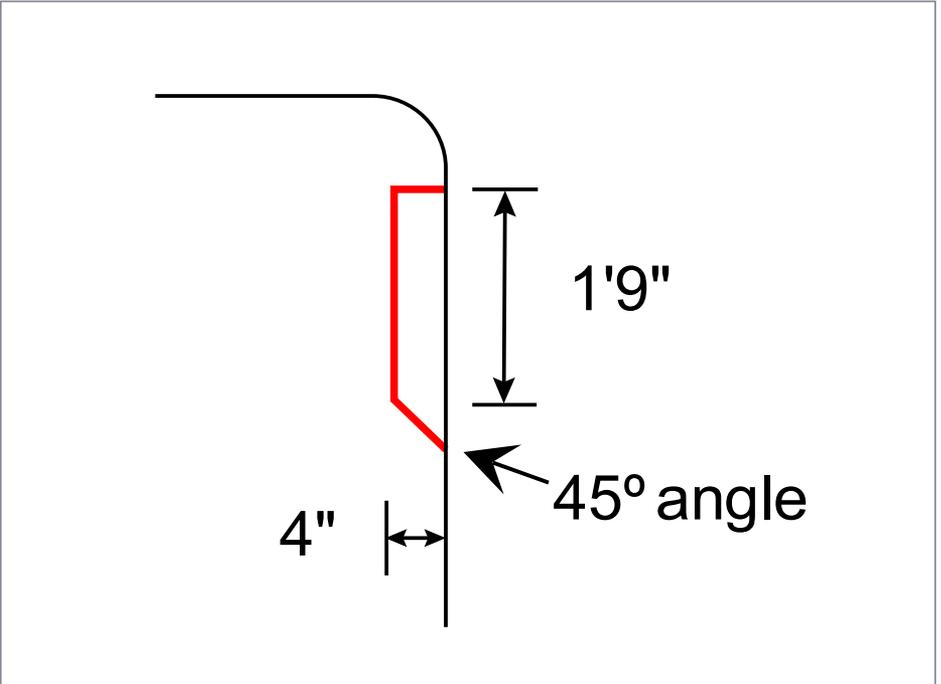
8. Dimensions of nose job (in scale measurements).
