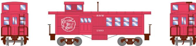
Completing the release of truss-rod era cars is a drover's caboose. The car has a side door for handling road supplies and LCL (less than car load) freight. It is equipped with clear window glazing and appropriate trucks with machined metal wheelsets. In addition to the Cotton Belt – St. Louis
