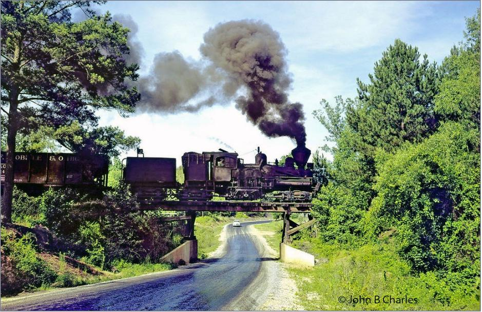
12. Shay No. 5 crossing the Kellerman “super” highway. This is the last trestle built for the extension to the new tippie. It is the only one with steel and concrete used in its construction. *Photo by John B. Charles, used with permission*
