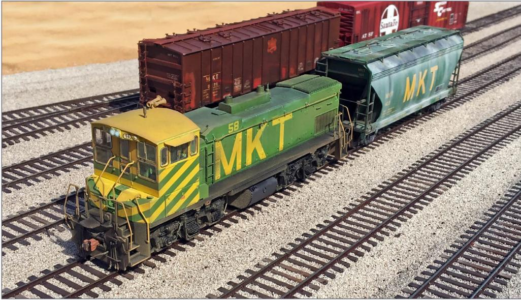
3. Scott Sanders modified a factory-painted Athearn Genesis MP15AC to match the MKT prototype engines. The big change needed was converting the Athearn MKT model from full-length handrails to the hand hold along the upper side of the locomotive found on Katy MP15ACs. Scott used .012" brass wire to simulate this distinctive feature. For weathering, Scott used oils and powders. He shot the photo on his yard diorama depicting the locomotive flat switching at the Katy's Eureka Yard in Houston, TX.
