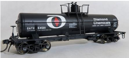
**Tangent Scale Models** has released new General American 8,000-gallon acid tank cars with welded underframes. Acid tank cars were rubber-lined, featured one percent expansion domes on
