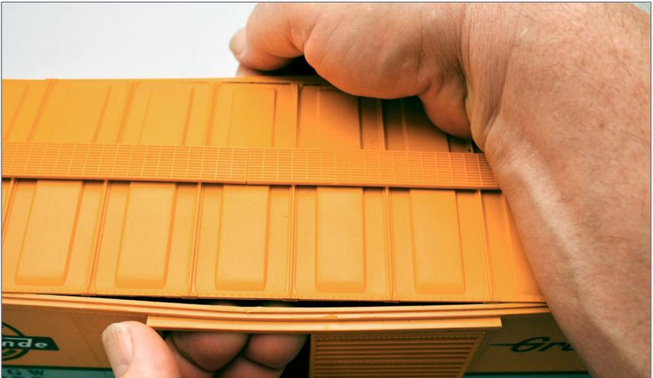
4. Removing the roof from the Piko box car. Open the doors, pull lightly out on the side wall just above each door. The tabs on the roof that engage the side walls should be able to be popped out, leaving the roof bowed from end to end. A slight tug on the end will release the end tabs. *Bruce Petrarca photo*
