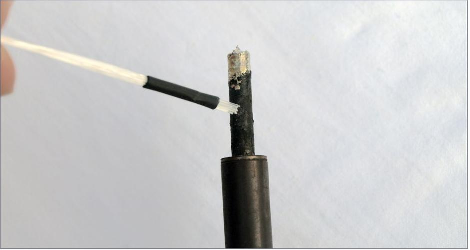
25. Using soldering iron to make light-gathering lenses.
