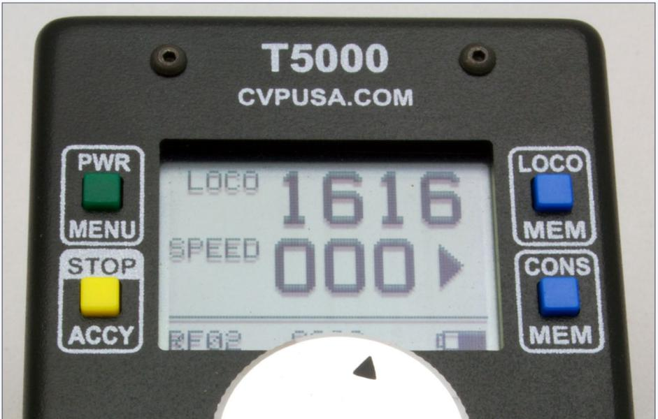
11. AirWire T5000 throttle on channel 02.
