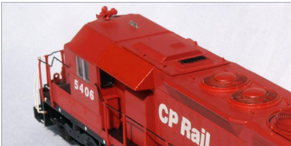
17. The completed awnings over the air intakes.
