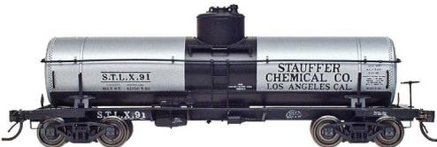
Completing the fall release will be a Stauffer Chemical car with a silver tank and a black waist band. The N scale ready-to-run model will be fitted with
