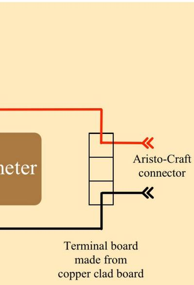
5. Schematic diagram for the battery car. I had no issues charging this battery with the digital meter connected. I used my X1 charger connected in place of the loco with the switch on. However, if your charger has issues connected this way, the charging connection shown (orange and gray wires in the diagram) could be added and used. If not needed, there is no reason for added confusion. *Bruce Petrarca diagram*
