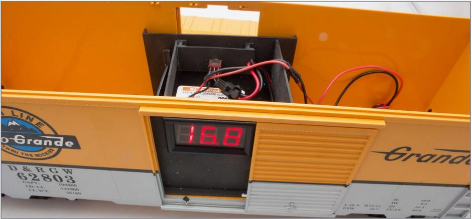
7. Side view of the Piko battery car showing the voltmeter. 16.8 volts indicates a fully charged battery. The batteries will hover between 15.25 and 14.75 volts for much of their life. Once they drop below 14 volts, it is time to turn off this battery car and charge it. *Bruce Petrarca photo*
