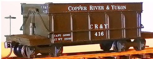
Precision Vintage Classics has introduced Sn3 and On30 kits for an ore car designed by Bryan Ellerby. The sides of the car are injection-molded plastic.
