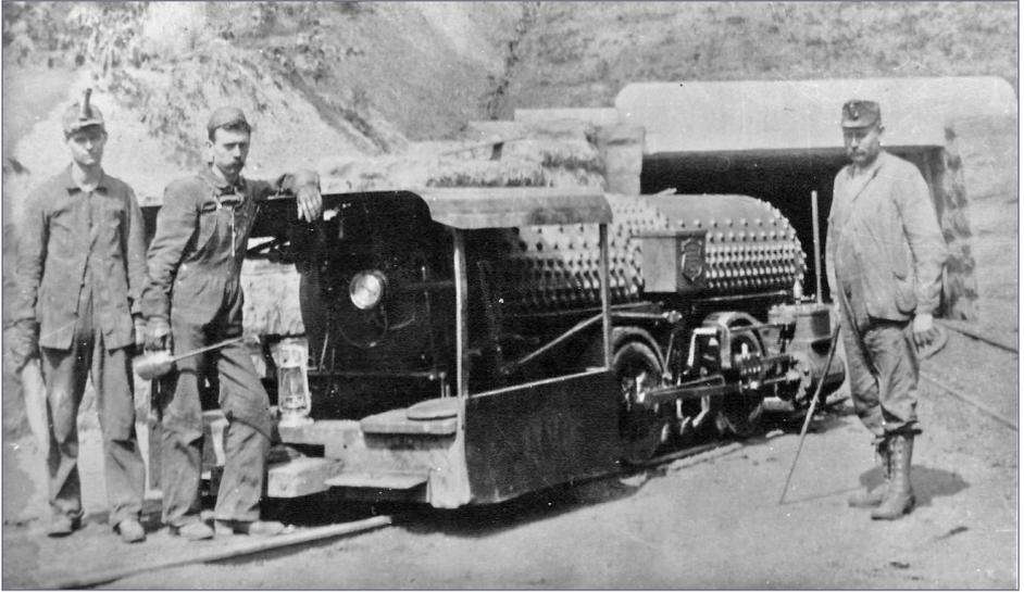
30. Compressed-air locomotive used by Twin Seam for underground operation. Central Coal and Iron 1903. Built by Porter April, 1903 C/N 2720.
