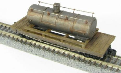
This narrow gauge tank car is available in kit form from **Showcase Miniatures**. Inspiration for the Nn3 model comes from a similar 24-foot prototype owned by the West Side Lumber Company. The kit includes a metal frame, laser-
