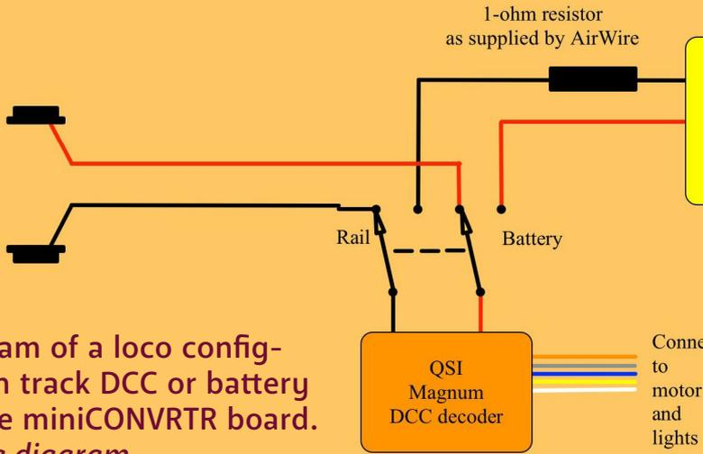
3. Block diagram of a loco configured to run on track DCC or battery and an AirWire miniCONVRTR board.
