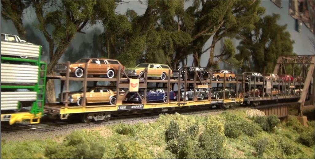
26. Here is a load of Mike's Chevrolet Impala station wagons and sedans. The glass in the windows is clear packing tape applied to the edges of the window frame from the outside.
