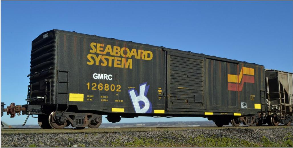
20. The last car is a Seaboard System boxcar with a wash of oils, underbody dust, and additional graffiti painted in place with a brush.
