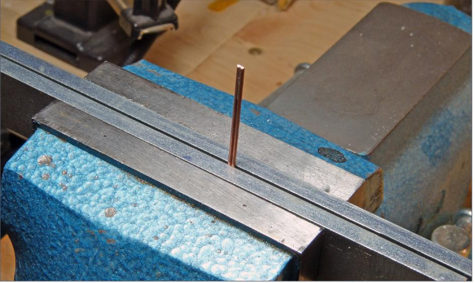
3. To form the fenders, flatten the ends of the barrier using a bench vise.
