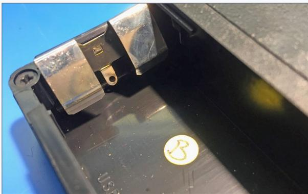
10. DT500 cabs have an on/off switch included, so they don't need their batteries flipped to shut them off. They have a different style of spring, making the insulation technique
