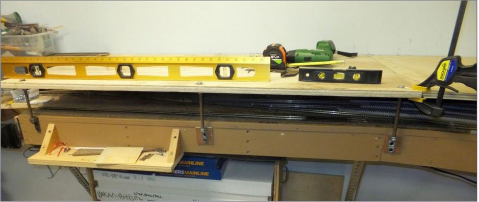
21. The temporary wood blocks have now been replaced by threaded rod. I recessed the nuts on top so they would not protrude above the cork. I'm using threaded pipe hangers as the bottom fastening point for the rod, since the new yard is slightly wider than the lower staging yard.
