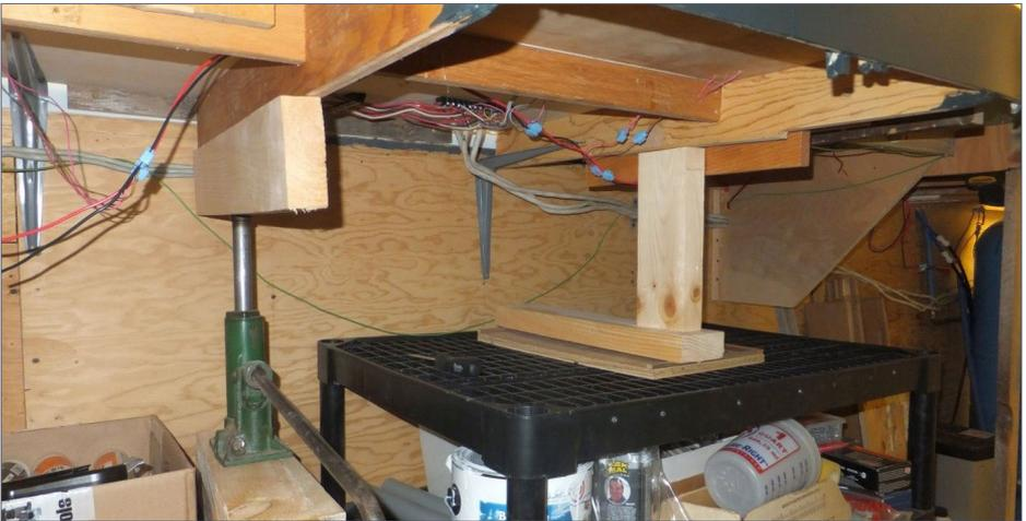
6. How do you raise a layout section by yourself? Why, with a hydraulic jack, of course! Once Ransom had been disconnected from the wall, it was simple to jack it to the correct height and reattach.
