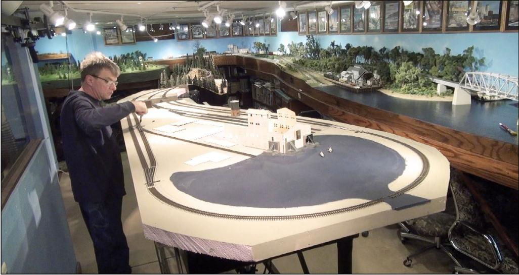
7. I start the process of building the B.T.S. sawmill complex by figuring the space required for all the buildings, and then place track around the scene with function, operation, and a minimum radius of 27 inches in mind. I draw lines with a black Sharpie where the tracks will be placed around the buildings and through the module.
