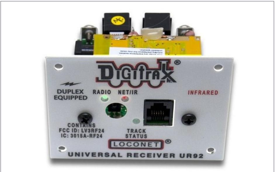
4. UR92 duplex radio base unit with infrared capability. The antenna is built into the (yellow) radio module.
