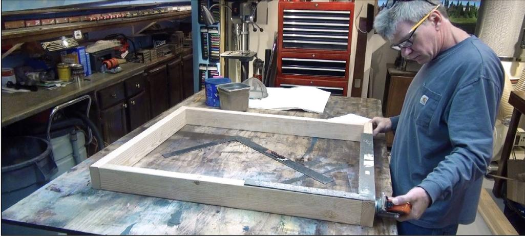
11. To hold the foam module I build benchwork from 2x4s, measuring from the floor to the top of the railhead. Every leg had to be cut to a different length as I was not going to use leg levelers on this project. Compensating for the uneven concrete floor ensures a level surface for the entire diorama.
