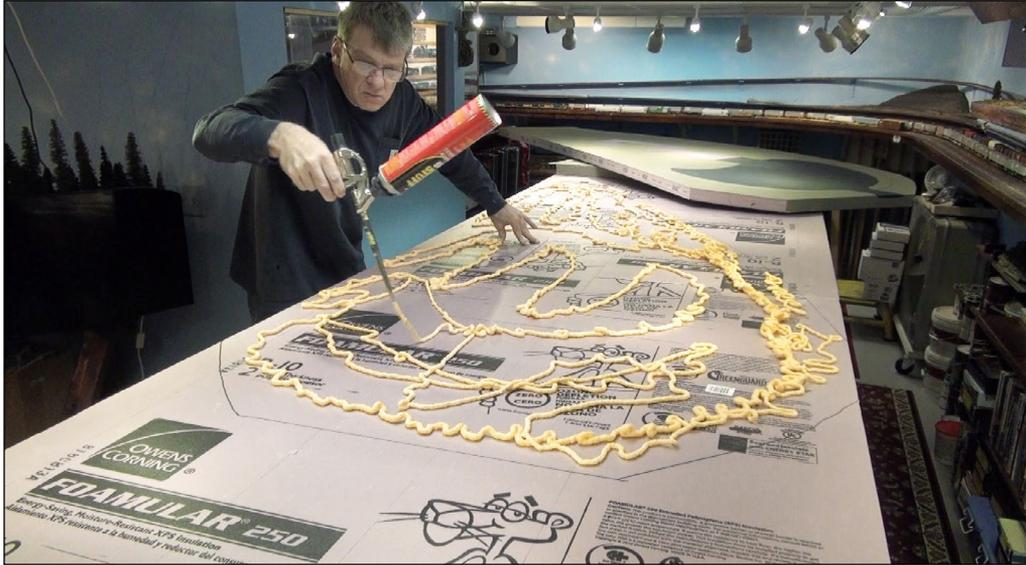
8. I then start stacking or layering two-inch-thick sheets of foam, gluing them together with Foam Pro Adhesive.
