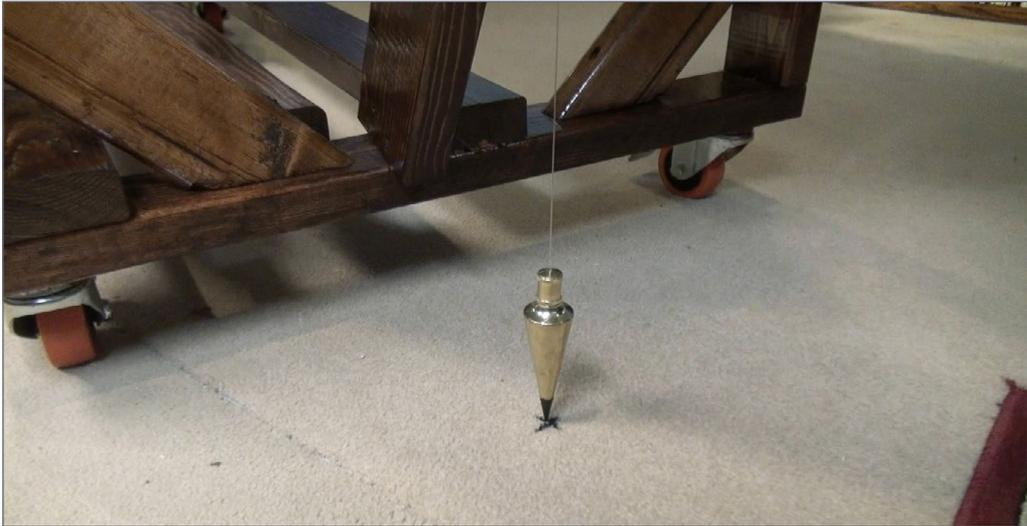
17. I also attach or hang brass plumb bobs to each end of the benchwork. These will point to an X on the floor when the benchwork is positioned in the room. This ensures the modules will be replaced in their exact location in the room after being moved for maintenance or photography. When the benchwork is back in its location, make sure each plumb bob points to its X. Then simply lock the wheels, slide the rail joiners on the track into position, and you're ready to run trains.
