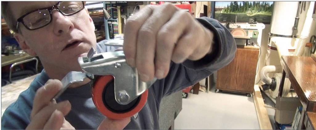
12. I attach these two-way locking wheels I found at Home Depot. It is very important to be able to both lock the wheel and to also lock the pivot. Locking this pivot point ensures the module won't wiggle from side to side, ensuring solid and tight benchwork.
