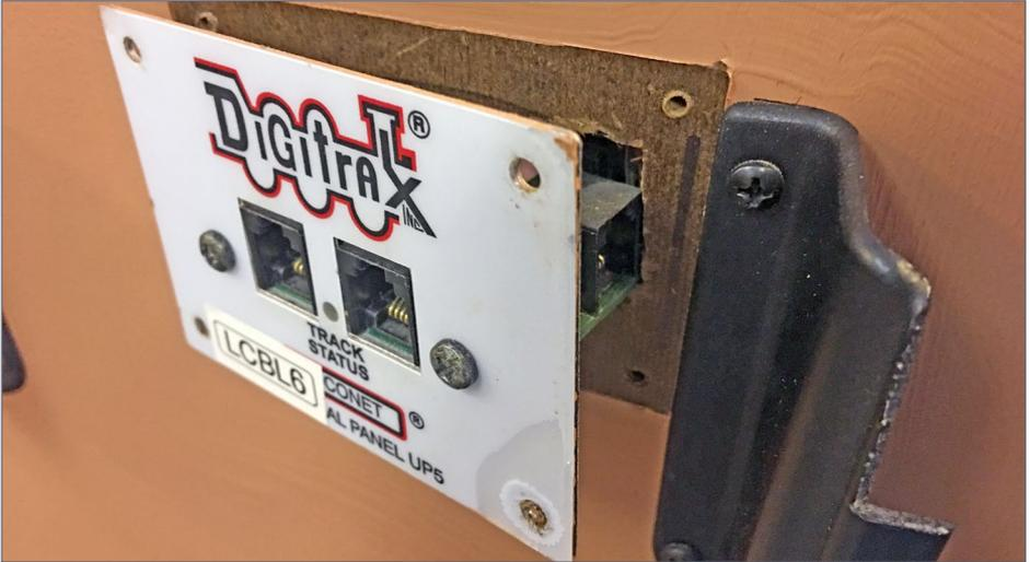
5. Mounting screws have been removed allowing the UP5 panel to slide out of the PCMRC layout.
