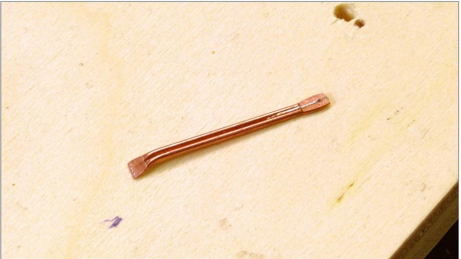
4. After flattening the ends, they need to be trimmed off and filed to make a smooth transition to the barrier.
