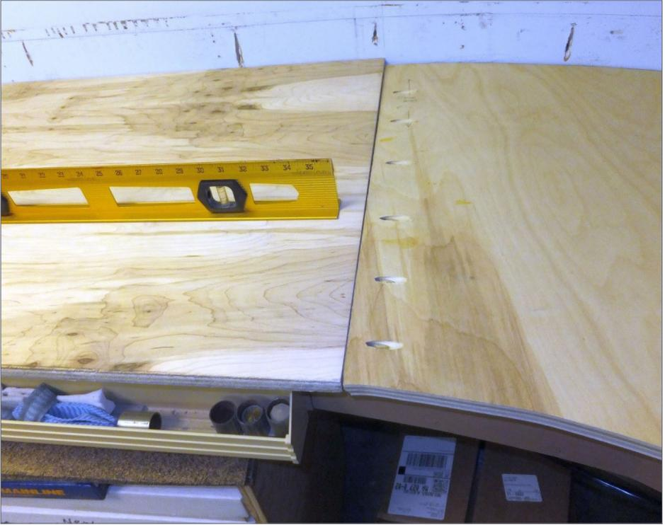
16. Since my clearances between the new Pittston Yard and the dropped staging yard were less than ideal, I decided not to use a conventional splice plate between the sub-roadbed sections and instead to use my new favorite tool: The Kreg Jig and pocket holes.
