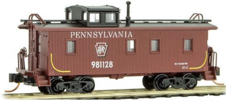
Modern Bettendorf-style swing-motion trucks have replaced the original arch bar trucks on this 34-foot wood sheathed caboose. The N scale model follows a prototype built in the
