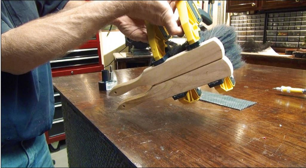
8. I sanded the clear coat off of each brush's wooden handle to ensure a good glue bond and allow me to stain the wood with red oak stain. Using carpenter's glue, I glue the handles together and clamp them tight. Let this cure overnight.
