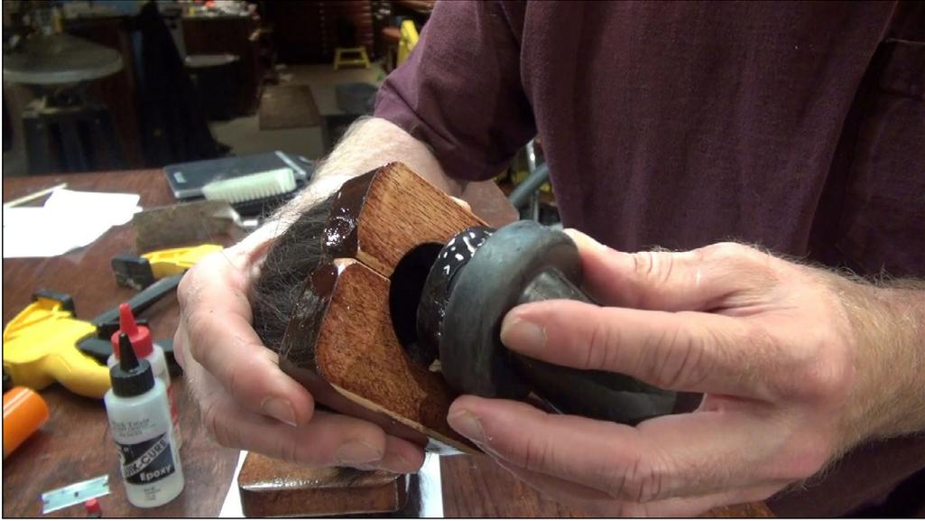
13. Mix some five-minute epoxy, apply this with a screwdriver around the round black edge of the attachment, and glue this into the wood for a perfect fit with both brushes. Set the part aside to cure.
