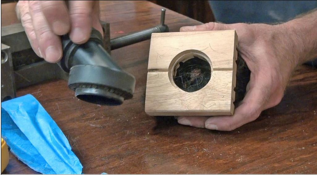
10. After cutting off the brush handles, I start making a vacuum attachment by cutting the synthetic fibers off of a two-inch round brush. Once the fibers are cut off, match the diameter of a Forstner wood hole cutting bit to match of the diameter of the vacuum cleaner attachment. Drill this hole through the fibers, wood, and nails holding the fiber hair in place in the brush. Then, test-fit the black brush attachment into the hole. Everything should fit together perfectly.
