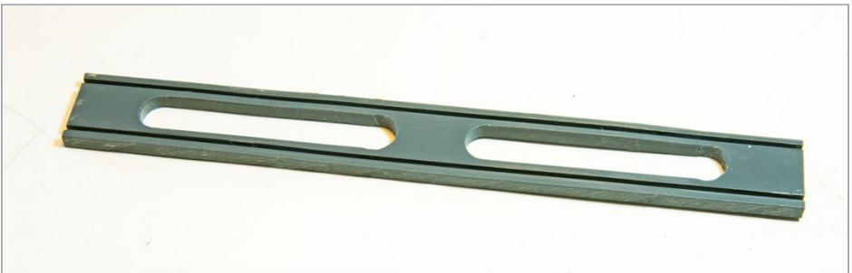
4. MLR Engineering produced this 8" resin tool for aligning flex track. It's also useful for cutting rail ends to match. Hardwood or aluminum could be used to make a similar tool. *MRH photo*
