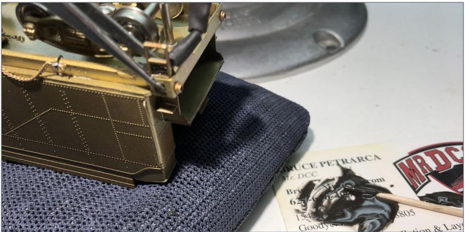
8. Applying JB Kwik Weld to hold heat-shrink tubing in place on a loco tender. *Bruce Petrarca photo*
