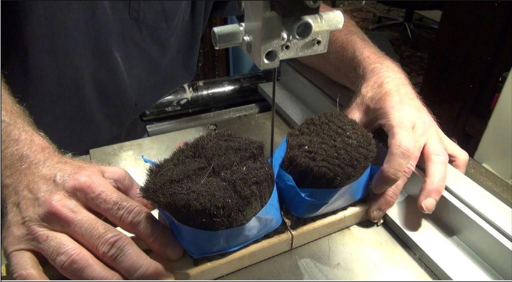
9. Using a trowel, I divide the brush fibers into two sections and wrap this in tape to keep things divided as I run the brush through the bandsaw. Cut it in half, making two brushes each measuring about 3 ½ inches square.
