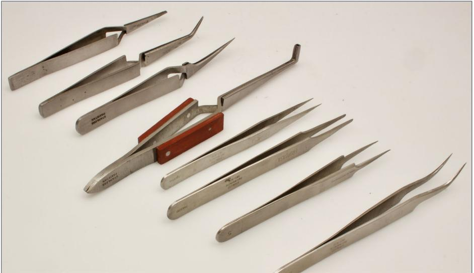
10. I use a bunch of tweezers, both regular and clamping styles. I prefer non-magnetic stainless steel whenever I can get it – most of the clamping ones are magnetic, alas. My favorite is the curved version in front. *Bruce Petrarca photo*
