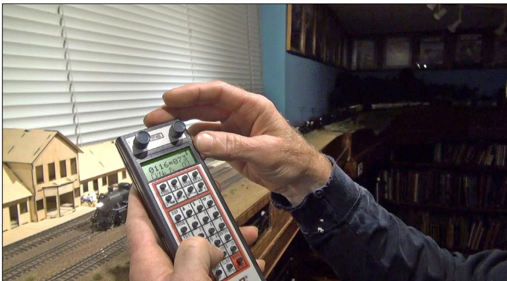
24. In the video, we take the model inside and set up the sound decoder's DCC quartering of the drivers and the delay or momentum to enhance the performance of the model. To match sound to the quartering of the drive wheels, we use CV 116. Through trial and error, I eventually found that programming CV 116 to 73 synchronized the wheels perfectly with four chuffs per revolution of the main driving wheels.
