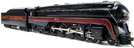
service, was perhaps the pinnacle of Norfolk & Western's steam development, featuring lightweight connecting rods, streamlining, and roller bearings
