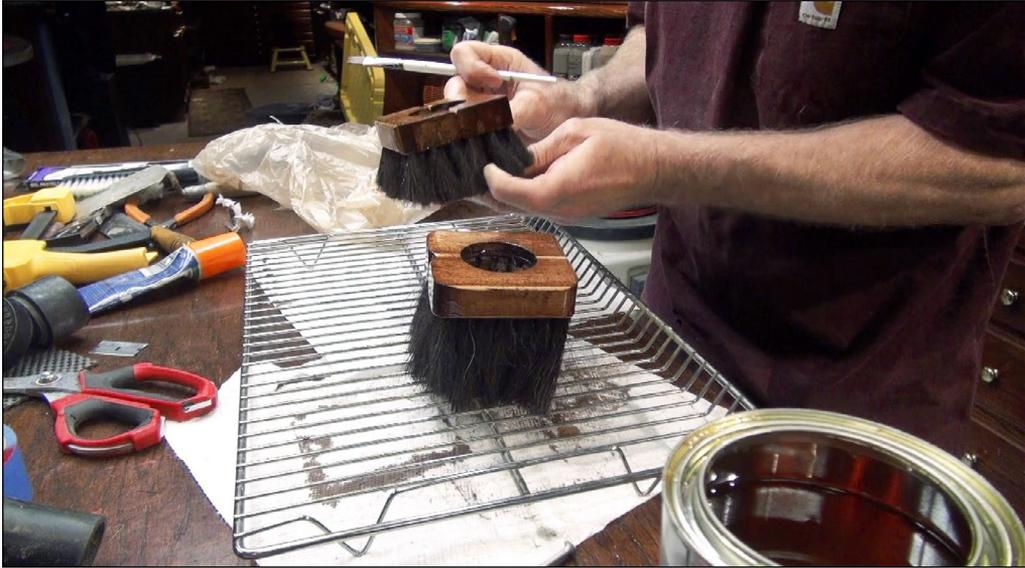
12. Repeat the process on the second brush, and with that we have two brushes to work with for this experiment. I cut the fiber hairs on one of the brushes with scissors but discovered later that a barber's hair clipper/trimmer works much better than scissors for cutting the fibers smooth and even. Cut the brush so the remaining fibers measure 1½ inches long. Stain and polyurethane the wood without getting any of the finish on the brush hairs.
