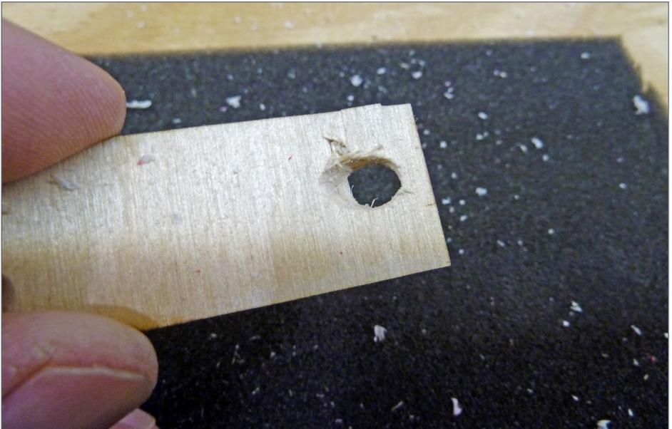
12. Sloped drilling jig made from 1/8" plywood.
