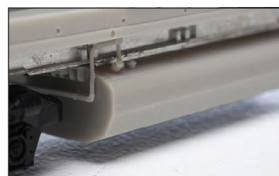
NS specific crash-worthy fuel tank per prototype
