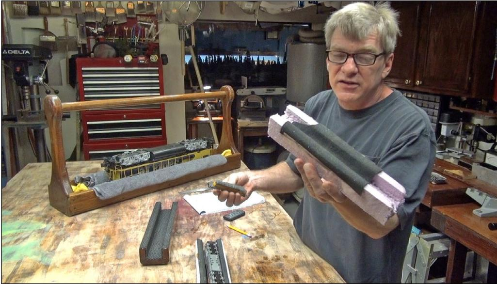
5. A locomotive cradle is an essential tool to hold models safely when doing repairs, decoder installations, or simple coupler replacement. I have three examples in this photograph. The large-scale cradle is lined with a bath towel. An N scale cradle is made from a piece of foam carved out and lined with felt, and the HO scale cradle we will build for this article.
