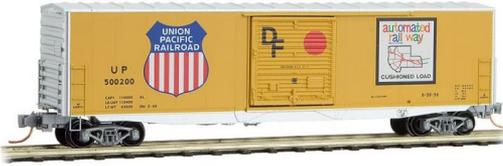
scale model include short ladders, no running board, and an extended cushion underframe.
