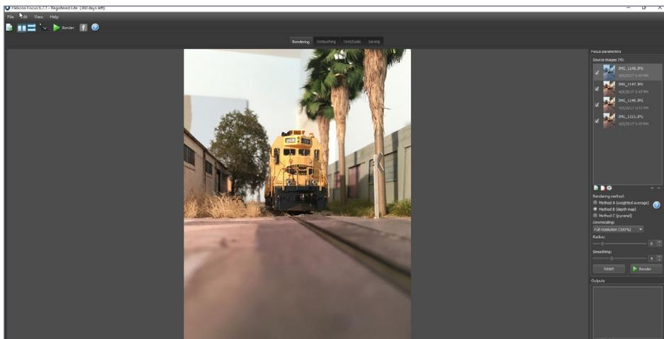
6. This is the work screen of the Helicon Focus program. It's very simple to use. Open a shot, drag it to the right source panel box, repeat for each image, and then hit "Render." Make sure to save your work.
