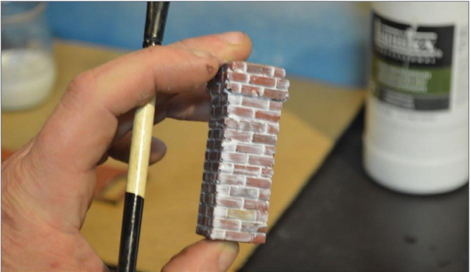
9. Apply the water/matte medium to wash the full strength layer from the brick faces, and let it dry. Check to see if you are happy with the finish. If not, add a second coat of medium and wash. I got this final finish with two coats.
