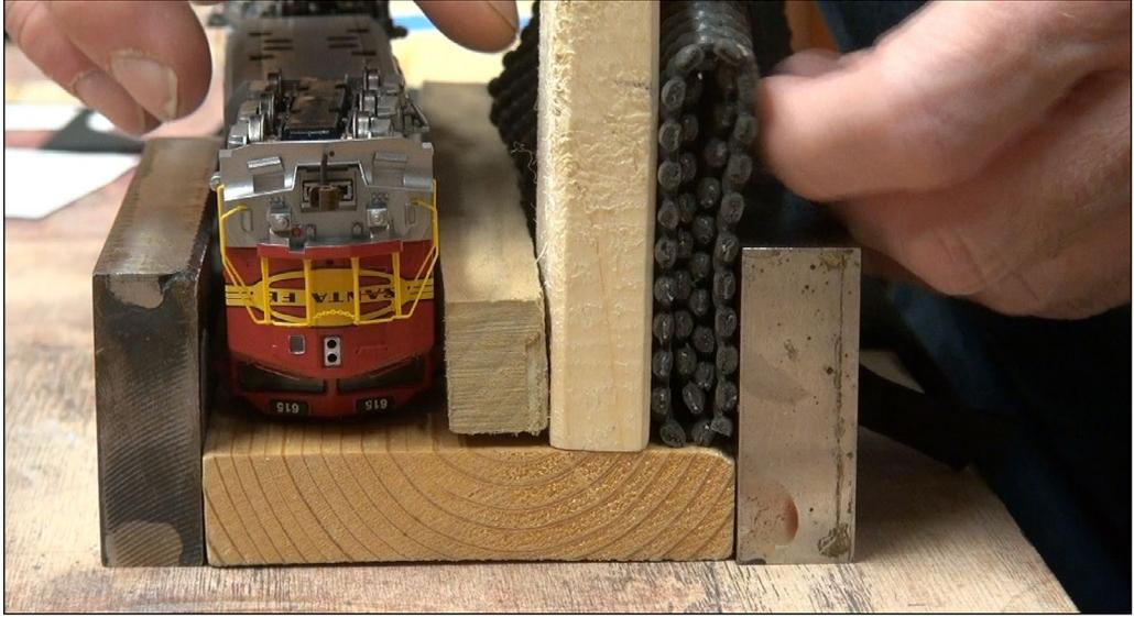
6. Using a scrap 1x4 for the base, I measured the width of a locomotive with sunshades. Then I figured the dimensions for the cradle's walls along with the thickness of the drawer liner made from synthetic rubber. In HO scale the clearance side to side needed to be  $1\frac{3}{4}$  inch to clear the locomotive sunshades.
