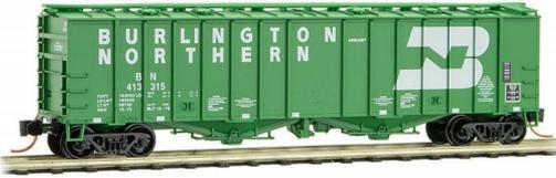
This Burlington Northern 50-foot Airslide covered hopper car features well-detailed outlet fixtures and underframe, and 100-ton
