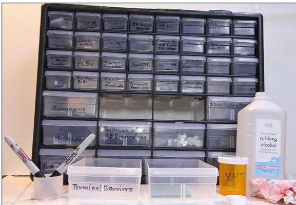
Labeling on plastic parts cabinets drawers with “permanent” labels like a black Industrial Sharpie, regular Sharpie, or general type marker can usually be wiped off with isopropyl (rubbing alcohol) and the drawer relabeled. The same trick works well on pill bottles.
