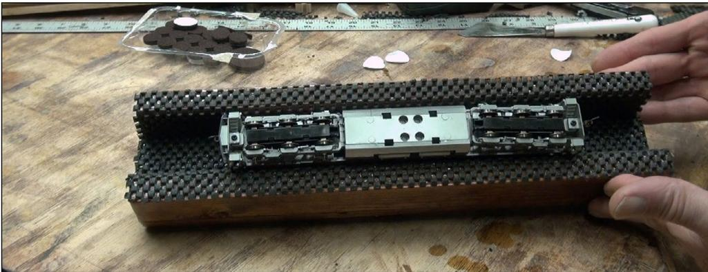
11. After the silicone glue dried I applied soft self-stick felt pads to the bottom of the cradle as feet. And with that, we have a new tool for gently holding models in place during repairs or while painting trucks, wheels, or underbody details.
