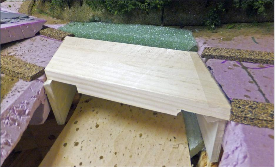
24. (Above) After determining the bridge location and gluing the abutments at the correct height, I made a blank out of wood to act as a place-holder for the bridge itself. This would allow me to “pave” right up to the blank, let the road material cure, remove the blank, and then simply drop the Pikestuff bridge into place, and have everything line up. I wanted the bridge removable so that I could do the stream bed and water pour without it being in the way.
