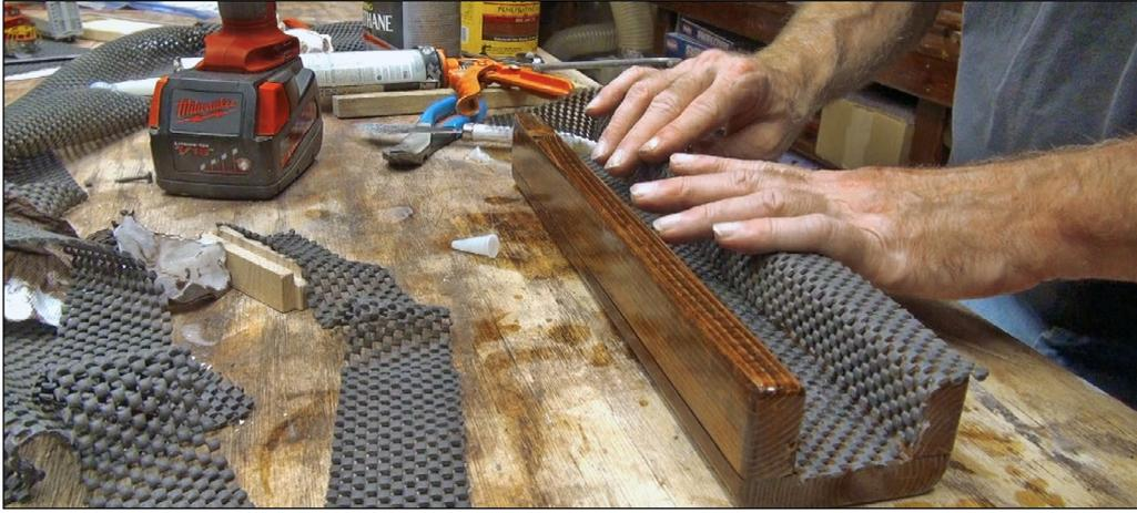
10. I used a box knife and a straight edge to cut strips of drawer liner material to fit in the cradle, providing a soft cushioned surface to the wood. I spread clear silicone adhesive to the inside walls of the cradle using a Ross painters knife. Then I pressed the black drawer liner into the silicone glue, wrapping the black material around the top sides of the cradle as seen in this photo.
