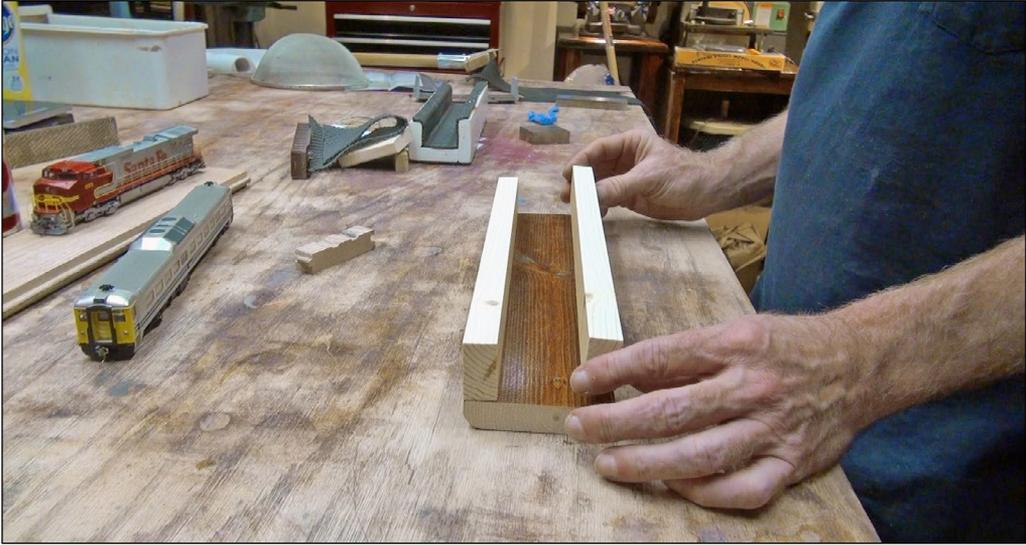
8. I made the side walls about 1½ inches high, then proceeded to cut the base on a radial arm cutoff saw. The sidewalls were run through the band saw. After test-fitting the pieces together to form our cradle, I used wood screws to assemble the new locomotive cradle.
