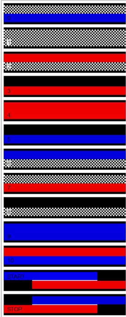
Even in the early years of the program there were problems reading the panels after dirt and grime accumulated in service. After several years, a test made under ideal conditions still showed a 10% mis-read rate, and the industry pulled the plug on the program.
