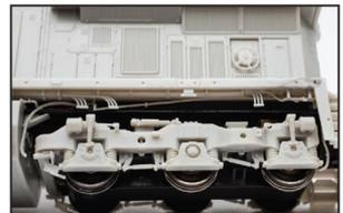
Separately-applied plumbing and traction motor cables.
