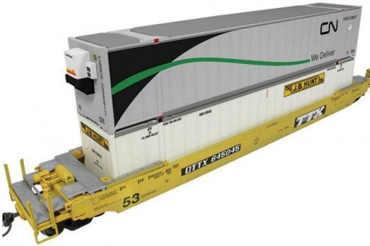
features a die-cast body with injection-molded plastic running boards, end handrails and extensive brake detail. The trucks are a new 70-ton design with separate in-line brake shoes, visible springs, and 33-inch metal wheelsets.
