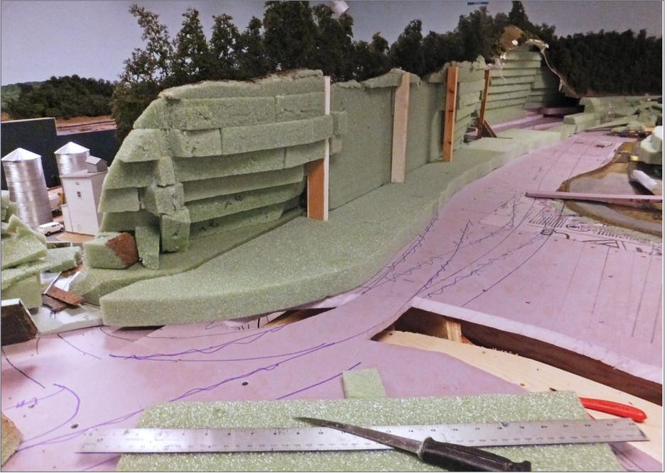
8. With the base layer cut out and in place, I had my starting point to proceed up the mountain face rapidly. One of the things I love about this type of construction is how easy it is to cut the foam using the pictured tools (that's a fish file knife that I sharpen often during this process).
