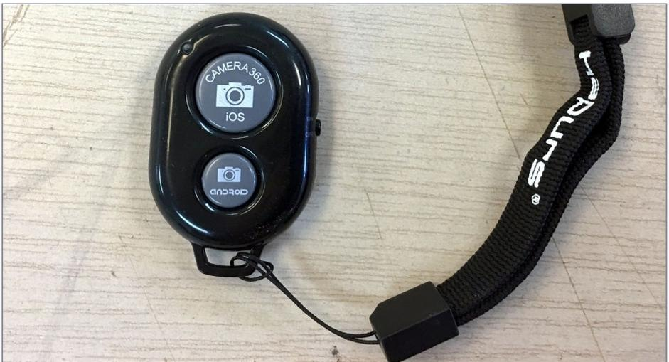
8. Remote shutter releases, such as the one above, are inexpensive and allow you to take shots without touching the camera. They are set up through the phone's Bluetooth settings.
