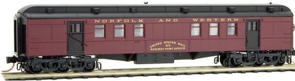
Also new is a Norfolk & Western Railway Post Office car. Both of these heavyweight steel head-end cars ride on six-wheel passenger trucks.
